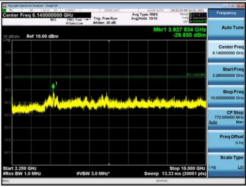
Antenna 0 / 10 GHz ~ 26.5 GHz / B25 LTE 5 MHz 1 Carrier + B25 LTE 20 MHz 1 Carrier + B25 LTE 5 MHz 1 Carrier + B66 LTE 10 MHz 1 Carrier [4 Carrier]\_Low / 64QAM
