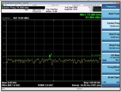
Antenna 0 / 150 kHz ~ 30 MHz / B25 LTE 5 MHz 1 Carrier + B25 LTE 20 MHz 1 Carrier + B25 LTE 5 MHz 1 Carrier + B66 LTE 5 MHz 1 Carrier + B66 LTE 10 MHz 1 Carrier [5 Carrier] / 16QAM
