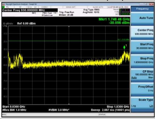
Antenna 1 / Low Edge - 100 MHz ~ Low Edge / B25 LTE 5 MHz 1 Carrier + B25 LTE 20 MHz 1 Carrier + B25 LTE 5 MHz 1 Carrier + B66 LTE 5 MHz 1 Carrier + B66 LTE 20 MHz 1 Carrier [5 Carrier] / QPSK
