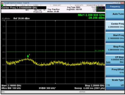
Antenna 1 / High Edge ~ High Edge + 100 MHz / B25 LTE 5 MHz 1 Carrier + B25 LTE 20 MHz 1 Carrier + B25 LTE 5 MHz 1 Carrier + B66 LTE 10 MHz 1 Carrier + B66 LTE 10 MHz 1 Carrier | 16QAM
