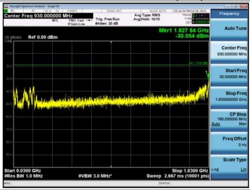
Antenna 1 / Low Edge - 100 MHz ~ Low Edge / B25 LTE 5 MHz 1 Carrier + B25 LTE 20 MHz 1 Carrier + B25 LTE 20 MHz 1 Carrier + B66 LTE 10 MHz 1 Carrier + B66 LTE 10 MHz 1 Carrier | 16QAM
