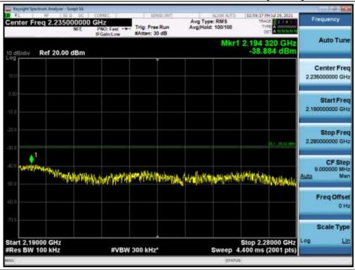
Antenna 3 / High Edge ~ High Edge + 100 MHz / B25 LTE 5 MHz 1 Carrier + B25 LTE 20 MHz 1 Carrier + B25 LTE 20 MHz 1 Carrier + B66 LTE 10 MHz 1 Carrier + B66 LTE 10 MHz 1 Carrier | 64QAM
