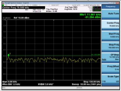
Antenna 0 / 150 kHz ~ 30 MHz / B25 LTE 5 MHz 1 Carrier + B25 LTE 20 MHz 1 Carrier + B25 LTE 5 MHz 1 Carrier + B66 LTE 5 MHz 1 Carrier + B66 LTE 20 MHz 1 Carrier [5 Carrier] / 256QAM
