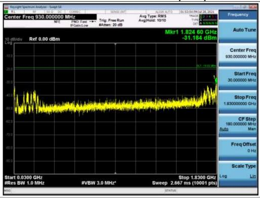
Antenna 1 / Low Edge - 100 MHz ~ Low Edge / B25 LTE 5 MHz 1 Carrier + B25 LTE 20 MHz 1 Carrier + B25 LTE 5 MHz 1 Carrier + B66 LTE 5 MHz 1 Carrier + B66 LTE 10 MHz 1 Carrier [5 Carrier] / QPSK
