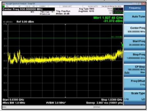
Antenna 1 / Low Edge - 100 MHz ~ Low Edge / B25 LTE 5 MHz 1 Carrier + B25 LTE 20 MHz 1 Carrier + B25 LTE 20 MHz 1 Carrier + B66 LTE 5 MHz 1 Carrier + B66 LTE 10 MHz 1 Carrier [5 Carrier] / 16QAM
