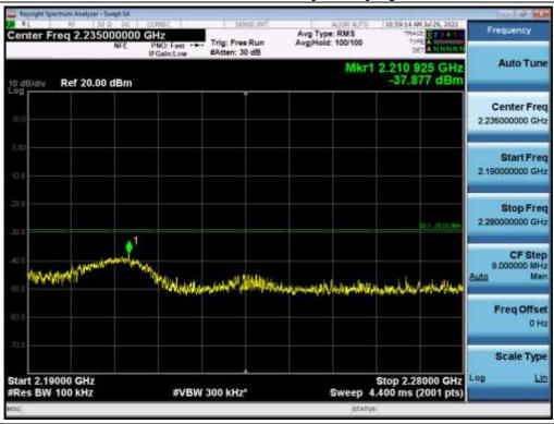
Antenna 1 / High Edge ~ High Edge + 100 MHz / B25 LTE 5 MHz 1 Carrier + B25 LTE 20 MHz 1 Carrier + B25 LTE 5 MHz 1 Carrier + B66 LTE 10 MHz 1 Carrier [4 Carrier]\_High / 64QAM
