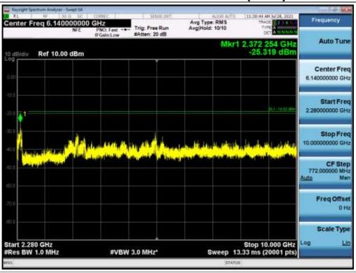
Antenna 1 / 10 GHz ~ 26.5 GHz / B25 LTE 5 MHz 1 Carrier + B25 LTE 20 MHz 1 Carrier + B25 LTE 5 MHz 1 Carrier + B66 LTE 5 MHz 1 Carrier + B66 LTE 20 MHz 1 Carrier [5 Carrier] / 256QAM
