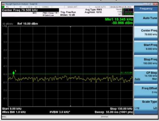
Antenna 0 / 150 kHz ~ 30 MHz / B25 LTE 5 MHz 1 Carrier + B25 LTE 20 MHz 1 Carrier + B25 LTE 5 MHz 1 Carrier + B66 LTE 10 MHz 1 Carrier | 5 Carrier | 7 16QAM
