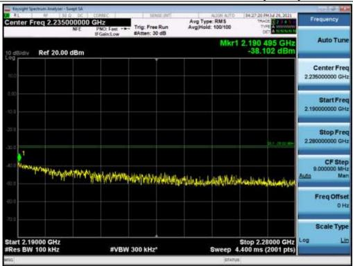
Antenna 2 / High Edge ~ High Edge + 100 MHz / B25 LTE 5 MHz 1 Carrier + B25 LTE 20 MHz 1 Carrier + B66 LTE 5 MHz 1 Carrier + B66 LTE 10 MHz 1 Carrier [5 Carrier] / 256QAM
