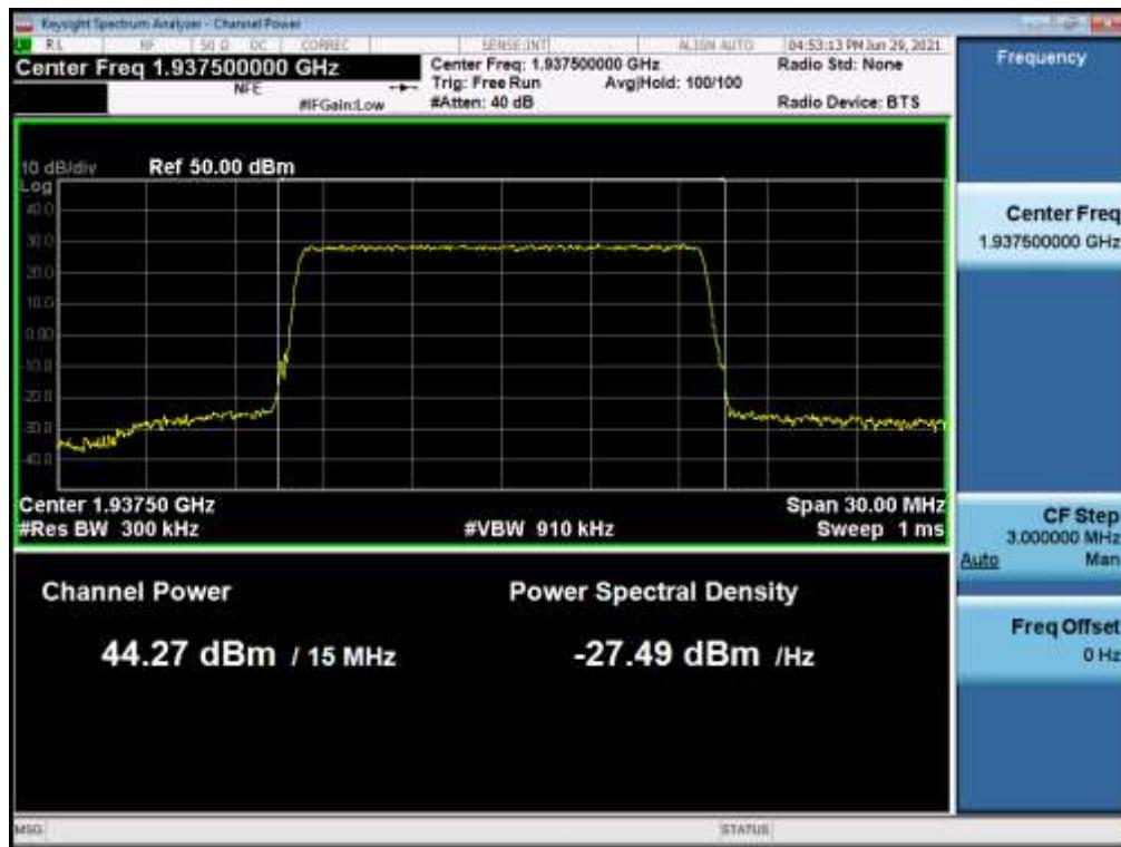
**Antenna 1 / B25 LTE 15 MHz 1 Carrier + B25 LTE 20 MHz 1 Carrier [2 Carrier] / Non-Contiguous / B25 LTE 20 MHz / 64QAM / High**
