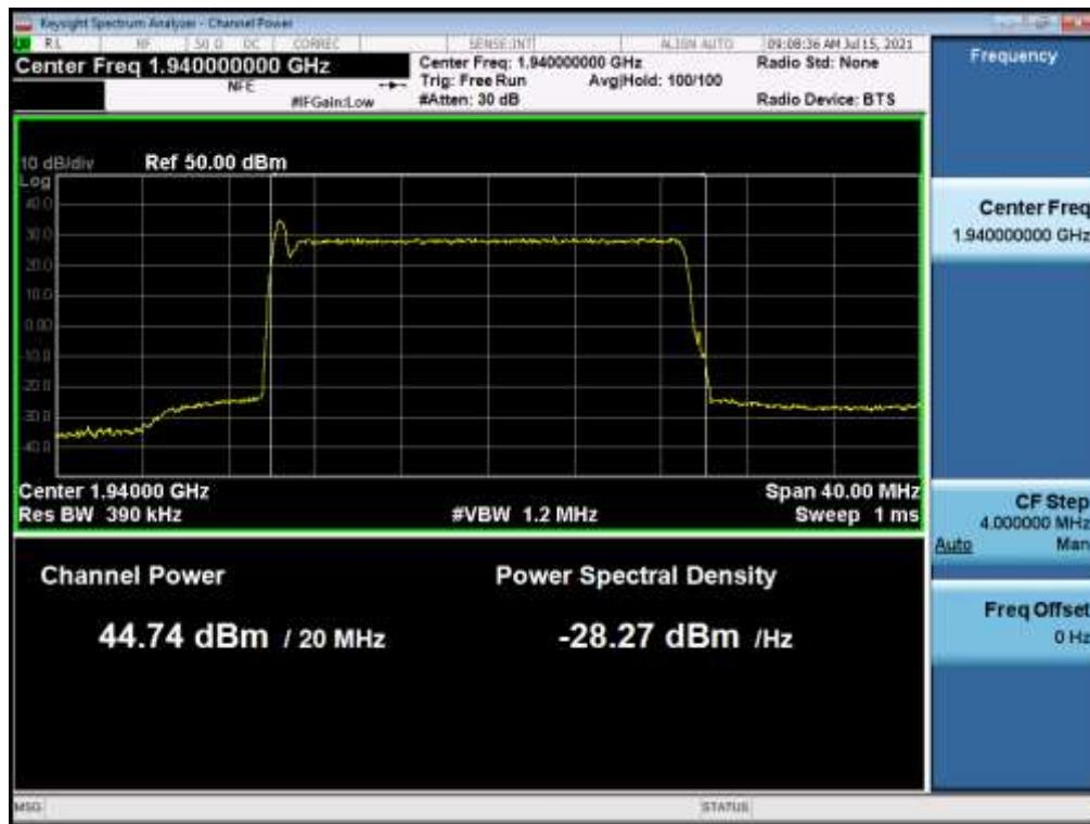
**Antenna 1 / B25 LTE 20 MHz & NB-IoT 1 Carrier + B25 LTE 20 MHz 1 Carrier [2 Carrier] / Non-Contiguous / B25 LTE 20 MHz / QPSK / High**
