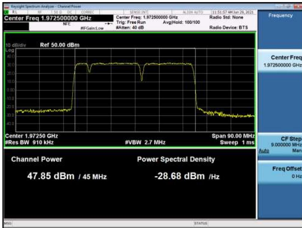
**Antenna 1 / B25 LTE 5 MHz 1 Carrier + B25 LTE 20 MHz 1 Carrier + B25 LTE 20 MHz & NB-IoT 1 Carrier [3 Carrier] / Contiguous / 16QAM / Middle**
