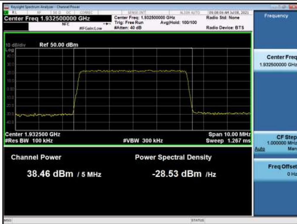
**Antenna 1 / B25 LTE 5 MHz 1 Carrier + B25 LTE 20 MHz 1 Carrier + B25 LTE 20 MHz 1 Carrier [3 Carrier] (1C+2C) / Non-Contiguous / B25 LTE 20 MHz + B25 LTE 20 MHz / 256QAM / High**
