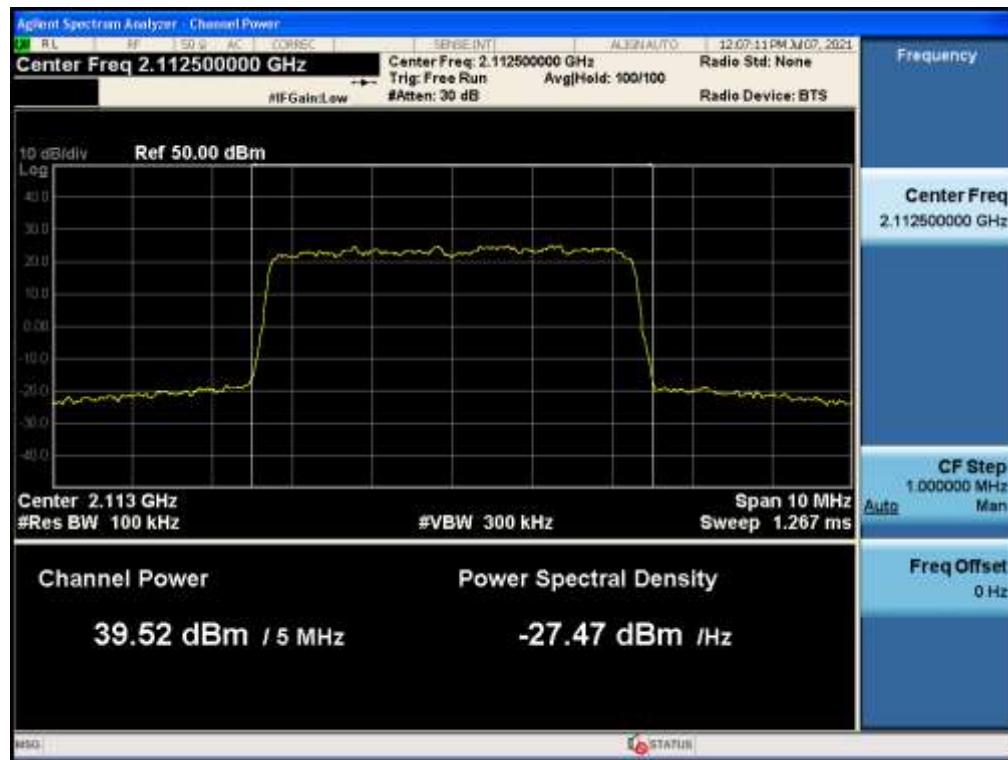
**Antenna 1 / B66 LTE 5 MHz 1 Carrier + B66 LTE 10 MHz & NB-IoT 1 Carrier [2 Carrier] / Non-Contiguous / 16QAM / B66 LTE 10 MHz & NB-IoT / High**
