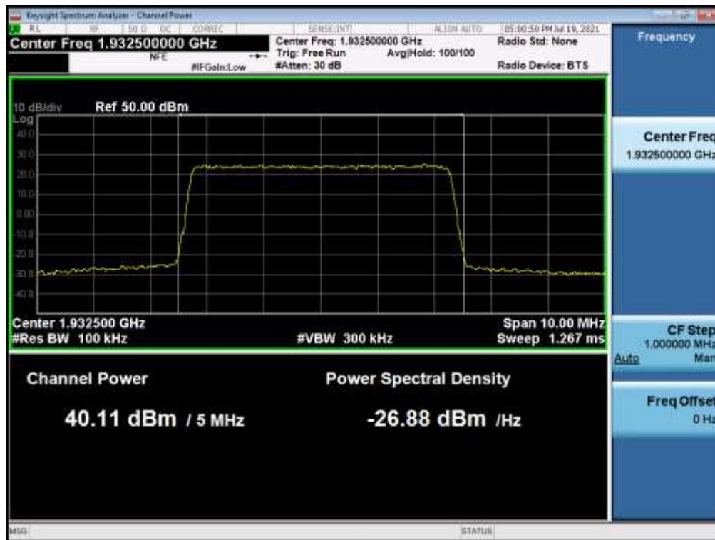
**Antenna 0 / B25 LTE 5 MHz 1 Carrier + B25 LTE 5 MHz 1 Carrier + B25 LTE 20 MHz & NB-IoT 1 Carrier [3 Carrier] (1C+2C) / Non-Contiguous / B25 LTE 5 MHz + B25 LTE 20 MHz & NB-IoT / 256QAM / High**
