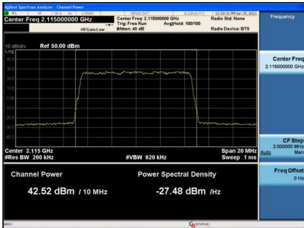
**Antenna 3 / B66 LTE 10 MHz 1 Carrier + B66 LTE 10 MHz 1 Carrier [2 Carrier] / Non-Contiguous / B66 LTE 10 MHz / 16QAM / High**
