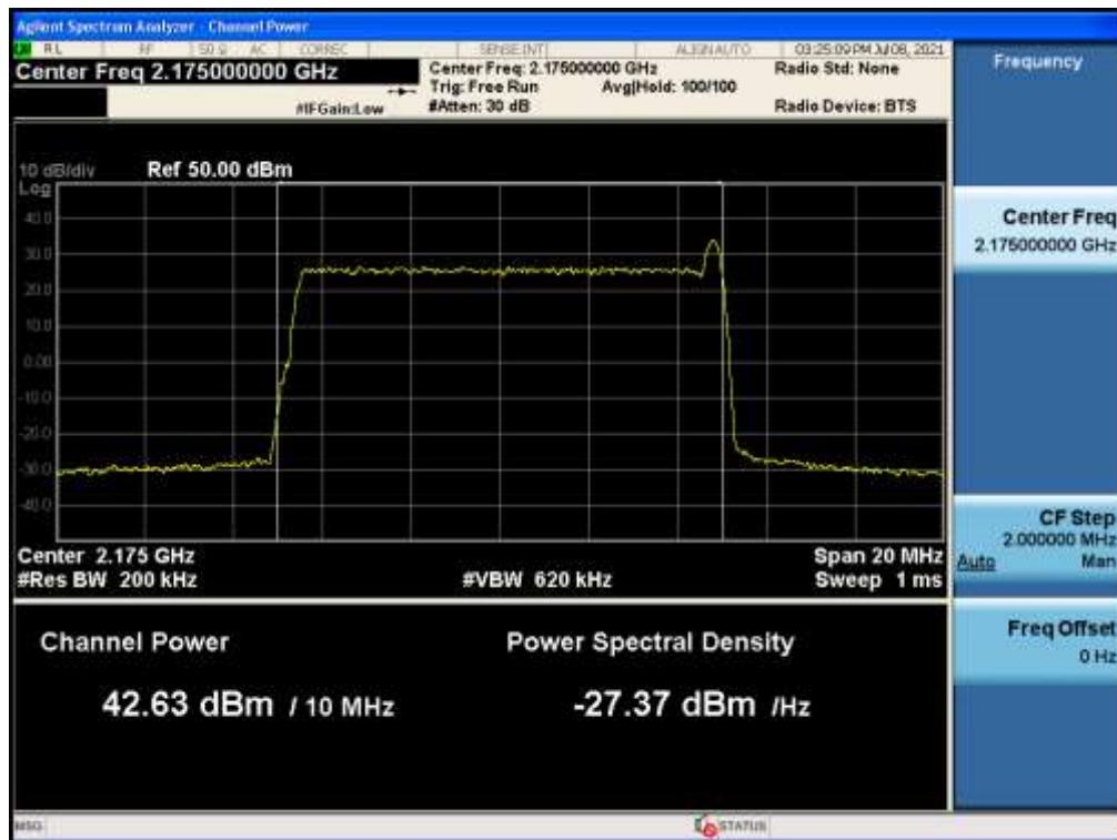
Antenna 1 / B25 LTE 5 MHz 1 Carrier + B25 LTE 5 MHz 1 Carrier + B25 LTE 20 MHz 1 Carrier [3 Carrier] (1C+2C) /
