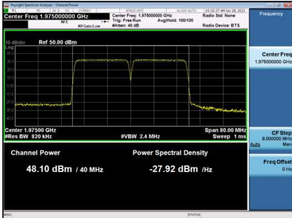
**Antenna 1 / B25 LTE 20 MHz & NB-IoT 1 Carrier + B25 LTE 20 MHz 1 Carrier [2 Carrier] / Contiguous / 256QAM / High**
