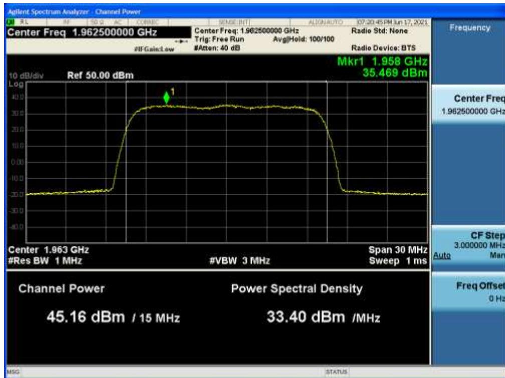
**Antenna 1 / B25 LTE 20 MHz 1 Carrier / 16QAM / High**
