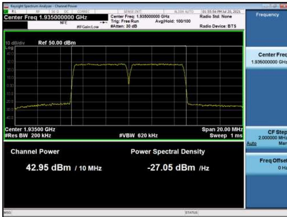
**Antenna 1 / B25 LTE 5 MHz 1 Carrier + B25 LTE 5 MHz 1 Carrier + B25 LTE 20 MHz & NB-IoT 1 Carrier [3 Carrier] (2C+1C) / Non-Contiguous / B25 LTE 20 MHz & NB-IoT / 256QAM / High**
