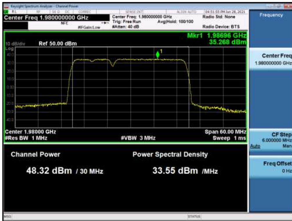
**Antenna 1 / B25 LTE 5 MHz 1 Carrier + B25 LTE 5 MHz 1 Carrier + B25 LTE 20 MHz & NB-IoT 1 Carrier [3 Carrier] / Contiguous / QPSK / Middle**
