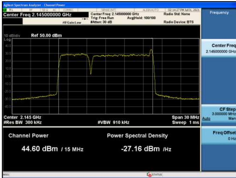
**Antenna 0 / B66 LTE 5 MHz 1 Carrier + B66 LTE 20 MHz 1 Carrier [2 Carrier] / Contiguous / QPSK / Middle**
