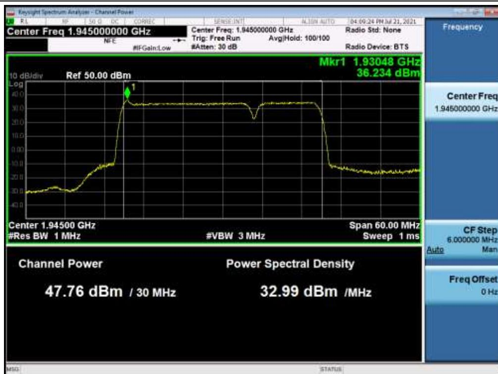
**Antenna 1 / B25 LTE 10 MHz & NB-IoT 1 Carrier + B25 LTE 20 MHz & NB-IoT 1 Carrier [2 Carrier] / Contiguous / 256QAM / Middle**
