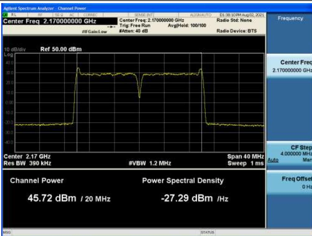
**Antenna 1 / B25 LTE 5 MHz 1 Carrier + B25 LTE 5 MHz 1 Carrier + B25 LTE 20 MHz 1 Carrier [3 Carrier] / Contiguous / 64QAM / High**
