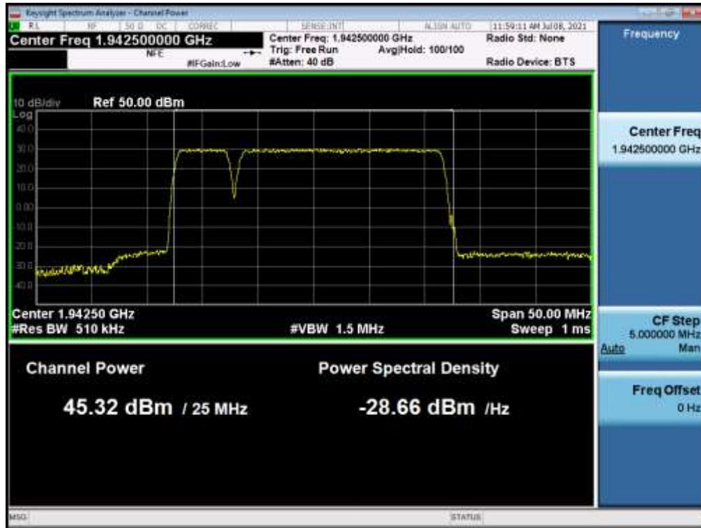
**Antenna 1 / B25 LTE 5 MHz 1 Carrier + B25 LTE 20 MHz 1 Carrier + B25 LTE 20 MHz 1 Carrier [3 Carrier] (2C+1C) / Non-Contiguous / B25 LTE 20 MHz / 64QAM / High**
