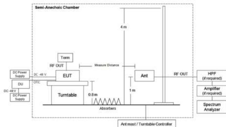
※ EUT position is adopted by placement of floor-standing refer to section 5.5.2.3.2 of ANSI C63.26-2015
