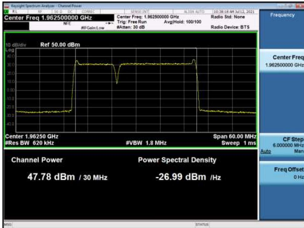
**Antenna 1 / B25 LTE 15 MHz 1 Carrier + B25 LTE 20 MHz 1 Carrier [2 Carrier] / Contiguous / 16QAM / Low**
