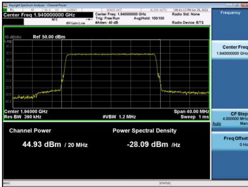
**Antenna 1 / B25 LTE 20 MHz 1 Carrier + B25 LTE 20 MHz 1 Carrier [2 Carrier] / Non-Contiguous / B25 LTE 20 MHz / 64QAM / High**
