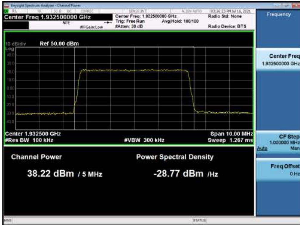
**Antenna 1 / B25 LTE 5 MHz 1 Carrier + B25 LTE 20 MHz 1 Carrier + B25 LTE 20 MHz & NB-IoT 1 Carrier [3 Carrier] (1C+2C) / Non-Contiguous / B25 LTE 20 MHz + B25 LTE 20 MHz & NB-IoT / QPSK / High**
