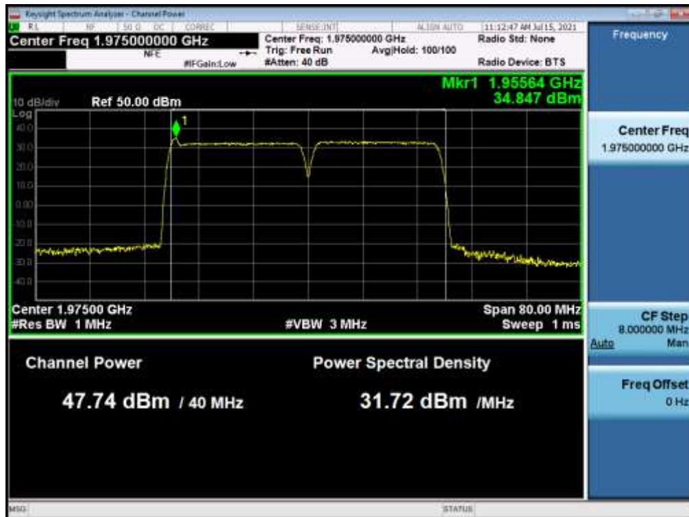
**Antenna 1 / B25 LTE 20 MHz & NB-IoT 1 Carrier + B25 LTE 20 MHz & NB-IoT 1 Carrier [2 Carrier] / Contiguous / 16QAM / Low**
