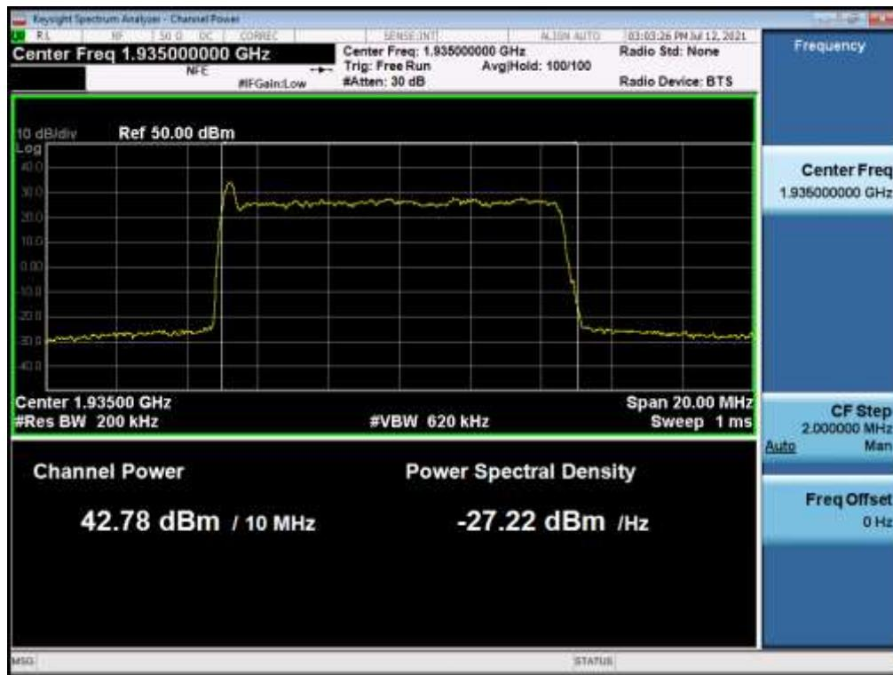
**Antenna 1 / B25 LTE 10 MHz & NB-IoT 1 Carrier + B25 LTE 20 MHz & NB-IoT 1 Carrier [2 Carrier] / Non-Contiguous /
