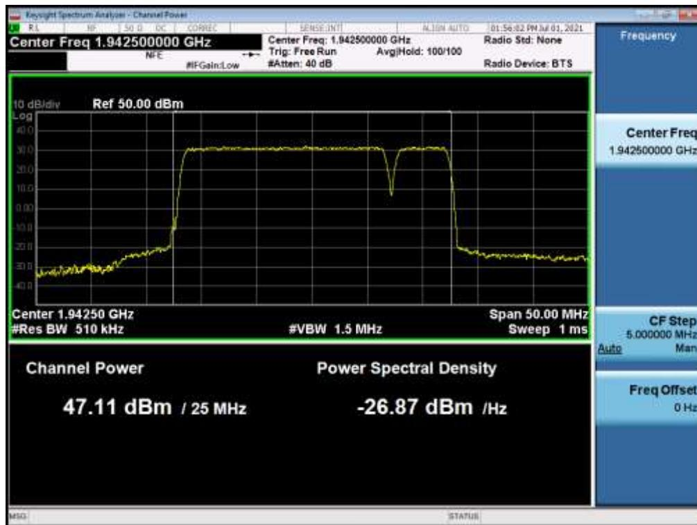
**Antenna 1 / B25 LTE 20 MHz 1 Carrier + B25 LTE 5 MHz 1 Carrier + B25 LTE 5 MHz 1 Carrier [3 Carrier] (2C+1C) / Non-Contiguous / B25 LTE 5 MHz / 256QAM / High**
