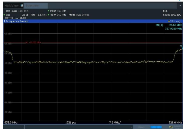
Plot 8-190. Conducted Spurious Emission Plot 652 MHz to 728 MHz (n71_2C_15M+20M+n85_2C_5M+10M_Dual-band - Mid Channel, Port 0)
