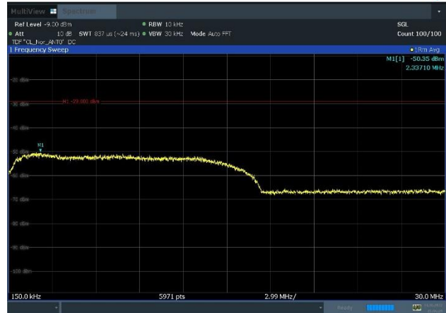
Plot 8-182. Conducted Spurious Emission Plot 150 kHz to 30 MHz (NR_n85_2C_5M+10M_NC_QPSK - Mid Channel, Port 0)
