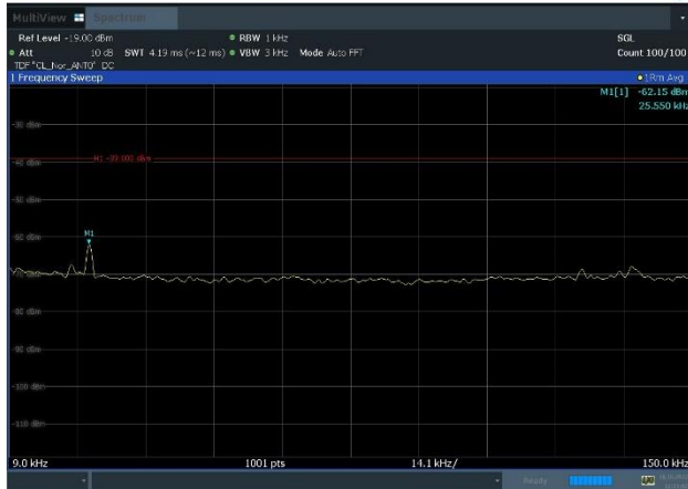
Plot 8-187. Conducted Spurious Emission Plot 9 kHz to 150 kHz (n71_2C_15M+20M+n85_2C_5M+10M_Dual-band - Mid Channel, Port 0)
