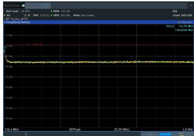
Plot 8-178. Conducted Spurious Emission Plot 746.1 MHz to 1 GHz (LTE_B85_2C_5M+10M_QPSK - Mid Channel, Port 0)
