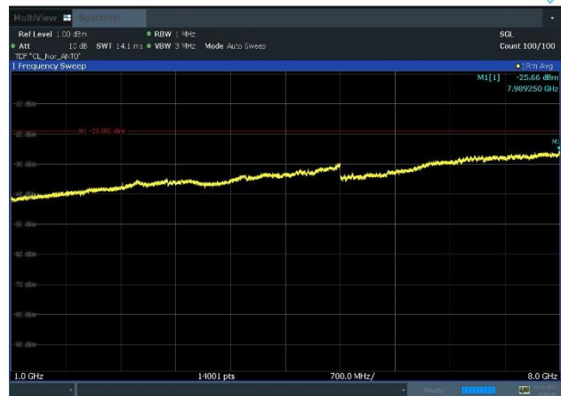
Plot 8-192. Conducted Spurious Emission Plot 1 GHz to 8 GHz (n71_2C_15M+20M+n85_2C_5M+10M_Dual-band - Mid Channel, Port 0)
