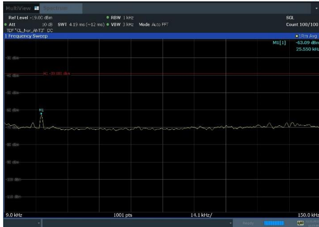
Plot 8-163. Conducted Spurious Emission Plot 9 kHz to 150 kHz (NR_n71_1C_20M_256QAM - High Channel, Port 3)
