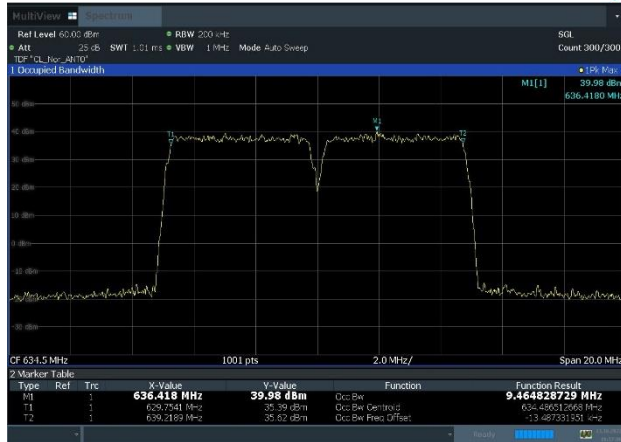
Plot 8-19. Occupied Bandwidth Plot (NR_n71_2C_5M+5M_QPSK – Mid Channel, Port 0)
