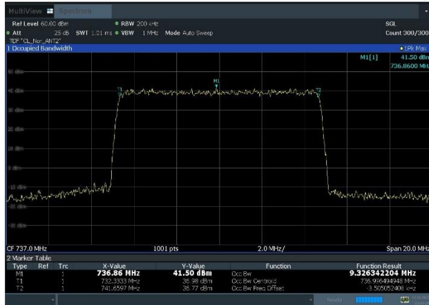
Plot 8-13. Occupied Bandwidth Plot (NR_n85_1C_10M_QPSK – Mid Channel, Port 2)
