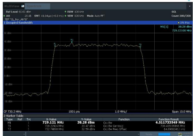
Plot 8-12. Occupied Bandwidth Plot (NR_n85_1C_10M_256QAM – Low Channel, Port 0)
