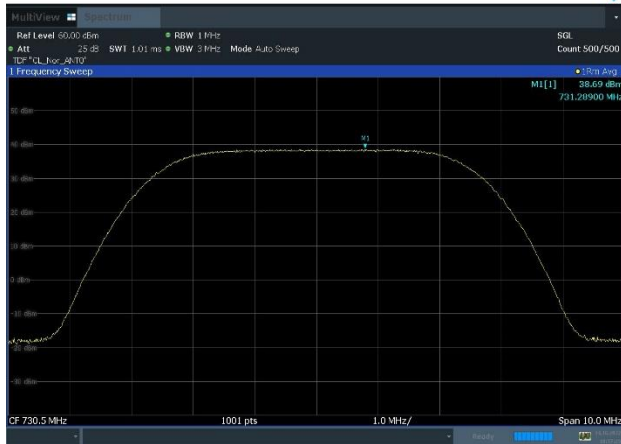
Plot 8-63. Power Spectral Density Plot (NR_n85_1C_5M_256QAM - Low Channel, Port 0)
