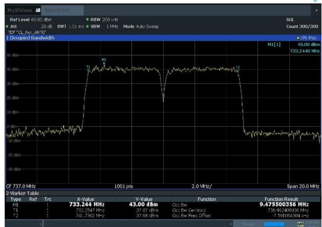
Plot 8-24. Occupied Bandwidth Plot (LTE_B85_2C_5M+5M_16QAM – Mid Channel, Port 0)
