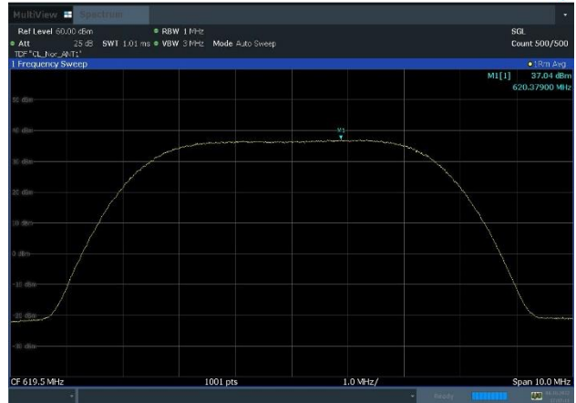
Plot 8-32. Power Spectral Density Plot (LTE_B71_1C_5M_16QAM - Low Channel, Port 1)
