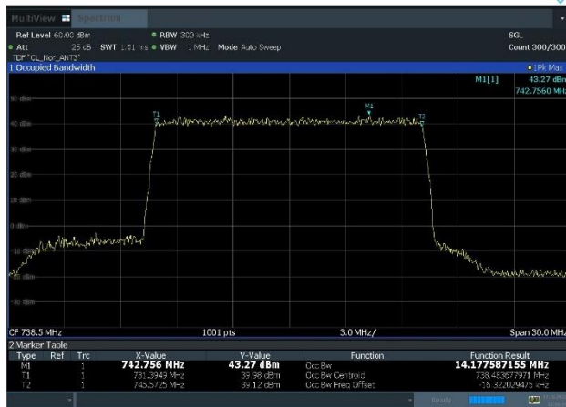
Plot 8-15. Occupied Bandwidth Plot (NR_n85_1C_15M_QPSK – High Channel, Port 3)
