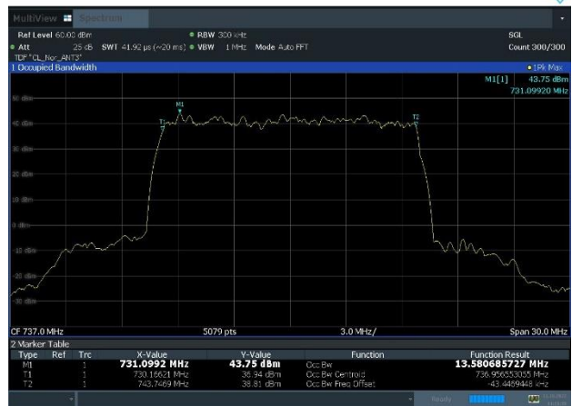
Plot 8-10. Occupied Bandwidth Plot (LTE_B85_1C_15M_16QAM – Mid Channel, Port 3)
