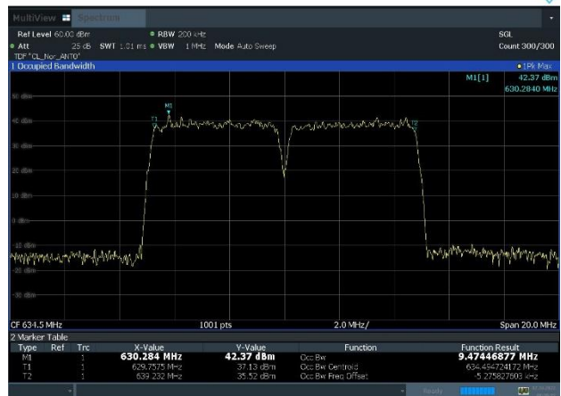
Plot 8-18. Occupied Bandwidth Plot (LTE_B71_2C_5M+5M_16QAM – Mid Channel, Port 0)
