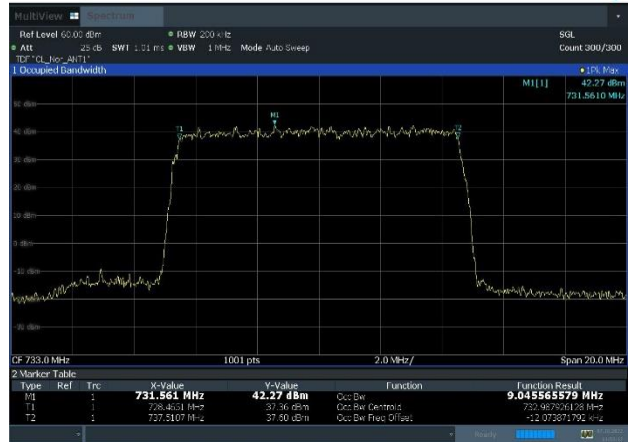
Plot 8-8. Occupied Bandwidth Plot (LTE_B85_1C_10M_16QAM – Low Channel, Port 1)
