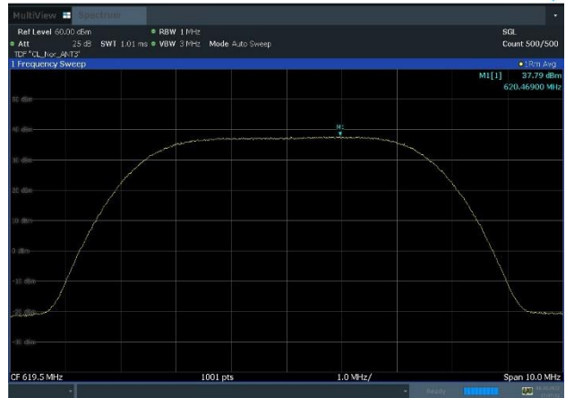
Plot 8-34. Power Spectral Density Plot (LTE_B71_1C_5M_16QAM - Low Channel, Port 3)
