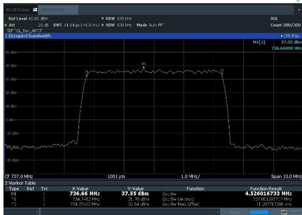
Plot 8-11. Occupied Bandwidth Plot (NR_n85_1C_5M_QPSK – Mid Channel, Port 3)
