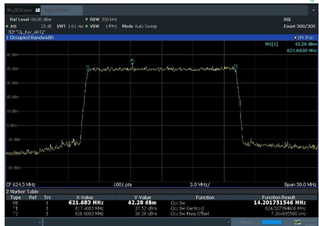
Plot 8-4. Occupied Bandwidth Plot (NR_n71_1C_15M_256QAM - Low Channel, Port 2)
