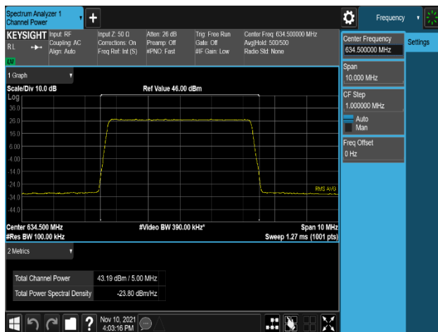
Plot 8-19. Conducted Average Output Power Plot (NR_n71_5M_64QAM - Mid Channel, Port 2)
