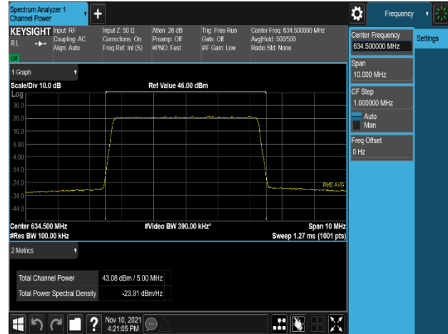
Plot 8-22. Conducted Average Output Power Plot (NR_n71_5M_256QAM - Mid Channel, Port 1)
