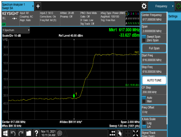
Plot 8-45. Lower Band Edge Emission Plot (NR_n71_10M_QPSK – Low Channel, Port 3)
