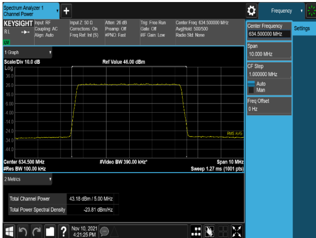
Plot 8-23. Conducted Average Output Power Plot (NR_n71_5M_256QAM - Mid Channel, Port 2)
