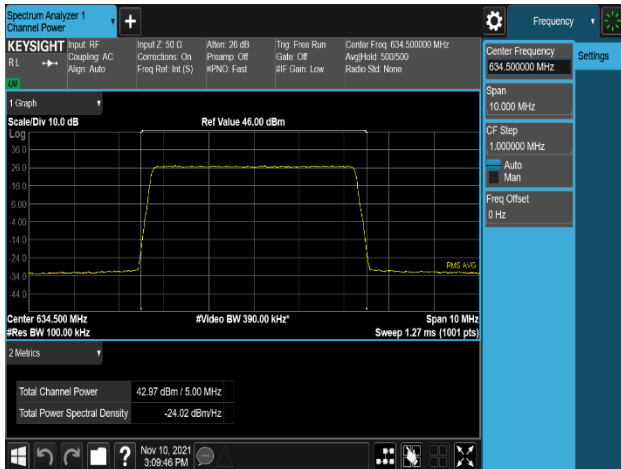
Plot 8-11. Conducted Average Output Power Plot (NR_n71_5M_QPSK - Mid Channel, Port 2)
