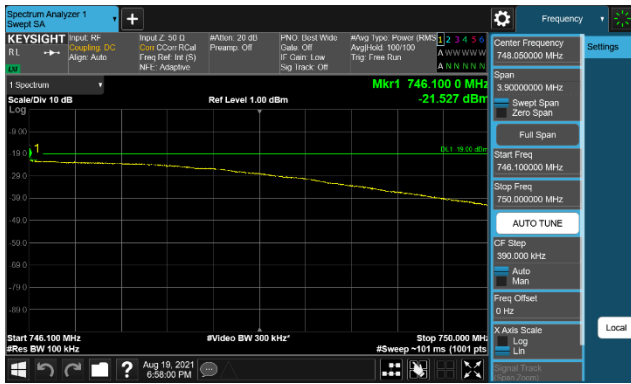
Plot 7-298. Conducted Spurious Emission Plot (746.1MHz to 750MHz) (Dual Band_71-85 B71 LTE 2C 10M+10M & B85 NB-IoT(SA) 1C + LTE 1C 5M + NB-IoT(SA) 1C - Port 3)
