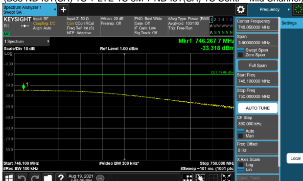
Plot 7-277. Conducted Spurious Emission Plot (746.1MHz to 750MHz) (B85 NB-IoT(SA) 1C + LTE 1C 5M + NB-IoT(SA) 1C Conti - Mid Channel)
