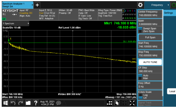
Plot 7-227. Conducted Spurious Emission Plot (746.1MHz to 750MHz) (B85 NB-IoT(SA) 2C Conti – High Channel)
