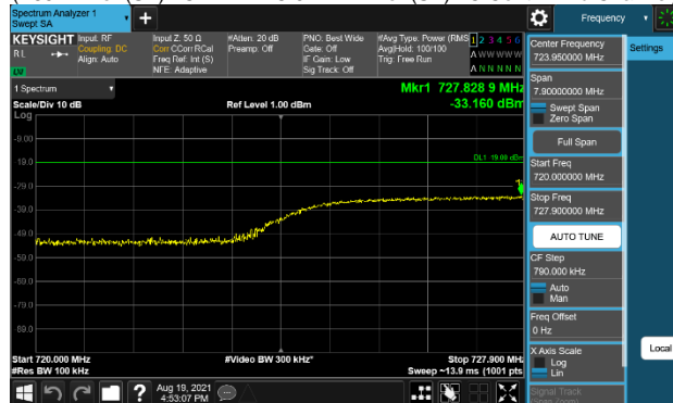
Plot 7-276. Conducted Spurious Emission Plot (720MHz to 727.9MHz) (B85 NB-IoT(SA) 1C + LTE 1C 5M + NB-IoT(SA) 1C Conti - Mid Channel)
