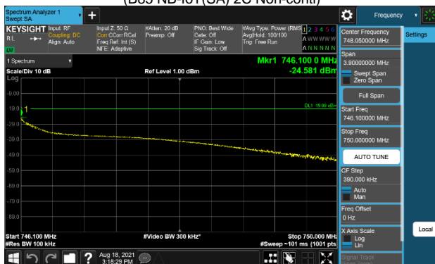
Plot 7-235. Conducted Spurious Emission Plot (746.1MHz to 750MHz) (B85 NB-IoT(SA) 2C Non-conti)
