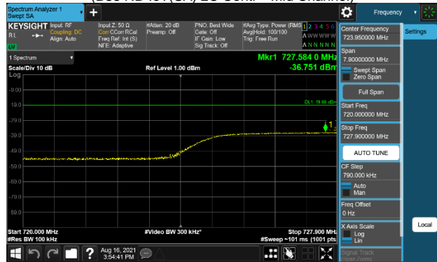
Plot 7-219. Conducted Spurious Emission Plot (720MHz to 727.9MHz) (B85 NB-IoT(SA) 2C Conti – Mid Channel)
