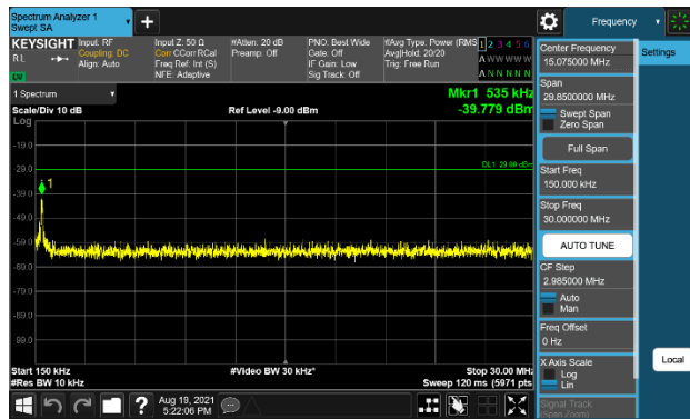
Plot 7-288. Conducted Spurious Emission Plot (150kHz to 30MHz) (B85 NB-IoT(SA) 1C + LTE 1C 5M + NB-IoT(SA) 1C Non-conti)
