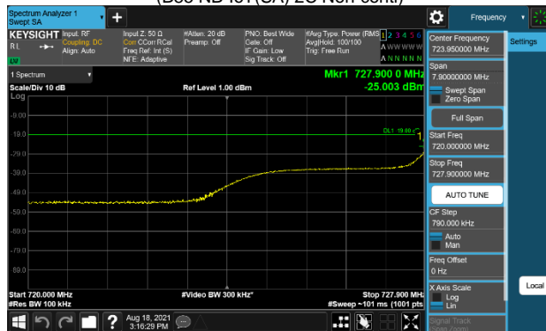
Plot 7-234. Conducted Spurious Emission Plot (720MHz to 727.9MHz) (B85 NB-IoT(SA) 2C Non-conti)
