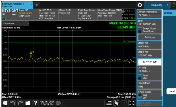
Plot 7-216. Conducted Spurious Emission Plot (9kHz to 150kHz) (B85 NB-IoT(SA) 2C Conti – Mid Channel)
