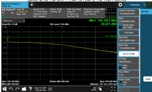
Plot 7-263. Conducted Spurious Emission Plot (746.1MHz to 750MHz) (B85 LTE 1C 5M + NB-IoT(SA) 1C Non-conti)
