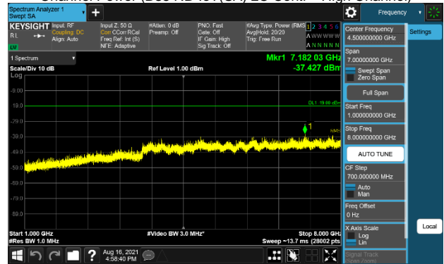
Plot 7-230. Conducted Spurious Emission Plot (1GHz to 8GHz) (B85 NB-IoT(SA) 2C Conti – High Channel)
