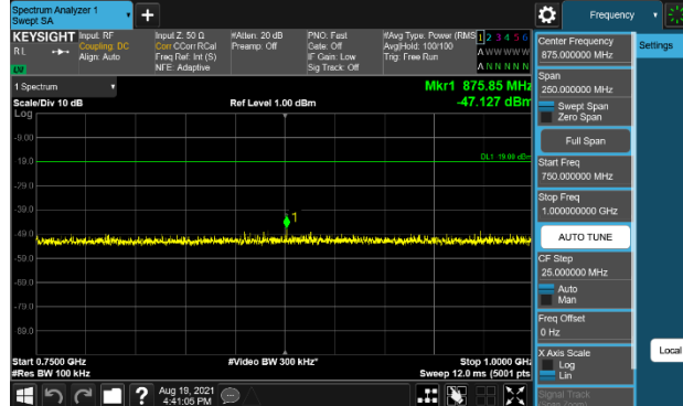
Plot 7-271. Conducted Spurious Emission Plot (750MHz to 1GHz) (B85 NB-IoT(SA) 1C + LTE 1C 5M + NB-IoT(SA) 1C Conti – Low Channel)
