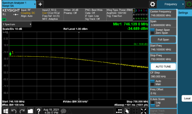
Plot 7-270. Conducted Spurious Emission Plot (746.1MHz to 750MHz) (B85 NB-IoT(SA) 1C + LTE 1C 5M + NB-IoT(SA) 1C Conti – Low Channel)
