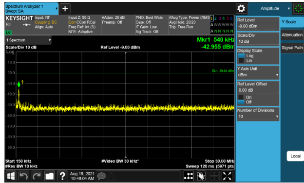
Plot 7-254. Conducted Spurious Emission Plot (150kHz to 30MHz) (B85 LTE 1C 5M + NB-IoT(SA) 1C Conti – High Channel)
