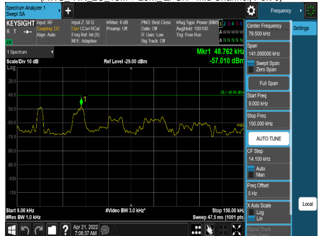
Plot 8-351. Conducted Spurious Emission Plot 9 kHz to 150 kHz (AWS_DSS_1C_15M + LTE_1C_5M_Non-Contiguous_QPSK - Mid Channel, Port 0)
