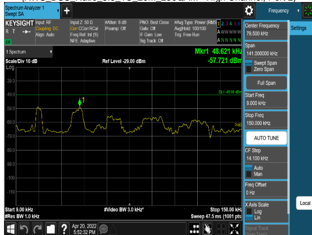
Plot 8-344. Conducted Spurious Emission Plot 9 kHz to 150 kHz (AWS_NR_2C_15M + 20M_QPSK - Mid Channel, Port 0)
