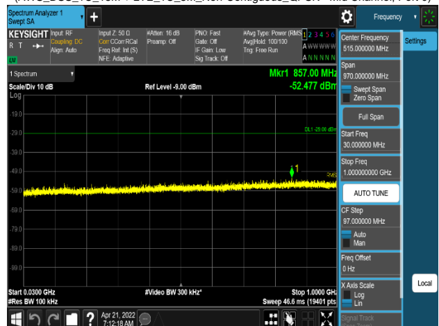
Plot 8-353. Conducted Spurious Emission Plot 30 MHz to 1 GHz (AWS_DSS_1C_15M + LTE_1C_5M_Non-Contiguous_QPSK - Mid Channel, Port 0)
