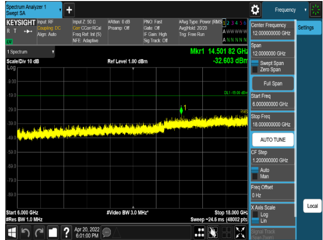
Plot 8-349. Conducted Spurious Emission Plot 6 GHz to 18 GHz (AWS_NR_2C_15M + 20M_QPSK - Mid Channel, Port 0)
