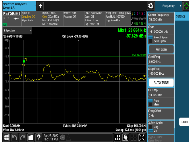
Plot 8-330. Conducted Spurious Emission Plot 9 kHz to 150 kHz (AWS_NR_1C_20M_64QAM - Low Channel, Port 3)
