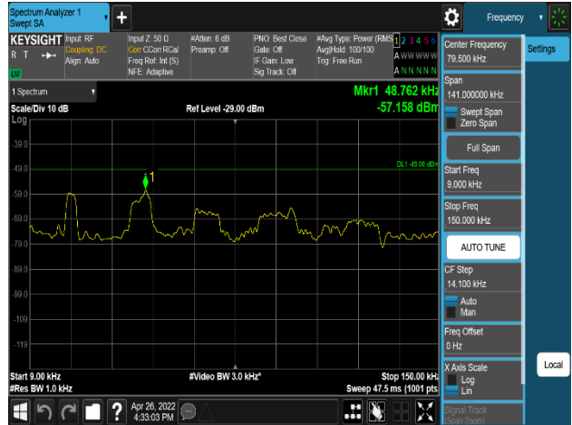
Plot 8-337. Conducted Spurious Emission Plot 9 kHz to 150 kHz (AWS_DSS_Ratio_5:5_1C_20M_256QAM - High Channel, Port 2)
