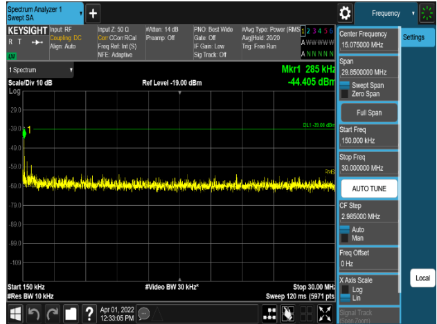
Plot 8-331. Conducted Spurious Emission Plot 150 kHz to 30 MHz (AWS_NR_1C_20M_64QAM - Low Channel, Port 3)
