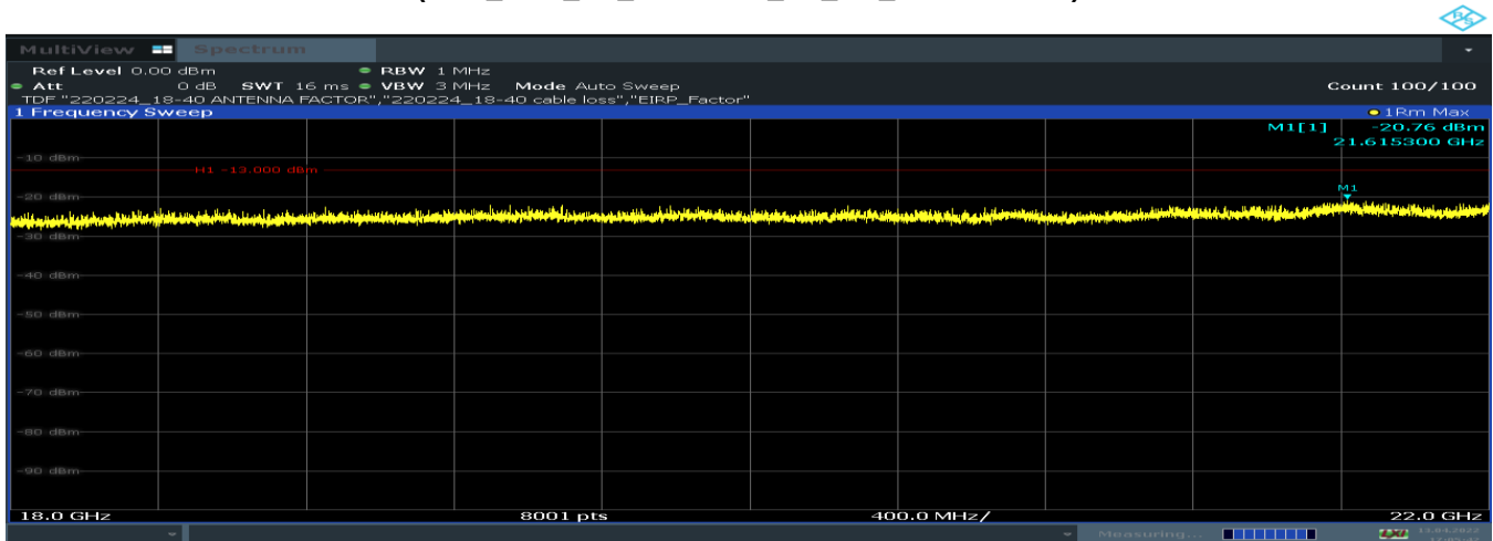
Plot 8-371. Radiated spurious emission Plot_18 GHz to 22 GHz (PCS_DSS_1C_20M + NR_1C_5M_Mid Channel)
