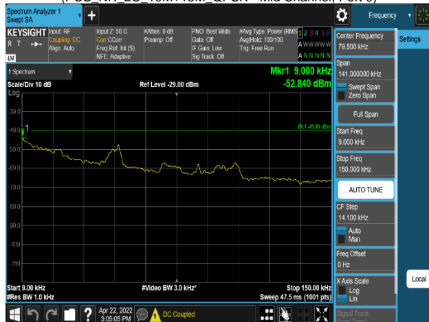
Plot 8-316. Conducted Spurious Emission Plot 9 kHz to 150 kHz (PCS_NR_2C_5M+5M_Non-Contiguous_QPSK - Mid Channel, Port 0)
