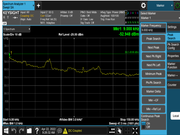
Plot 8-288. Conducted Spurious Emission Plot 9 kHz to 150 kHz (PCS_NR_1C_5M_256QAM - Low Channel, Port 3)
