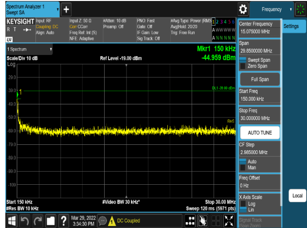
Plot 8-289. Conducted Spurious Emission Plot 150 kHz to 30 MHz (PCS_NR_1C_5M_256QAM - Low Channel, Port 3)
