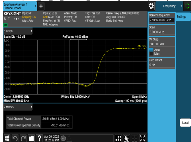
Plot 8-285. Band Edge Emission Plot (AWS NR 2C 15M + 20M Non-Cont QPSK - Low Channel, Port 0)
