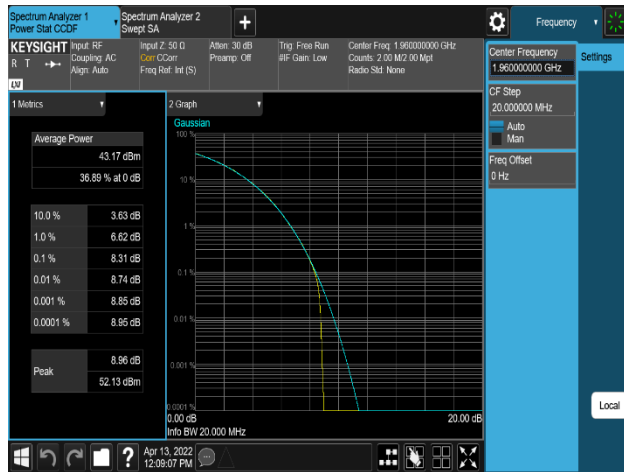
Plot 8-211. Peak To Average Power Ratio Plot (DSS_1C_15M + LTE_1C_5M_16QAM - Mid Channel, Port 0)
