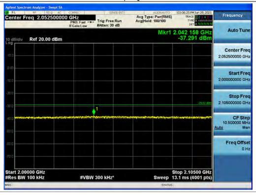
Antenna 0 / High Edge + 100 MHz ~ 2 GHz (10 GHz) / B2 DSS 10 MHz + B66 LTE (10 MHz+5 MHz) (40W+120W)\_Near / Inter Band / 16QAM
