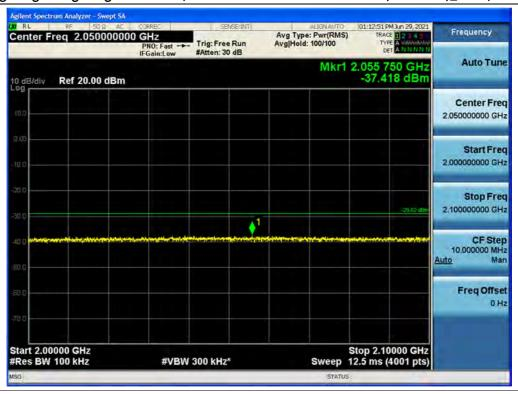
Antenna 0 / High Edge + 100 MHz ~ 2 GHz (10 GHz) / B2 DSS 10 MHz + B66 LTE 10 MHz (80W+80W)\_Near / Inter Band / 64QAM
