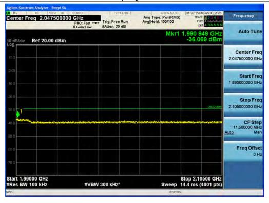
Antenna 0 / High Edge + 100 MHz ~ 2 GHz (10 GHz) / B2 DSS 10 MHz + B66 LTE (10 MHz+5 MHz) (40W+120W)\_Far / Inter Band / 16QAM
