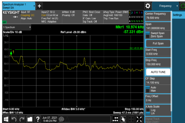
Plot 7-2605. Conducted Spurious Emission Plot 9 kHz to 150 kHz (B2_20M+5M + B66_20M_QPSK - High Channel, Port 1)
