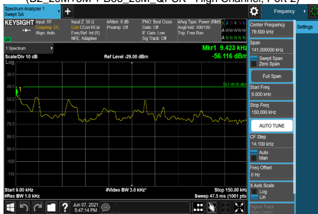
Plot 7-2621. Conducted Spurious Emission Plot 9 kHz to 150 kHz (B2_20M+5M + B66_20M_QPSK - High Channel, Port 3)
