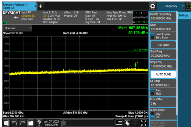
Plot 7-2623. Conducted Spurious Emission Plot 30 MHz to 1 GHz (B2_20M+5M + B66_20M_QPSK - High Channel, Port 3)
