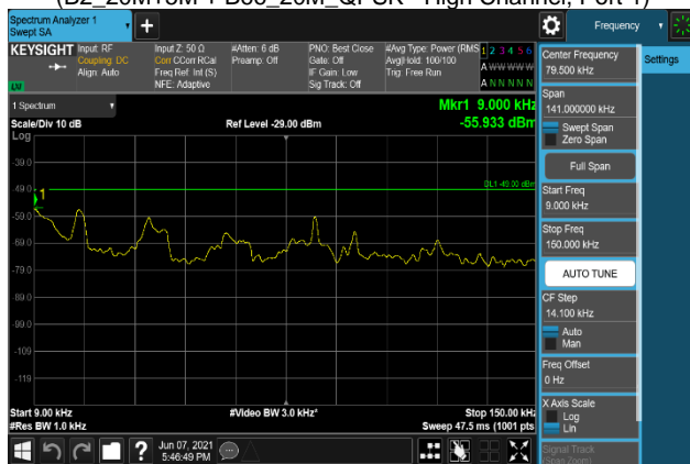
Plot 7-2613. Conducted Spurious Emission Plot 9 kHz to 150 kHz (B2_20M+5M + B66_20M_QPSK - High Channel, Port 2)
