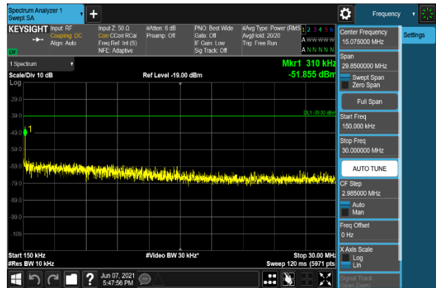
Plot 7-2606. Conducted Spurious Emission Plot 150 kHz to 30 MHz (B2_20M+5M + B66_20M_QPSK - High Channel, Port 1)
