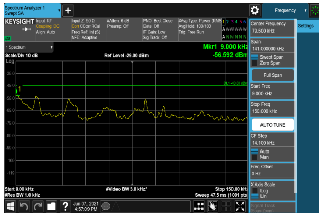
Plot 7-2557. Conducted Spurious Emission Plot 9 kHz to 150 kHz (B2_20M+5M + B66_20M_QPSK - Low Channel, Port 3)
