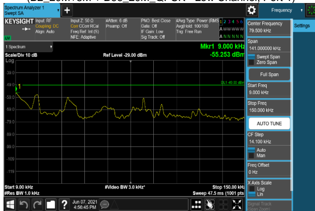
Plot 7-2549. Conducted Spurious Emission Plot 9 kHz to 150 kHz (B2_20M+5M + B66_20M_QPSK - Low Channel, Port 2)
