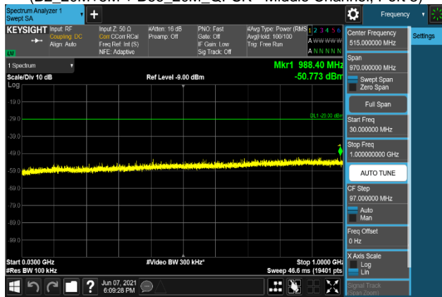
Plot 7-2591. Conducted Spurious Emission Plot 30 MHz to 1 GHz (B2_20M+5M + B66_20M_QPSK - Middle Channel, Port 3)
