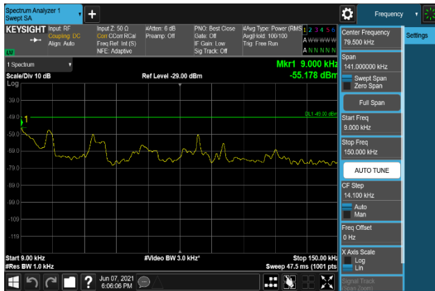
Plot 7-2581. Conducted Spurious Emission Plot 9 kHz to 150 kHz (B2_20M+5M + B66_20M_QPSK - Middle Channel, Port 2)
