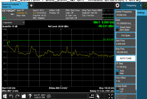
Plot 7-2589. Conducted Spurious Emission Plot 9 kHz to 150 kHz (B2_20M+5M + B66_20M_QPSK - Middle Channel, Port 3)
