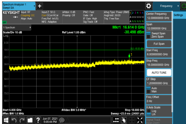
Plot 7-2563. Conducted Spurious Emission Plot 6 GHz to 18 GHz (B2_20M+5M + B66_20M_QPSK - Low Channel, Port 3)
