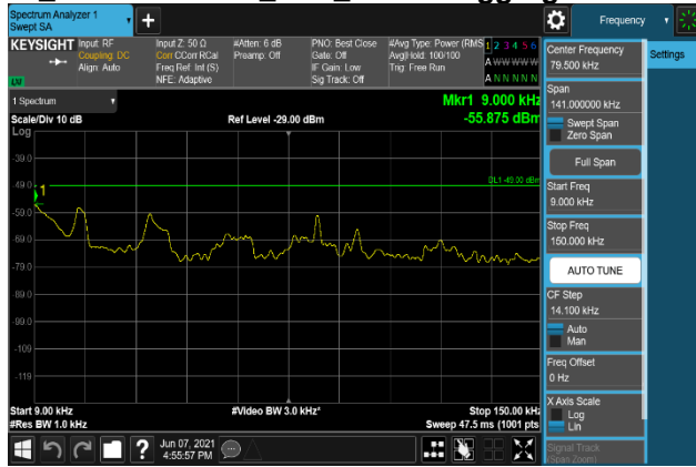
Plot 7-2533. Conducted Spurious Emission Plot 9 kHz to 150 kHz (B2_20M+5M + B66_20M_QPSK - Low Channel, Port 0)
