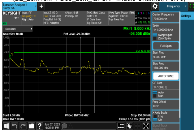
Plot 7-2573. Conducted Spurious Emission Plot 9 kHz to 150 kHz (B2_20M+5M + B66_20M_QPSK - Middle Channel, Port 1)
