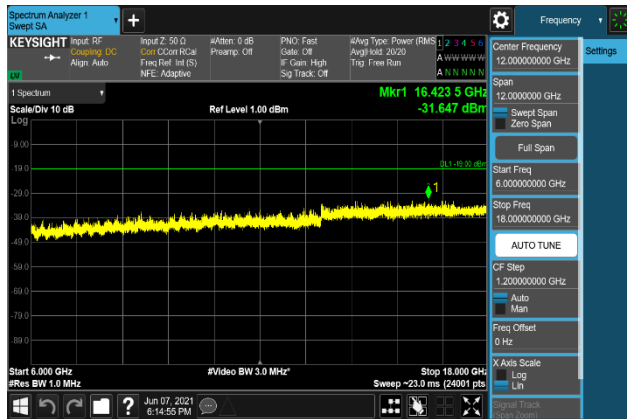
Plot 7-2587. Conducted Spurious Emission Plot 6 GHz to 18 GHz (B2_20M+5M + B66_20M_QPSK - Middle Channel, Port 2)
