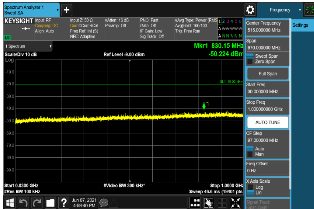
Plot 7-2551. Conducted Spurious Emission Plot 30 MHz to 1 GHz (B2_20M+5M + B66_20M_QPSK - Low Channel, Port 2)
