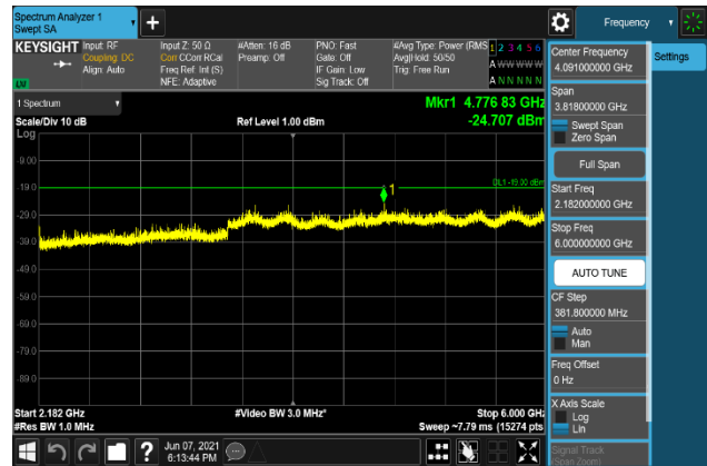
Plot 7-2594. Conducted Spurious Emission Plot 2.182 GHz to 6 GHz (B2_20M+5M + B66_20M_QPSK - Middle Channel, Port 3)
