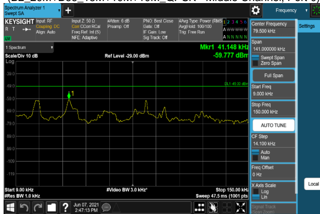
Plot 7-2477. Conducted Spurious Emission Plot 9 kHz to 150 kHz (B2_20M+B66_15M+10M+10M_QPSK - Middle Channel, Port 1)
