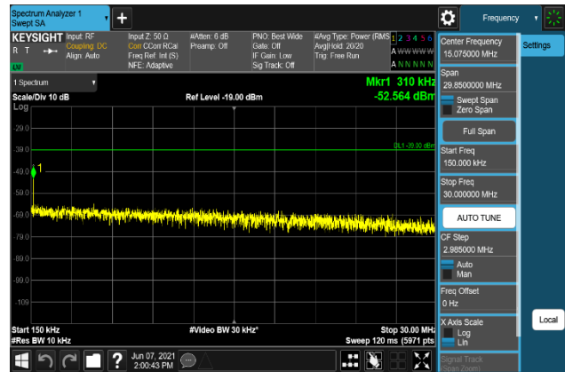
Plot 7-2462. Conducted Spurious Emission Plot 150 kHz to 30 MHz (B2_20M + B66_15M+10M+10M_QPSK - Low Channel, Port 3)
