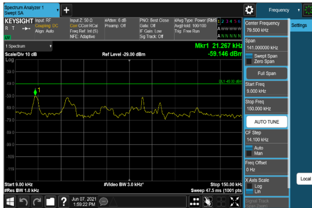
Plot 7-2461. Conducted Spurious Emission Plot 9 kHz to 150 kHz (B2_20M + B66_15M+10M+10M_QPSK - Low Channel, Port 3)
