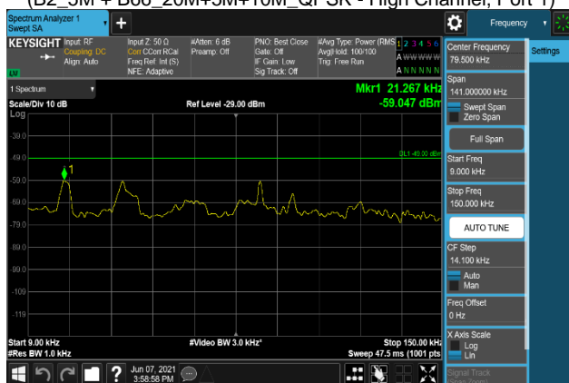
Plot 7-2421. Conducted Spurious Emission Plot 9 kHz to 150 kHz (B2_5M + B66_20M+5M+10M_QPSK - High Channel, Port 2)
