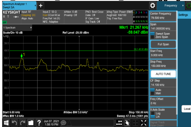
Plot 7-2437. Conducted Spurious Emission Plot 9 kHz to 150 kHz
