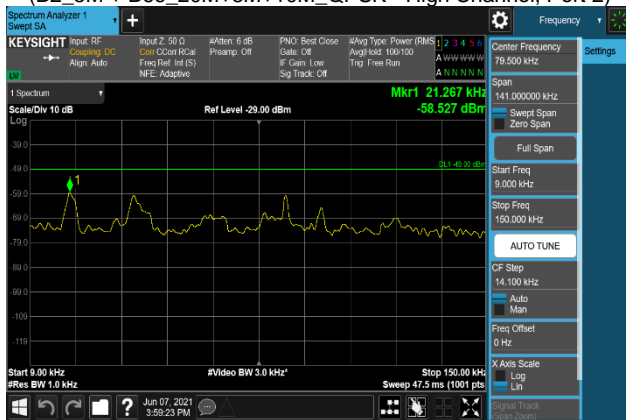
Plot 7-2429. Conducted Spurious Emission Plot 9 kHz to 150 kHz (B2_5M + B66_20M+5M+10M_QPSK - High Channel, Port 3)
