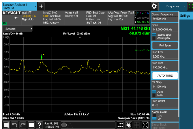
Plot 7-2413. Conducted Spurious Emission Plot 9 kHz to 150 kHz
