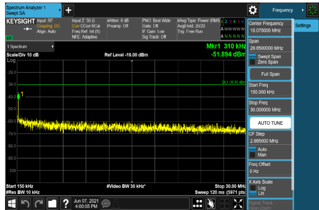
Plot 7-2414. Conducted Spurious Emission Plot 150 kHz to 30 MHz
