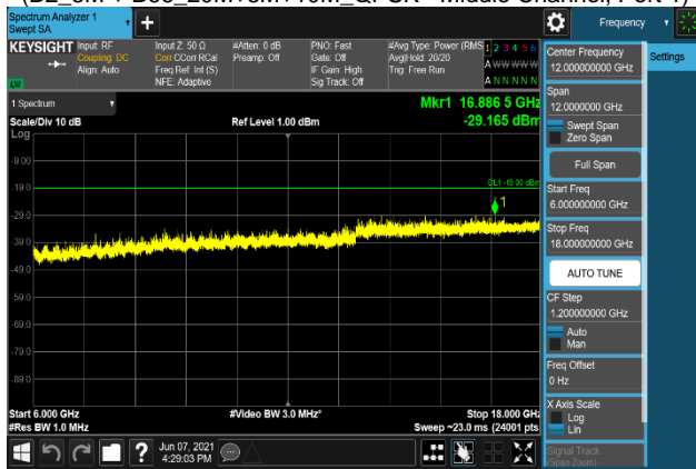
Plot 7-2387. Conducted Spurious Emission Plot 6 GHz to 18 GHz
