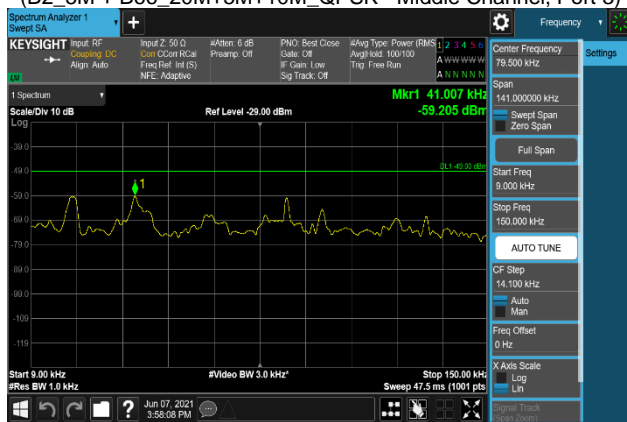
Plot 7-2405. Conducted Spurious Emission Plot 9 kHz to 150 kHz (B2_5M + B66_20M+5M+10M_QPSK - High Channel, Port 0)
