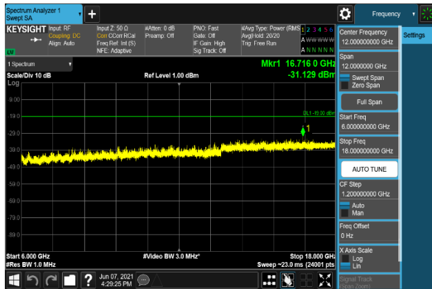
Plot 7-2395. Conducted Spurious Emission Plot 6 GHz to 18 GHz
