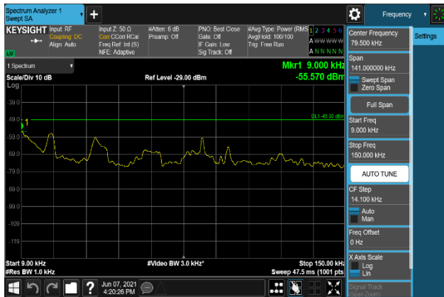
Plot 7-2389. Conducted Spurious Emission Plot 9 kHz to 150 kHz
