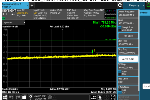
Plot 7-2439. Conducted Spurious Emission Plot 30 MHz to 1 GHz
