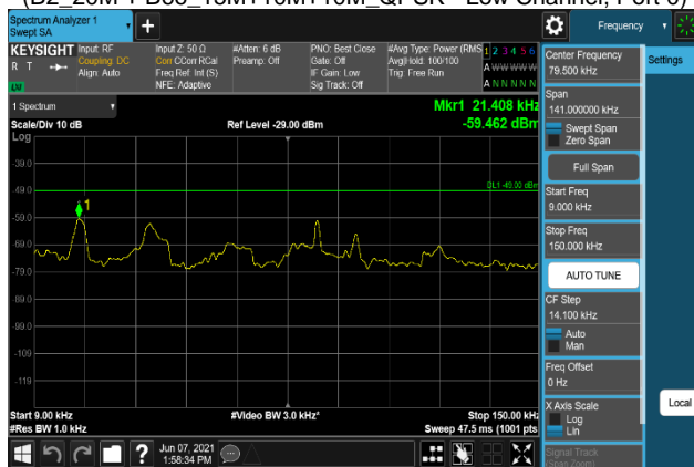
Plot 7-2445. Conducted Spurious Emission Plot 9 kHz to 150 kHz
