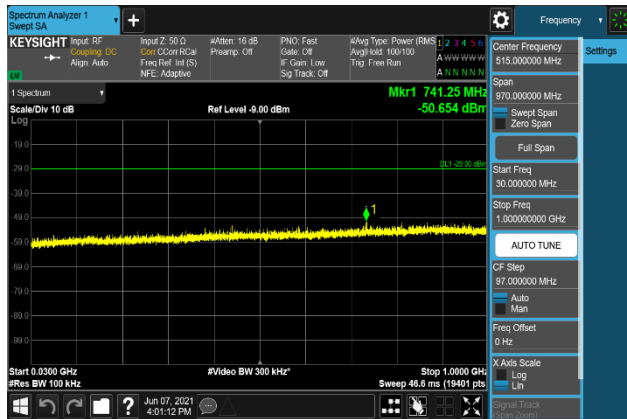
Plot 7-2407. Conducted Spurious Emission Plot 30 MHz to 1 GHz
