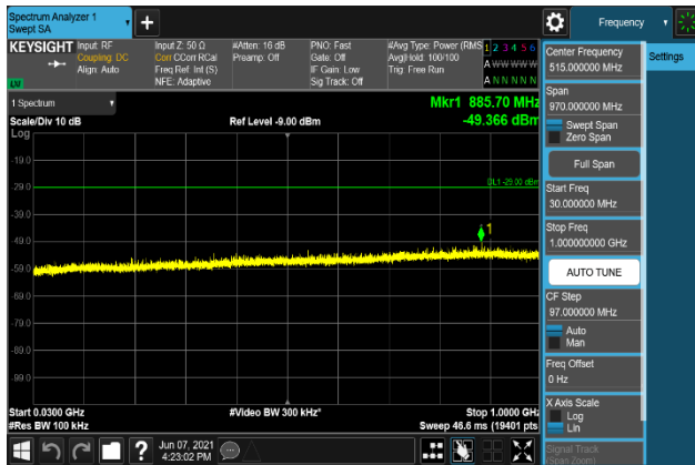
Plot 7-2383. Conducted Spurious Emission Plot 30 MHz to 1 GHz
