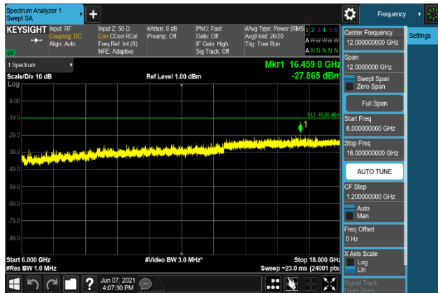
Plot 7-2419. Conducted Spurious Emission Plot 6 GHz to 18 GHz (B2_5M + B66_20M+5M+10M_QPSK - High Channel, Port 1)
