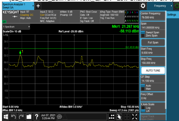
Plot 7-2357. Conducted Spurious Emission Plot 9 kHz to 150 kHz (B2_5M + B66_20M+5M+10M_QPSK - Low Channel, Port 2)
