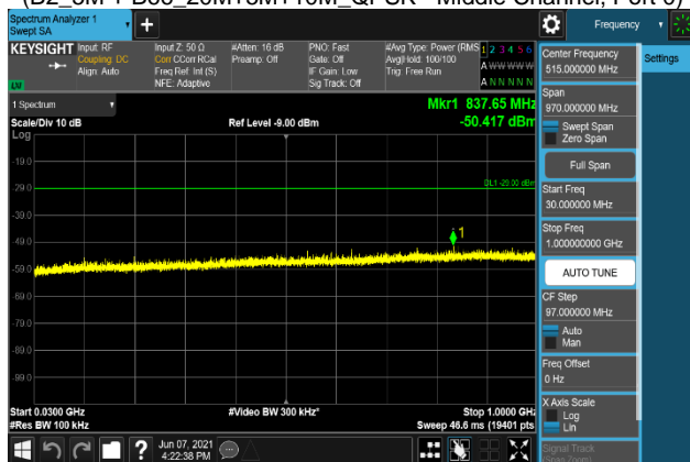
Plot 7-2375. Conducted Spurious Emission Plot 30 MHz to 1 GHz
