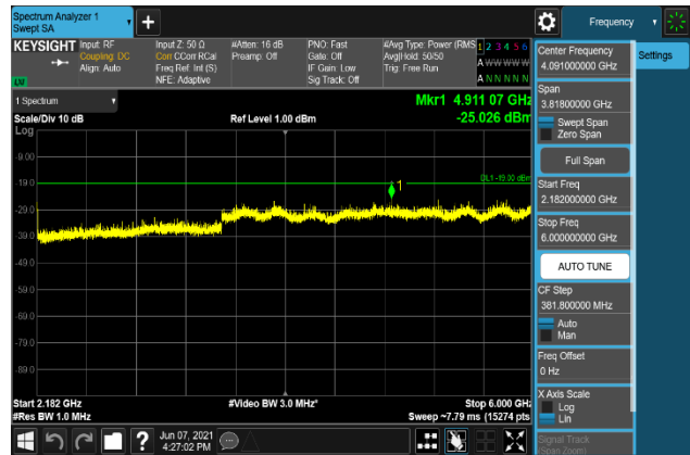
Plot 7-2378. Conducted Spurious Emission Plot 2.182 GHz to 6 GHz (B2_5M + B66_20M+5M+10M_QPSK - Middle Channel, Port 0)
