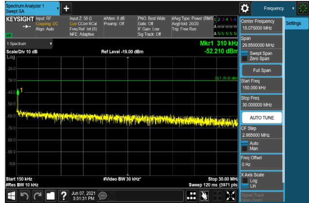
Plot 7-2366. Conducted Spurious Emission Plot 150 kHz to 30 MHz
