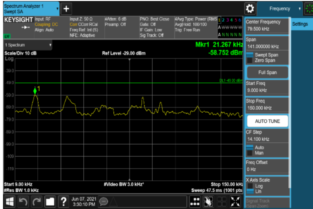
Plot 7-2365. Conducted Spurious Emission Plot 9 kHz to 150 kHz
