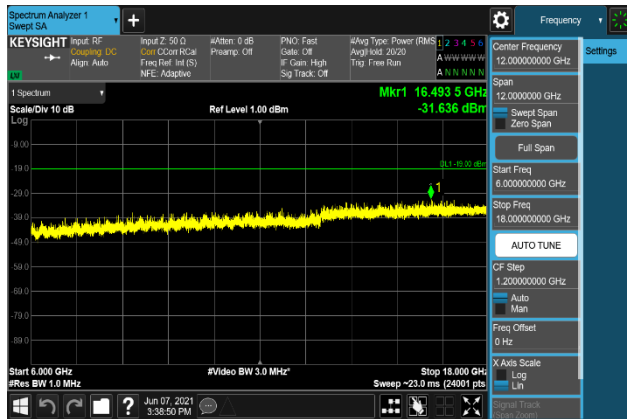
Plot 7-2371. Conducted Spurious Emission Plot 6 GHz to 18 GHz
