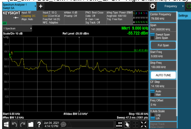
Plot 7-2333. Conducted Spurious Emission Plot 9 kHz to 150 kHz (B2_5M + B66_15M+10M+10M_QPSK - High Channel, Port 3)
