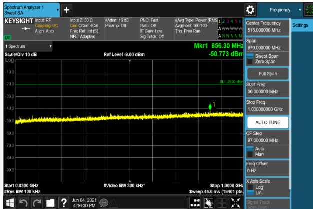
Plot 7-2311. Conducted Spurious Emission Plot 30 MHz to 1 GHz
