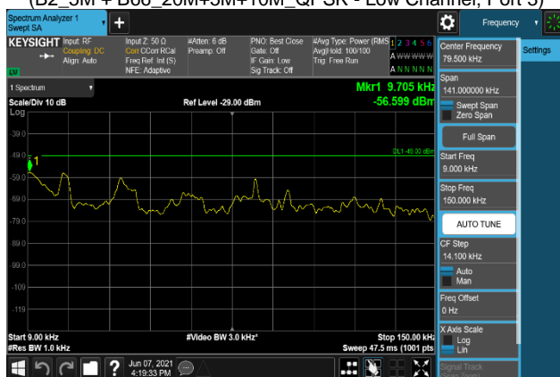
Plot 7-2373. Conducted Spurious Emission Plot 9 kHz to 150 kHz
