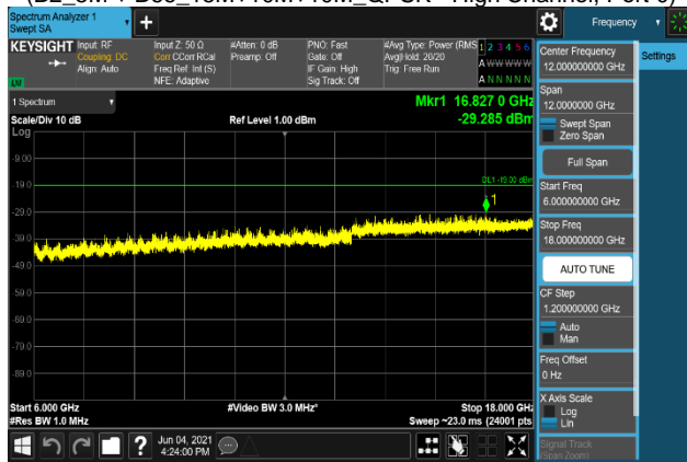
Plot 7-2315. Conducted Spurious Emission Plot 6 GHz to 18 GHz
