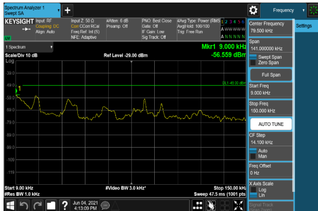
Plot 7-2317. Conducted Spurious Emission Plot 9 kHz to 150 kHz
