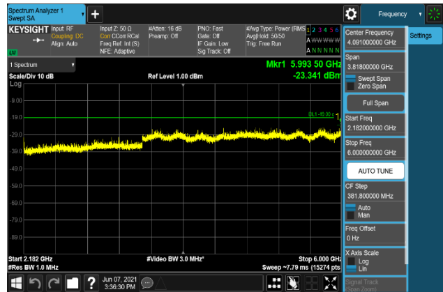
Plot 7-2354. Conducted Spurious Emission Plot 2.182 GHz to 6 GHz (B2_5M + B66_20M+5M+10M_QPSK - Low Channel, Port 1)
