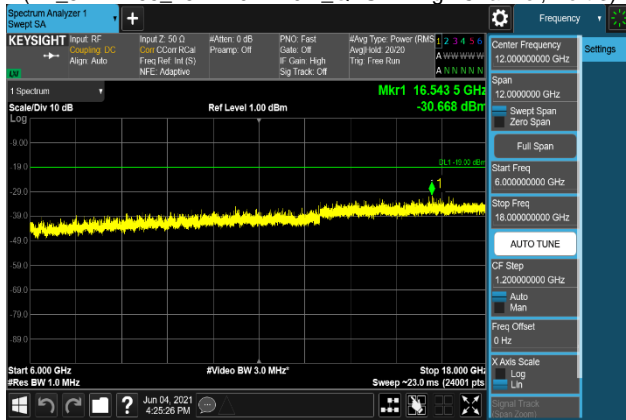
Plot 7-2339. Conducted Spurious Emission Plot 6 GHz to 18 GHz
