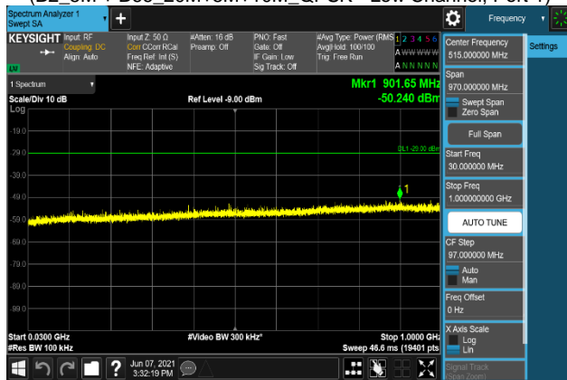
Plot 7-2351. Conducted Spurious Emission Plot 30 MHz to 1 GHz (B2_5M + B66_20M+5M+10M_QPSK - Low Channel, Port 1)
