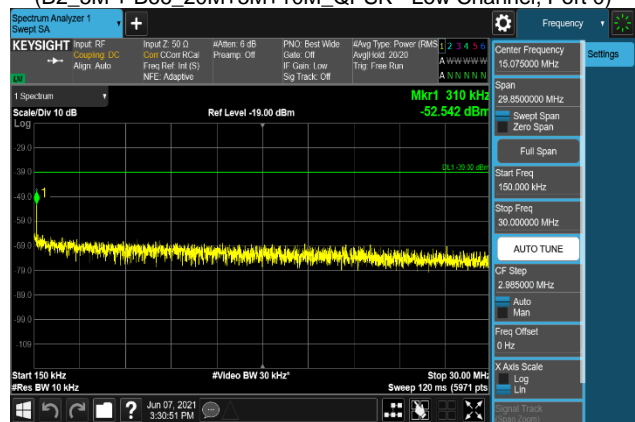
Plot 7-2350. Conducted Spurious Emission Plot 150 kHz to 30 MHz (B2_5M + B66_20M+5M+10M_QPSK - Low Channel, Port 1)
