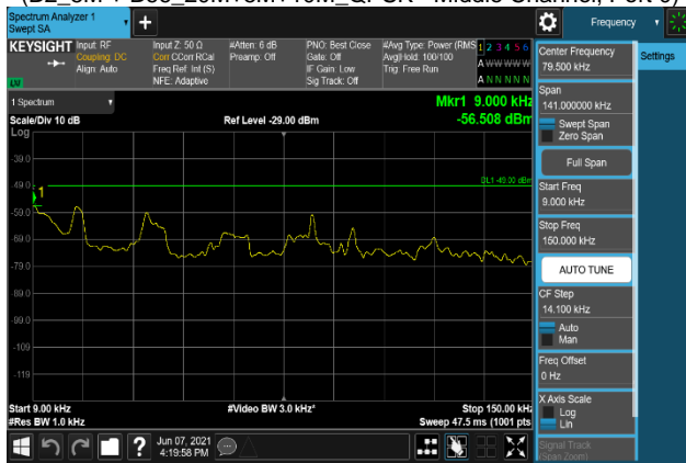
Plot 7-2381. Conducted Spurious Emission Plot 9 kHz to 150 kHz (B2_5M + B66_20M+5M+10M_QPSK - Middle Channel, Port 1)
