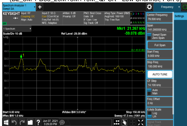
Plot 7-2349. Conducted Spurious Emission Plot 9 kHz to 150 kHz (B2_5M + B66_20M+5M+10M_QPSK - Low Channel, Port 1)
