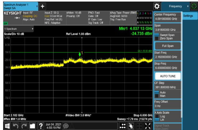
Plot 7-2282. Conducted Spurious Emission Plot 2.182 GHz to 6 GHz (B2_5M + B66_15M+10M+10M_QPSK - Middle Channel, Port 0)
