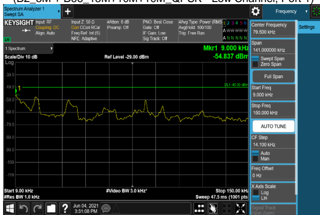
Plot 7-2261. Conducted Spurious Emission Plot 9 kHz to 150 kHz (B2_5M + B66_15M+10M+10M_QPSK - Low Channel, Port 2)
