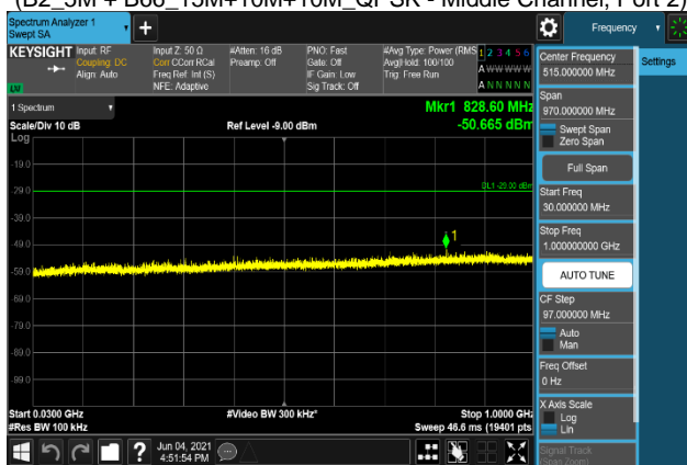
Plot 7-2295. Conducted Spurious Emission Plot 30 MHz to 1 GHz (B2_5M + B66_15M+10M+10M_QPSK - Middle Channel, Port 2)
