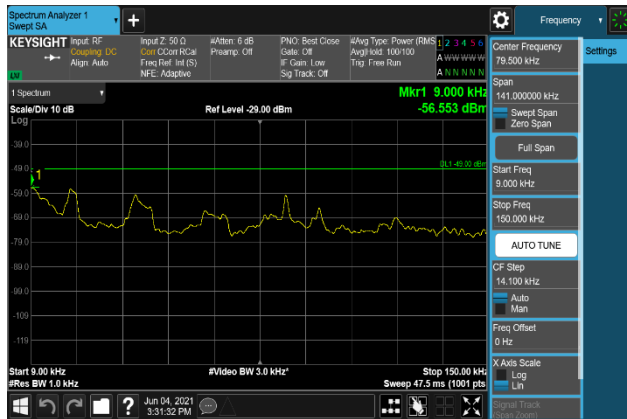
Plot 7-2269. Conducted Spurious Emission Plot 9 kHz to 150 kHz (B2_5M + B66_15M+10M+10M_QPSK - Low Channel, Port 3)
