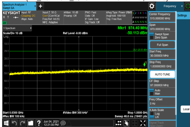
Plot 7-2227. Conducted Spurious Emission Plot 30 MHz to 1 GHz (B2_20M+5M_64QAM - Low Channel, Port 3)
