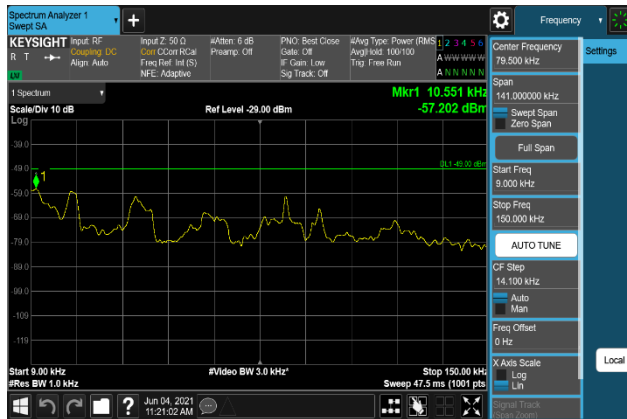
Plot 7-2217. Conducted Spurious Emission Plot 9 kHz to 150 kHz (B2_20M+5M_QPSK - Low Channel, Port 3)
