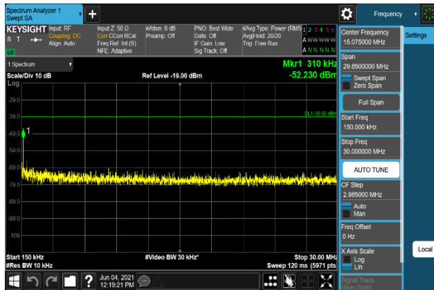
Plot 7-2223. Conducted Spurious Emission Plot 150 kHz to 30 MHz (B2_20M+5M_64QAM - Low Channel, Port 3)
