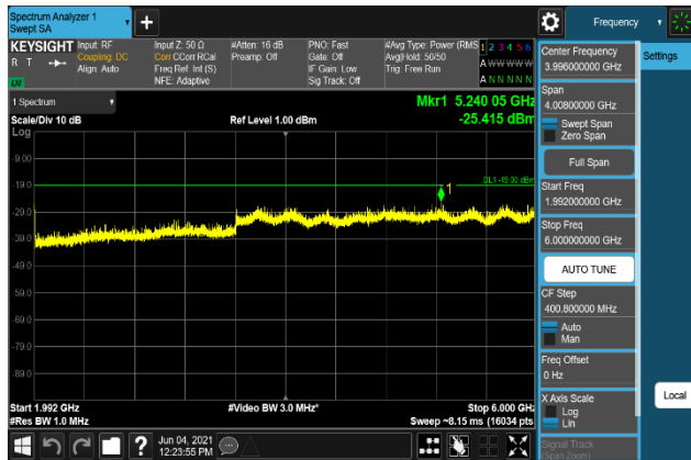
Plot 7-2235. Conducted Spurious Emission Plot 1.992 GHz to 6 GHz (B2_20M+5M_64QAM - Low Channel, Port 3)
