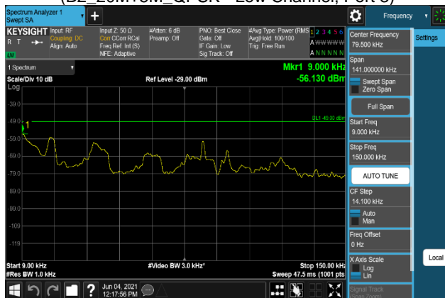
Plot 7-2219. Conducted Spurious Emission Plot 9 kHz to 150 kHz (B2_20M+5M_64QAM - Low Channel, Port 3)
