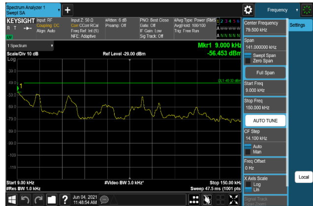
Plot 7-2218. Conducted Spurious Emission Plot 9 kHz to 150 kHz (B2_20M+5M_16QAM - Low Channel, Port 3)
