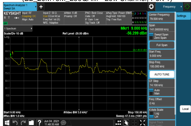
Plot 7-2190. Conducted Spurious Emission Plot 9 kHz to 150 kHz (B2_20M+5M_256QAM - Low Channel, Port 2)
