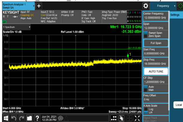
Plot 7-2239. Conducted Spurious Emission Plot 6 GHz to 18 GHz (B2_20M+5M_64QAM - Low Channel, Port 3)
