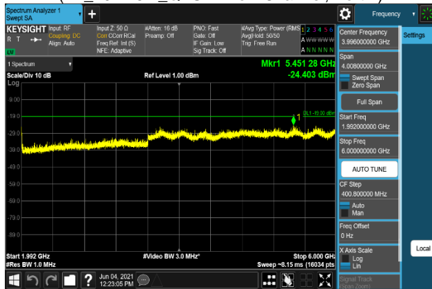
Plot 7-2179. Conducted Spurious Emission Plot 1.992 GHz to 6 GHz (B2_20M+5M_64QAM - Low Channel, Port 1)
