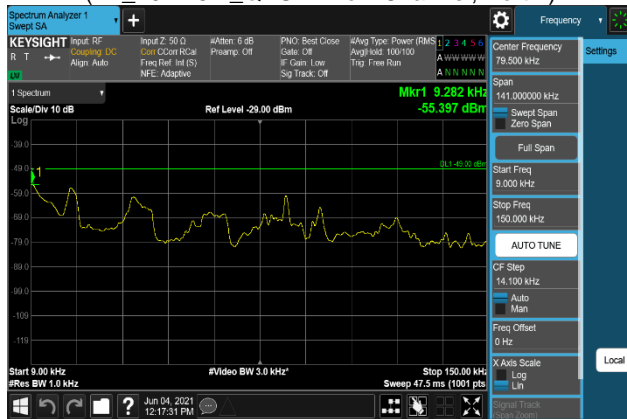
Plot 7-2191. Conducted Spurious Emission Plot 9 kHz to 150 kHz (B2_20M+5M_64QAM - Low Channel, Port 2)
