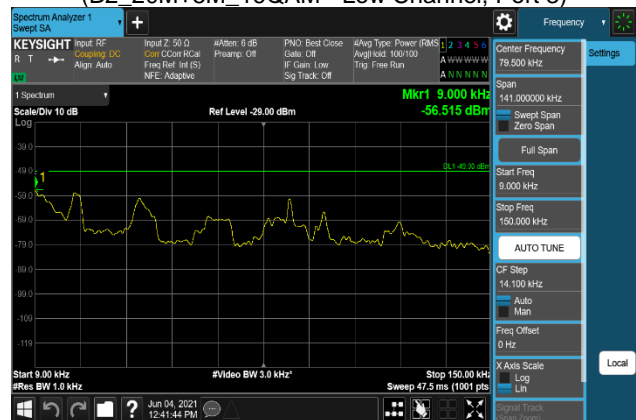
Plot 7-2220. Conducted Spurious Emission Plot 9 kHz to 150 kHz (B2_20M+5M_256QAM - Low Channel, Port 3)
