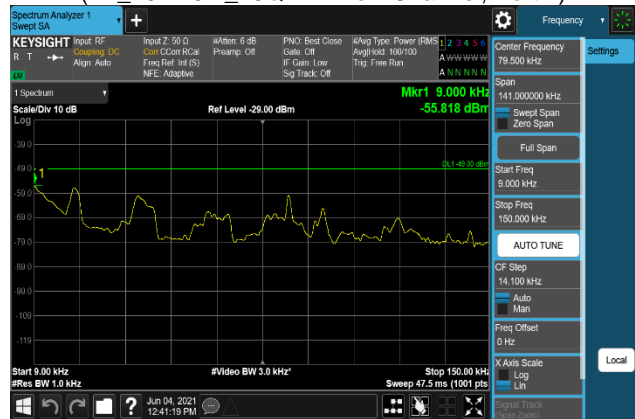
Plot 7-2192. Conducted Spurious Emission Plot 9 kHz to 150 kHz (B2_20M+5M_256QAM - Low Channel, Port 2)
