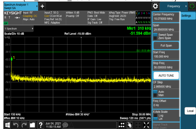
Plot 7-2222. Conducted Spurious Emission Plot 150 kHz to 30 MHz (B2_20M+5M_16QAM - Low Channel, Port 3)
