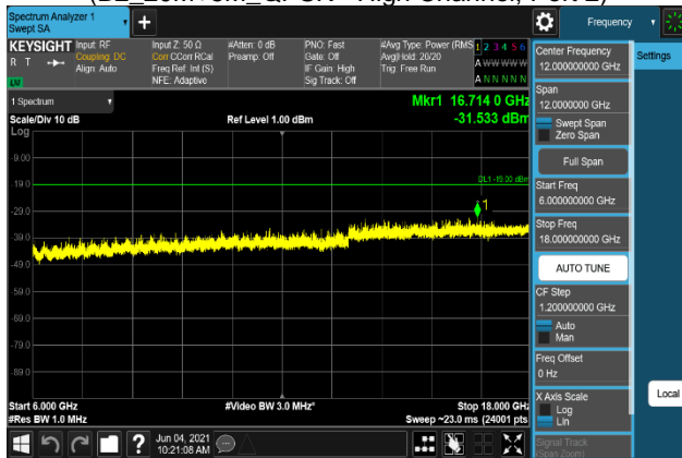
Plot 7-2099. Conducted Spurious Emission Plot 6 GHz to 18 GHz (B2_20M+5M_64QAM - High Channel, Port 2)
