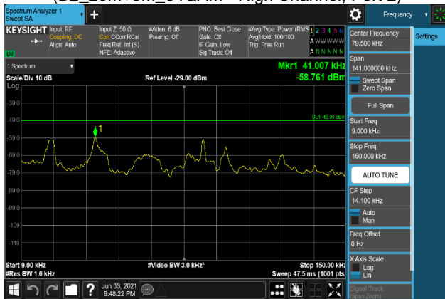
Plot 7-2105. Conducted Spurious Emission Plot 9 kHz to 150 kHz (B2_20M+5M_QPSK - High Channel, Port 3)
