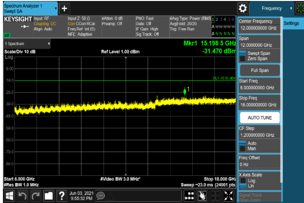
Plot 7-2097. Conducted Spurious Emission Plot 6 GHz to 18 GHz (B2_20M+5M_QPSK - High Channel, Port 2)
