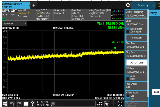
Plot 7-2153. Conducted Spurious Emission Plot 6 GHz to 18 GHz (B2_20M+5M_QPSK - Low Channel, Port 0)
