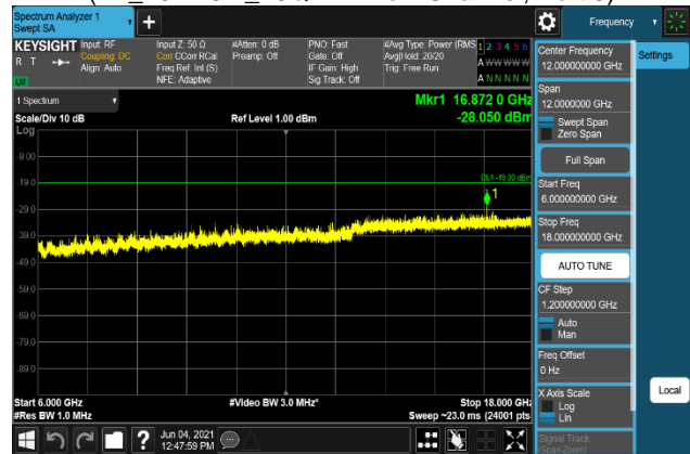
Plot 7-2156. Conducted Spurious Emission Plot 6 GHz to 18 GHz (B2_20M+5M_256QAM - Low Channel, Port 0)
