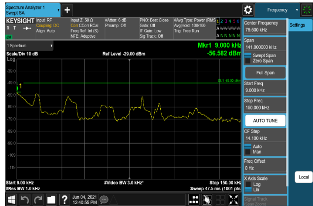
Plot 7-2164. Conducted Spurious Emission Plot 9 kHz to 150 kHz (B2_20M+5M_256QAM - Low Channel, Port 1)
