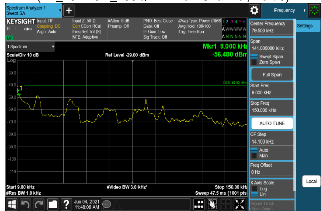
Plot 7-2162. Conducted Spurious Emission Plot 9 kHz to 150 kHz (B2_20M+5M_16QAM - Low Channel, Port 1)
