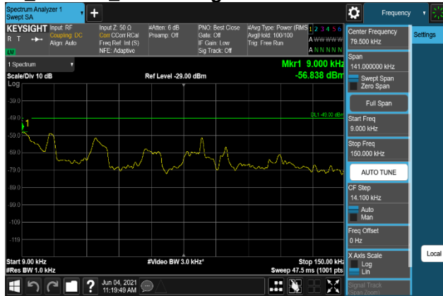
Plot 7-2133. Conducted Spurious Emission Plot 9 kHz to 150 kHz (B2_20M+5M_QPSK - Low Channel, Port 0)
