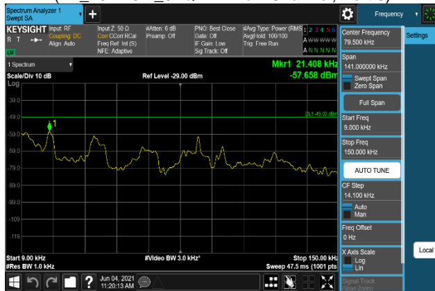
Plot 7-2161. Conducted Spurious Emission Plot 9 kHz to 150 kHz (B2_20M+5M_QPSK - Low Channel, Port 1)
