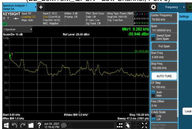
Plot 7-2135. Conducted Spurious Emission Plot 9 kHz to 150 kHz (B2_20M+5M_64QAM - Low Channel, Port 0)
