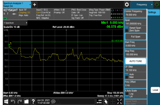
Plot 7-2134. Conducted Spurious Emission Plot 9 kHz to 150 kHz (B2_20M+5M_16QAM - Low Channel, Port 0)
