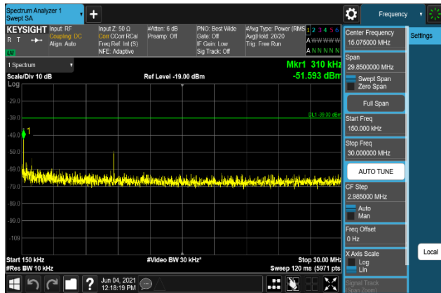
Plot 7-2139. Conducted Spurious Emission Plot 150 kHz to 30 MHz (B2_20M+5M_64QAM - Low Channel, Port 0)
