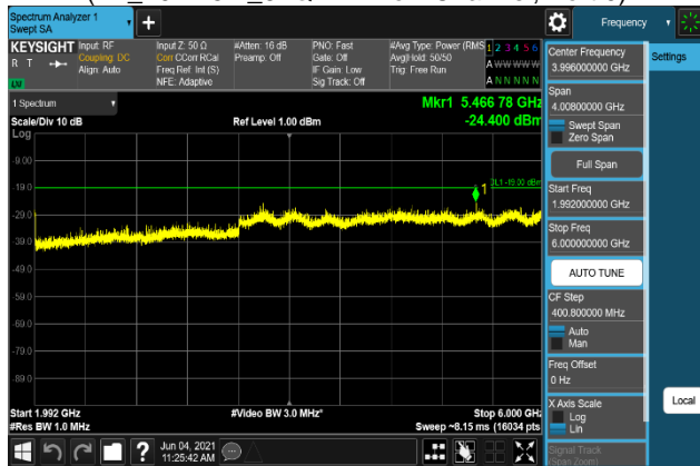
Plot 7-2149. Conducted Spurious Emission Plot 1.992 GHz to 6 GHz (B2_20M+5M_QPSK - Low Channel, Port 0)
