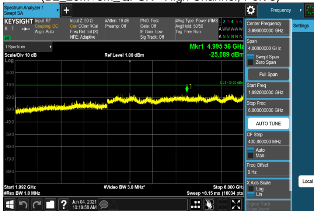
Plot 7-2123. Conducted Spurious Emission Plot 1.992 GHz to 6 GHz (B2_20M+5M_64QAM - High Channel, Port 3)
