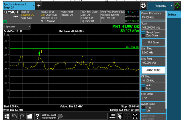
Plot 7-2106. Conducted Spurious Emission Plot 9 kHz to 150 kHz (B2_20M+5M_16QAM - High Channel, Port 3)
