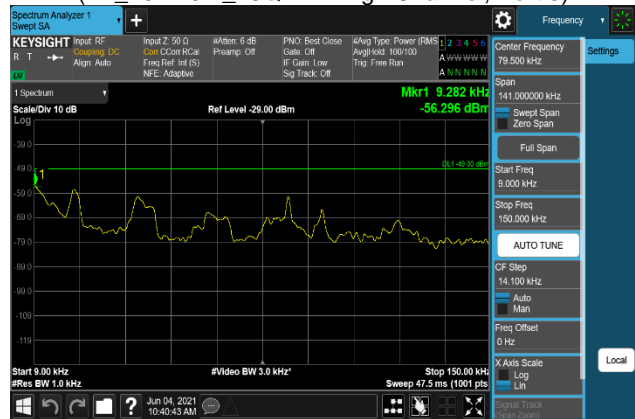
Plot 7-2108. Conducted Spurious Emission Plot 9 kHz to 150 kHz (B2_20M+5M_256QAM - High Channel, Port 3)
