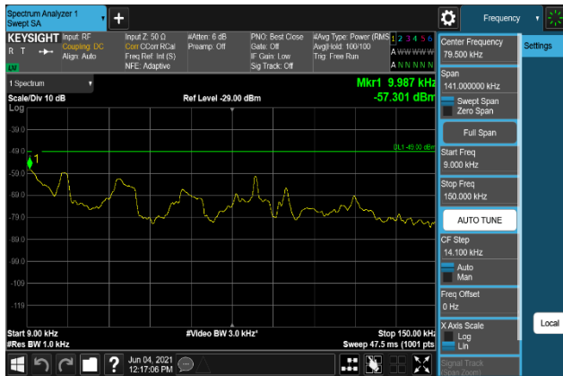
Plot 7-2163. Conducted Spurious Emission Plot 9 kHz to 150 kHz (B2_20M+5M_64QAM - Low Channel, Port 1)
