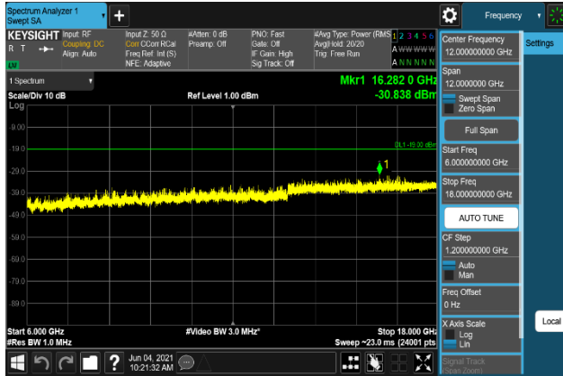
Plot 7-2127. Conducted Spurious Emission Plot 6 GHz to 18 GHz (B2_20M+5M_64QAM - High Channel, Port 3)
