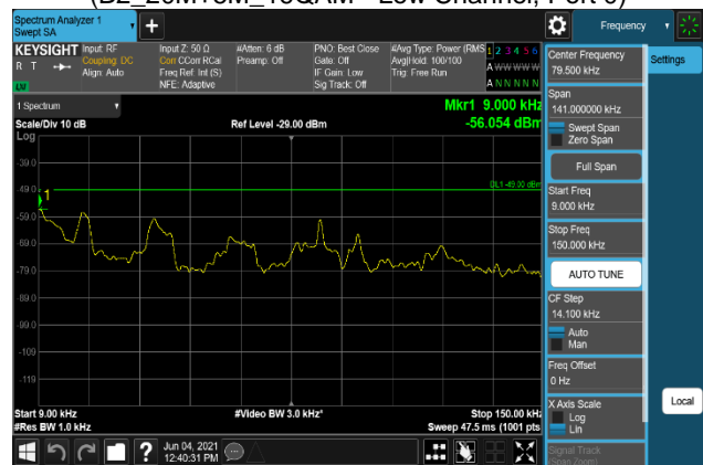
Plot 7-2136. Conducted Spurious Emission Plot 9 kHz to 150 kHz (B2_20M+5M_256QAM - Low Channel, Port 0)
