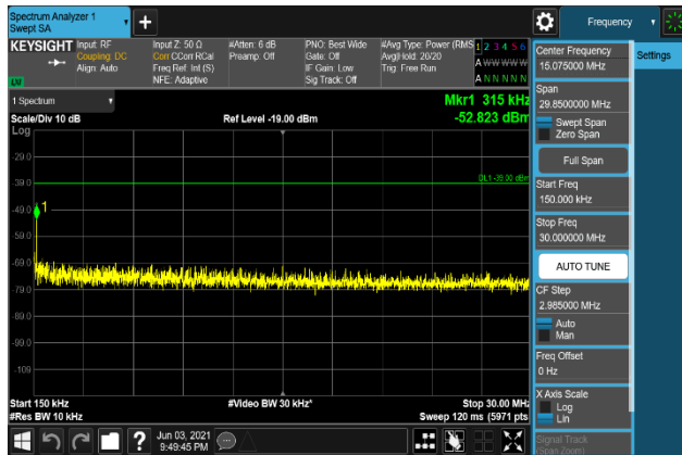
Plot 7-2109. Conducted Spurious Emission Plot 150 kHz to 30 MHz (B2_20M+5M_QPSK - High Channel, Port 3)
