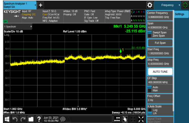
Plot 7-2122. Conducted Spurious Emission Plot 1.992 GHz to 6 GHz (B2_20M+5M_16QAM - High Channel, Port 3)
