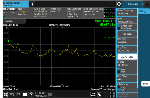
Plot 7-280. Conducted Spurious Emission Plot 9 kHz to 150 kHz (B2_20M+5M_256QAM - High Channel, Port 2)
