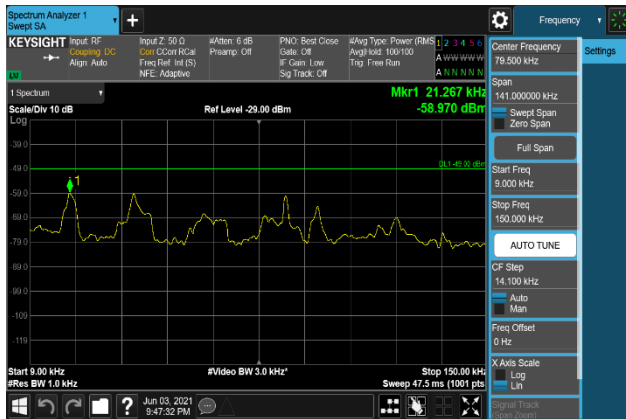
Plot 7-2049. Conducted Spurious Emission Plot 9 kHz to 150 kHz (B2_20M+5M_QPSK - High Channel, Port 1)
