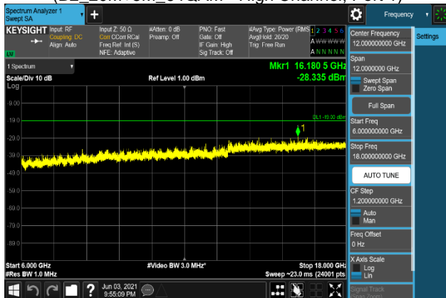
Plot 7-2069. Conducted Spurious Emission Plot 6 GHz to 18 GHz (B2_20M+5M_QPSK - High Channel, Port 1)
