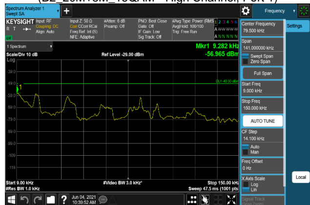
Plot 7-2052. Conducted Spurious Emission Plot 9 kHz to 150 kHz (B2_20M+5M_256QAM - High Channel, Port 1)
