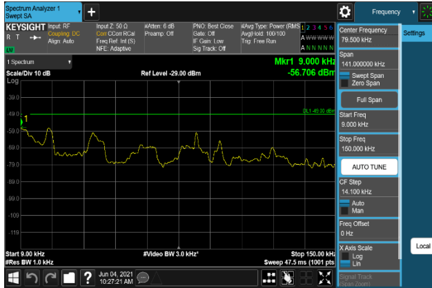
Plot 7-279. Conducted Spurious Emission Plot 9 kHz to 150 kHz (B2_20M+5M_64QAM - High Channel, Port 2)
