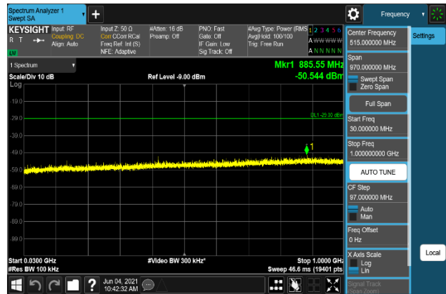
Plot 7-232. Conducted Spurious Emission Plot 30 MHz to 1 GHz (B2_20M+5M_256QAM - High Channel, Port 0)
