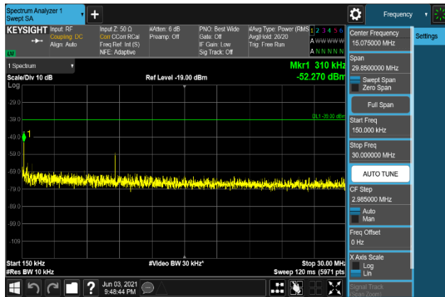
Plot 7-2025. Conducted Spurious Emission Plot 150 kHz to 30 MHz (B2_20M+5M_QPSK - High Channel, Port 0)
