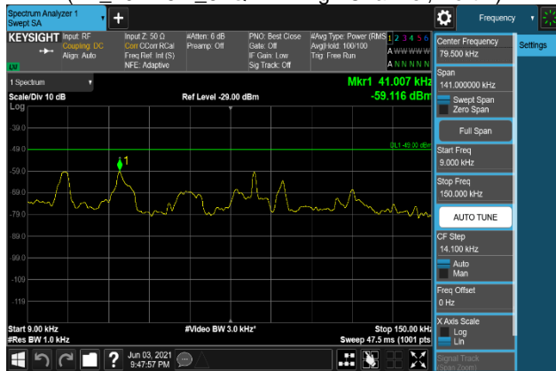
Plot 7-277. Conducted Spurious Emission Plot 9 kHz to 150 kHz (B2_20M+5M_QPSK - High Channel, Port 2)
