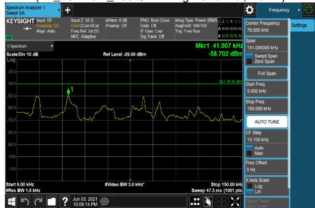
Plot 7-278. Conducted Spurious Emission Plot 9 kHz to 150 kHz (B2_20M+5M_16QAM - High Channel, Port 2)
