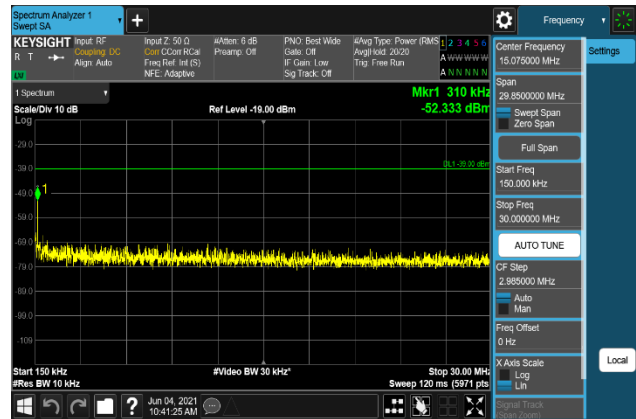
Plot 7-2056. Conducted Spurious Emission Plot 150 kHz to 30 MHz (B2_20M+5M_256QAM - High Channel, Port 1)
