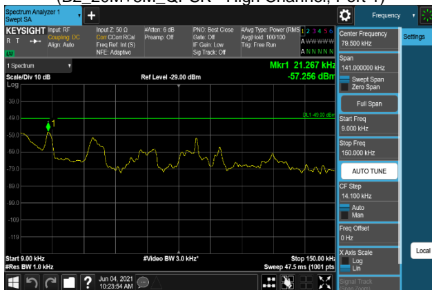
Plot 7-2051. Conducted Spurious Emission Plot 9 kHz to 150 kHz (B2_20M+5M_64QAM - High Channel, Port 1)
