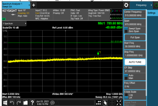
Plot 7-2029. Conducted Spurious Emission Plot 30 MHz to 1 GHz (B2_20M+5M_QPSK - High Channel, Port 0)
