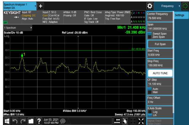
Plot 7-2050. Conducted Spurious Emission Plot 9 kHz to 150 kHz (B2_20M+5M_16QAM - High Channel, Port 1)
