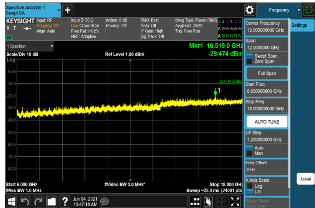
Plot 7-2044. Conducted Spurious Emission Plot 6 GHz to 18 GHz (B2_20M+5M_256QAM - High Channel, Port 0)
