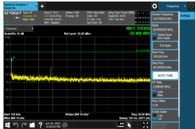
Plot 7-2026. Conducted Spurious Emission Plot 150 kHz to 30 MHz (B2_20M+5M_QPSK - High Channel, Port 0)
