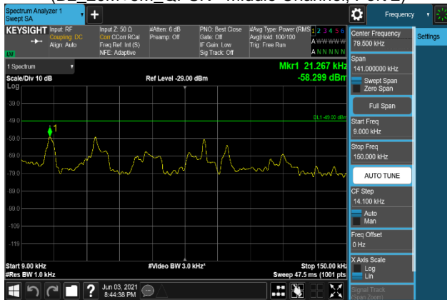
Plot 7-1967. Conducted Spurious Emission Plot 9 kHz to 150 kHz (B2_20M+5M_64QAM - Middle Channel, Port 2)
