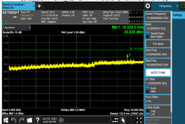
Plot 7-2015. Conducted Spurious Emission Plot 6 GHz to 18 GHz (B2_20M+5M_64QAM - Middle Channel, Port 3)
