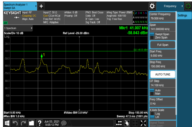
Plot 7-1996. Conducted Spurious Emission Plot 9 kHz to 150 kHz (B2_20M+5M_256QAM - Middle Channel, Port 3)
