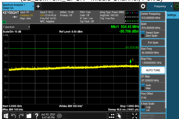
Plot 7-1975. Conducted Spurious Emission Plot 30 MHz to 1 GHz (B2_20M+5M_64QAM - Middle Channel, Port 2)
