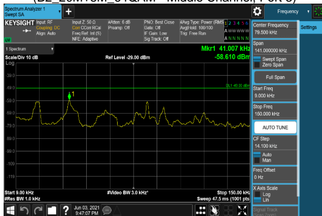
Plot 7-2021. Conducted Spurious Emission Plot 9 kHz to 150 kHz (B2_20M+5M_QPSK - High Channel, Port 0)
