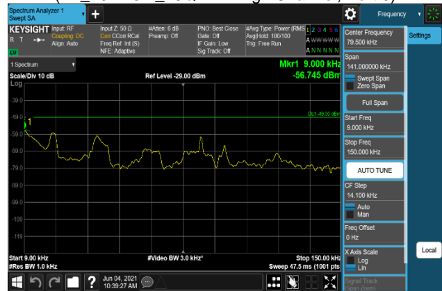
Plot 7-2024. Conducted Spurious Emission Plot 9 kHz to 150 kHz (B2_20M+5M_256QAM - High Channel, Port 0)
