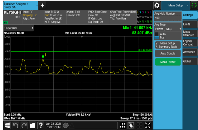
Plot 7-1966. Conducted Spurious Emission Plot 9 kHz to 150 kHz (B2_20M+5M_16QAM - Middle Channel, Port 2)
