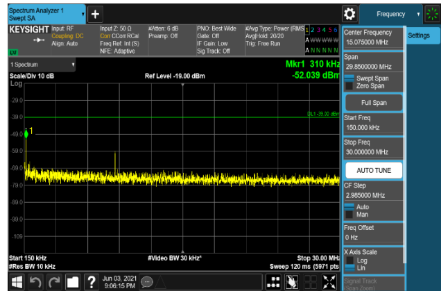
Plot 7-1972. Conducted Spurious Emission Plot 150 kHz to 30 MHz (B2_20M+5M_256QAM - Middle Channel, Port 2)
