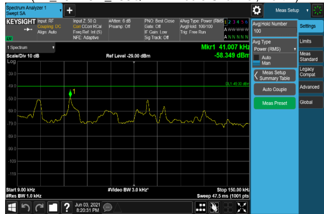
Plot 7-1994. Conducted Spurious Emission Plot 9 kHz to 150 kHz (B2_20M+5M_16QAM - Middle Channel, Port 3)
