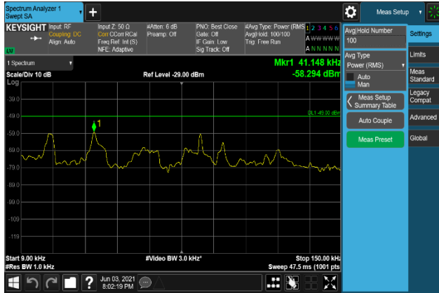
Plot 7-1965. Conducted Spurious Emission Plot 9 kHz to 150 kHz (B2_20M+5M_QPSK - Middle Channel, Port 2)
