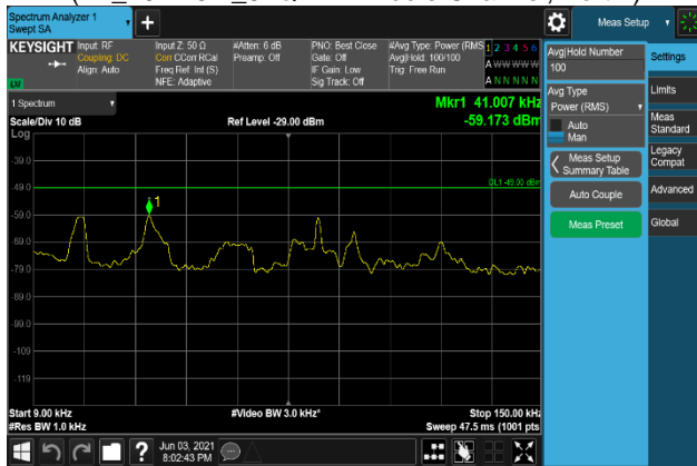
Plot 7-1993. Conducted Spurious Emission Plot 9 kHz to 150 kHz (B2_20M+5M_QPSK - Middle Channel, Port 3)
