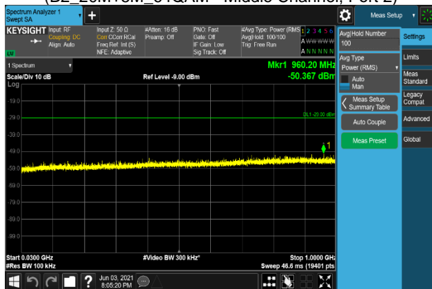
Plot 7-1973. Conducted Spurious Emission Plot 30 MHz to 1 GHz (B2_20M+5M_QPSK - Middle Channel, Port 2)
