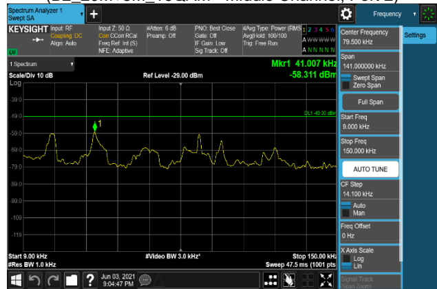
Plot 7-1968. Conducted Spurious Emission Plot 9 kHz to 150 kHz (B2_20M+5M_256QAM - Middle Channel, Port 2)
