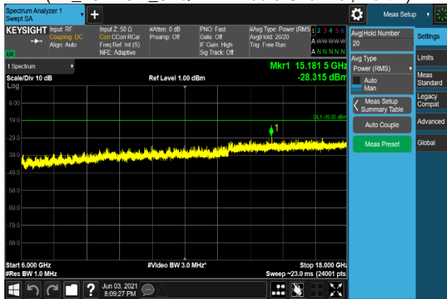
Plot 7-1957. Conducted Spurious Emission Plot 6 GHz to 18 GHz (B2_20M+5M_QPSK - Middle Channel, Port 1)
