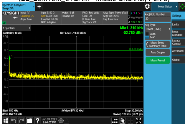
Plot 7-1997. Conducted Spurious Emission Plot 150 kHz to 30 MHz (B2_20M+5M_QPSK - Middle Channel, Port 3)
