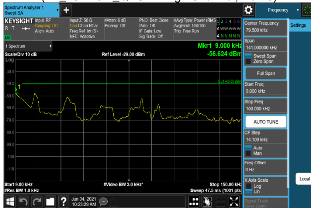
Plot 7-2023. Conducted Spurious Emission Plot 9 kHz to 150 kHz (B2_20M+5M_64QAM - High Channel, Port 0)
