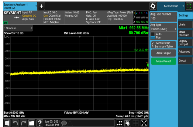
Plot 7-2002. Conducted Spurious Emission Plot 30 MHz to 1 GHz (B2_20M+5M_16QAM - Middle Channel, Port 3)
