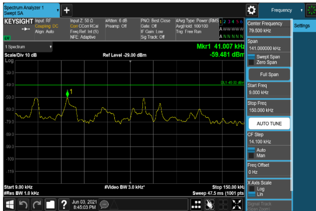
Plot 7-1995. Conducted Spurious Emission Plot 9 kHz to 150 kHz (B2_20M+5M_64QAM - Middle Channel, Port 3)
