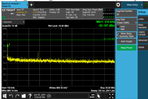
Plot 7-1969. Conducted Spurious Emission Plot 150 kHz to 30 MHz (B2_20M+5M_QPSK - Middle Channel, Port 2)
