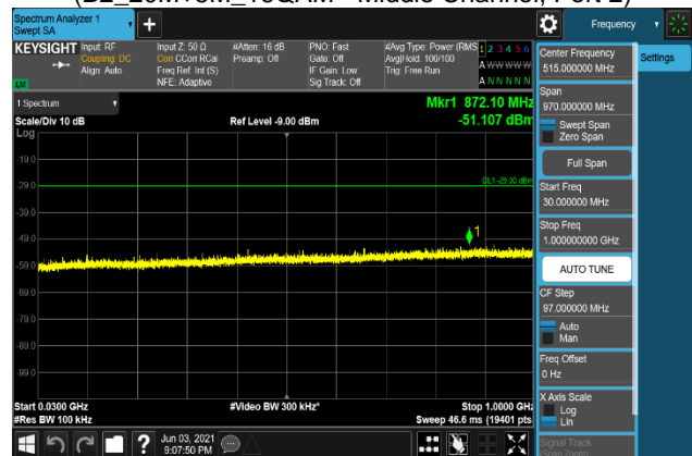
Plot 7-1976. Conducted Spurious Emission Plot 30 MHz to 1 GHz (B2_20M+5M_256QAM - Middle Channel, Port 2)
