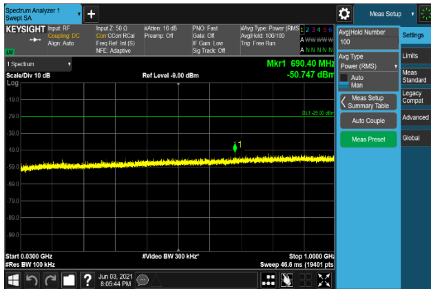
Plot 7-2001. Conducted Spurious Emission Plot 30 MHz to 1 GHz (B2_20M+5M_QPSK - Middle Channel, Port 3)
