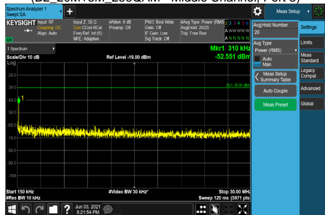
Plot 7-1998. Conducted Spurious Emission Plot 150 kHz to 30 MHz (B2_20M+5M_16QAM - Middle Channel, Port 3)
