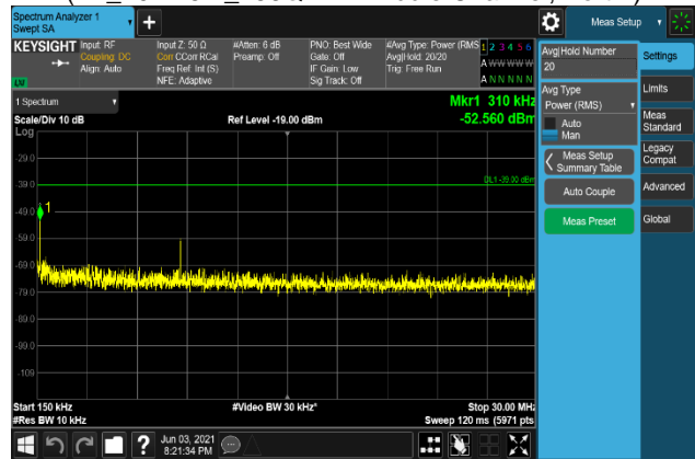
Plot 7-1970. Conducted Spurious Emission Plot 150 kHz to 30 MHz (B2_20M+5M_16QAM - Middle Channel, Port 2)
