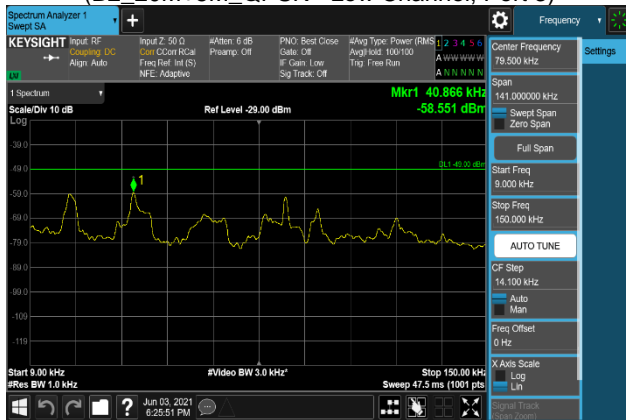
Plot 7-1883. Conducted Spurious Emission Plot 9 kHz to 150 kHz (B2_20M+5M_64QAM - Low Channel, Port 3)
