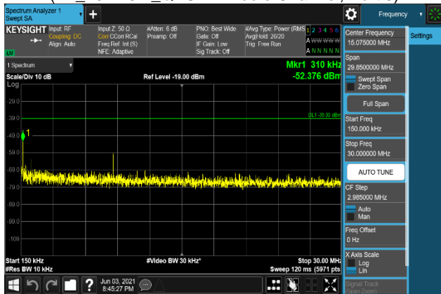
Plot 7-1915. Conducted Spurious Emission Plot 150 kHz to 30 MHz (B2_20M+5M_64QAM - Middle Channel, Port 0)
