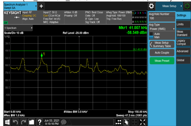
Plot 7-1910. Conducted Spurious Emission Plot 9 kHz to 150 kHz (B2_20M+5M_16QAM - Middle Channel, Port 0)
