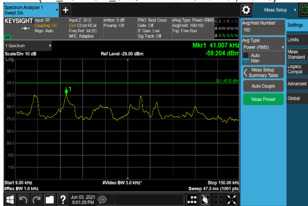
Plot 7-1909. Conducted Spurious Emission Plot 9 kHz to 150 kHz (B2_20M+5M_QPSK - Middle Channel, Port 0)
