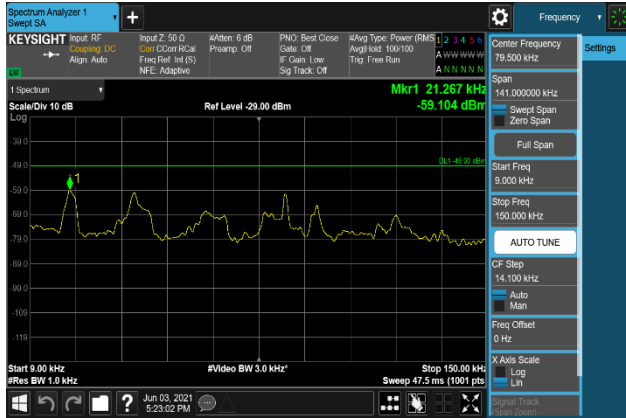
Plot 7-1881. Conducted Spurious Emission Plot 9 kHz to 150 kHz (B2_20M+5M_QPSK - Low Channel, Port 3)
