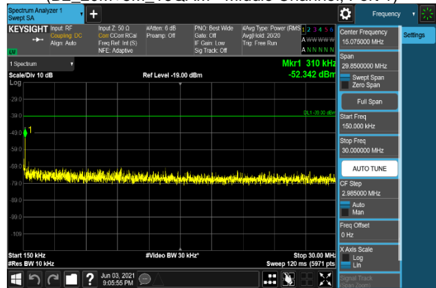
Plot 7-1944. Conducted Spurious Emission Plot 150 kHz to 30 MHz (B2_20M+5M_256QAM - Middle Channel, Port 1)
