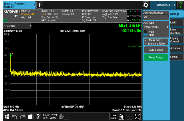
Plot 7-1942. Conducted Spurious Emission Plot 150 kHz to 30 MHz (B2_20M+5M_16QAM - Middle Channel, Port 1)
