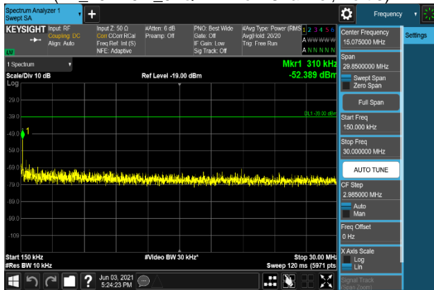
Plot 7-1885. Conducted Spurious Emission Plot 150 kHz to 30 MHz (B2_20M+5M_QPSK - Low Channel, Port 3)
