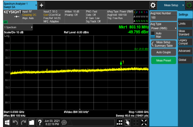
Plot 7-1918. Conducted Spurious Emission Plot 30 MHz to 1 GHz (B2_20M+5M_16QAM - Middle Channel, Port 0)
