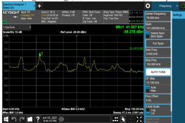
Plot 7-1939. Conducted Spurious Emission Plot 9 kHz to 150 kHz (B2_20M+5M_64QAM - Middle Channel, Port 1)
