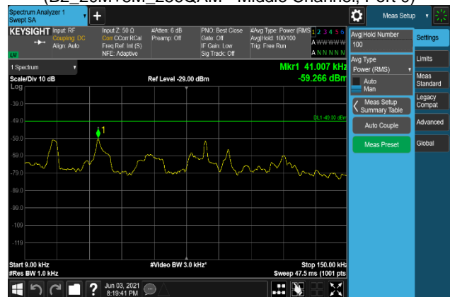
Plot 7-1938. Conducted Spurious Emission Plot 9 kHz to 150 kHz (B2_20M+5M_16QAM - Middle Channel, Port 1)
