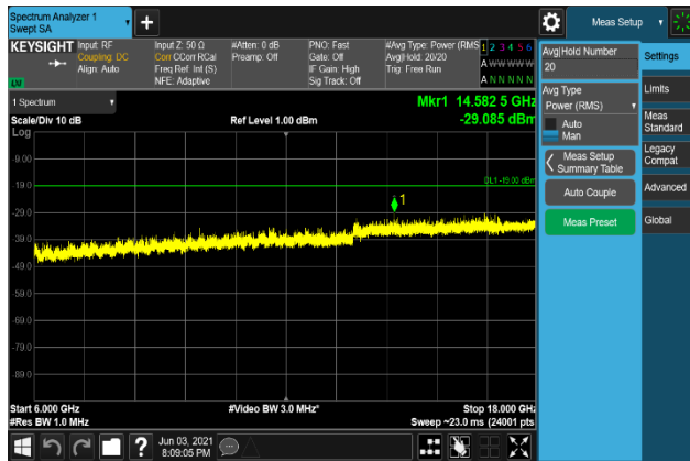
Plot 7-1929. Conducted Spurious Emission Plot 6 GHz to 18 GHz (B2_20M+5M_QPSK - Middle Channel, Port 0)
