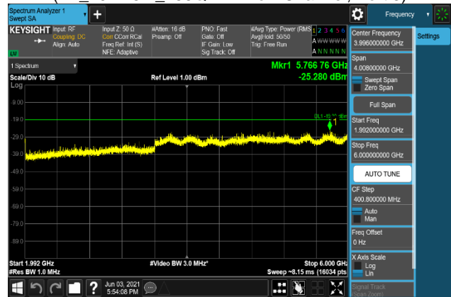
Plot 7-1898. Conducted Spurious Emission Plot 1.992 GHz to 6 GHz (B2_20M+5M_16QAM - Low Channel, Port 3)
