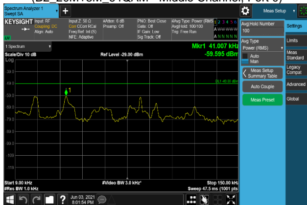
Plot 7-1937. Conducted Spurious Emission Plot 9 kHz to 150 kHz (B2_20M+5M_QPSK - Middle Channel, Port 1)
