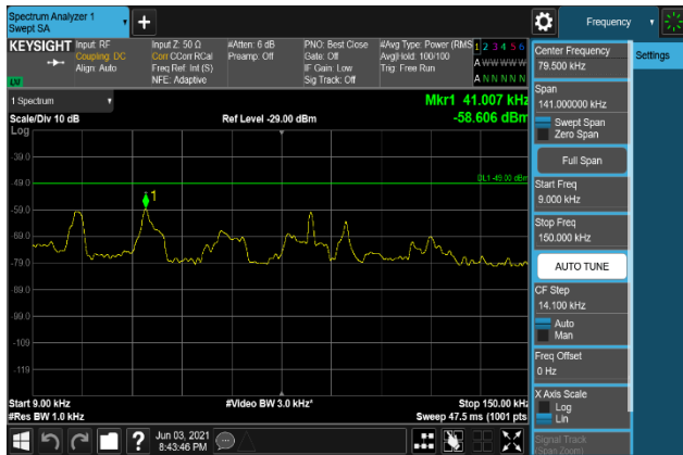
Plot 7-1911. Conducted Spurious Emission Plot 9 kHz to 150 kHz (B2_20M+5M_64QAM - Middle Channel, Port 0)
