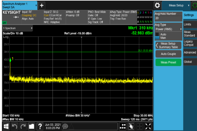
Plot 7-1941. Conducted Spurious Emission Plot 150 kHz to 30 MHz (B2_20M+5M_QPSK - Middle Channel, Port 1)
