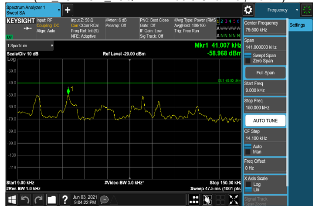
Plot 7-1940. Conducted Spurious Emission Plot 9 kHz to 150 kHz (B2_20M+5M_256QAM - Middle Channel, Port 1)
