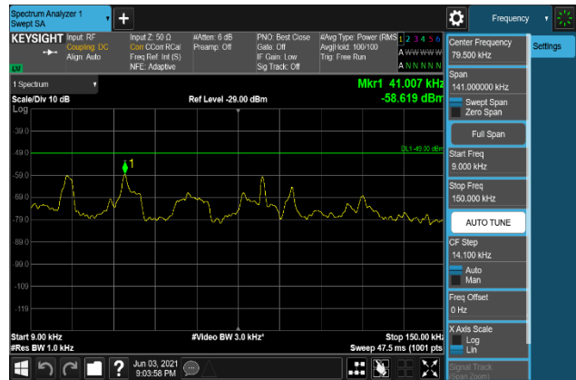
Plot 7-1912. Conducted Spurious Emission Plot 9 kHz to 150 kHz (B2_20M+5M_256QAM - Middle Channel, Port 0)
