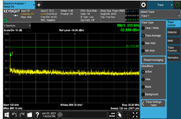
Plot 7-1888. Conducted Spurious Emission Plot 150 kHz to 30 MHz (B2_20M+5M_256QAM - Low Channel, Port 3)
