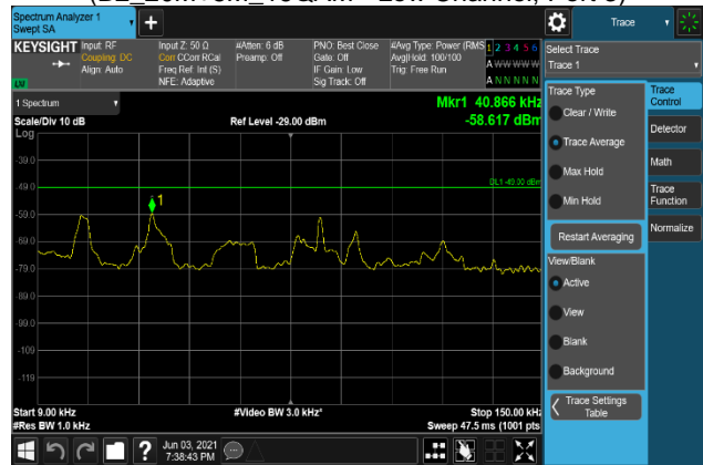
Plot 7-1884. Conducted Spurious Emission Plot 9 kHz to 150 kHz (B2_20M+5M_256QAM - Low Channel, Port 3)
