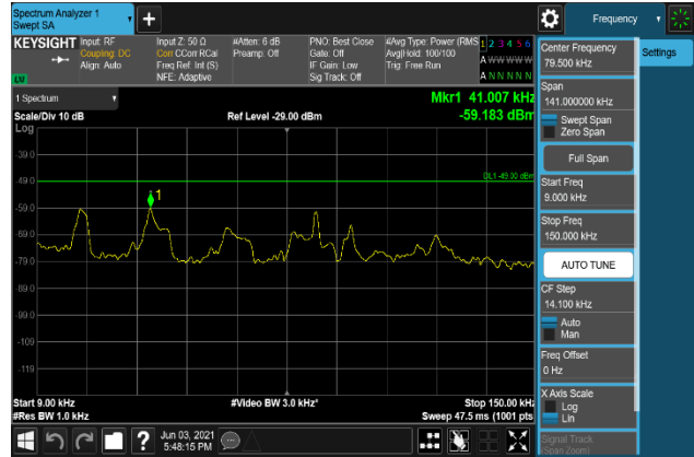
Plot 7-1882. Conducted Spurious Emission Plot 9 kHz to 150 kHz (B2_20M+5M_16QAM - Low Channel, Port 3)
