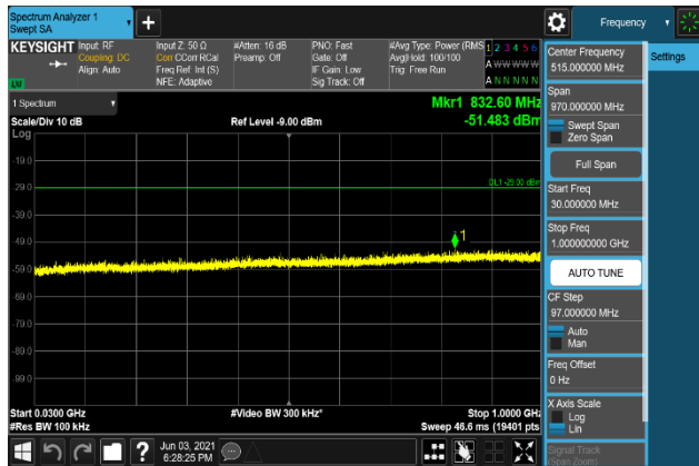
Plot 7-1863. Conducted Spurious Emission Plot 30 MHz to 1 GHz (B2_20M+5M_64QAM - Low Channel, Port 2)
