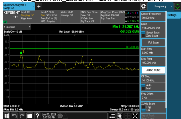
Plot 7-1854. Conducted Spurious Emission Plot 9 kHz to 150 kHz (B2_20M+5M_16QAM - Low Channel, Port 2)
