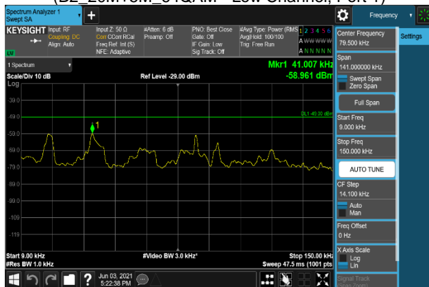
Plot 7-1853. Conducted Spurious Emission Plot 9 kHz to 150 kHz (B2_20M+5M_QPSK - Low Channel, Port 2)
