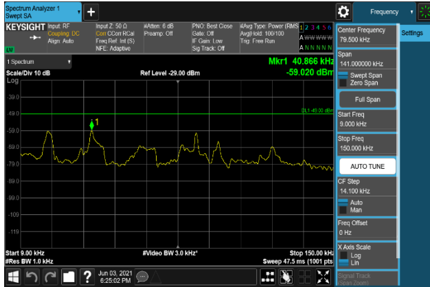
Plot 7-1827. Conducted Spurious Emission Plot 9 kHz to 150 kHz (B2_20M+5M_64QAM - Low Channel, Port 1)
