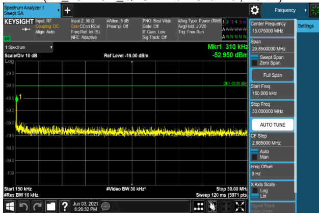
Plot 7-1831. Conducted Spurious Emission Plot 150 kHz to 30 MHz (B2_20M+5M_64QAM - Low Channel, Port 1)
