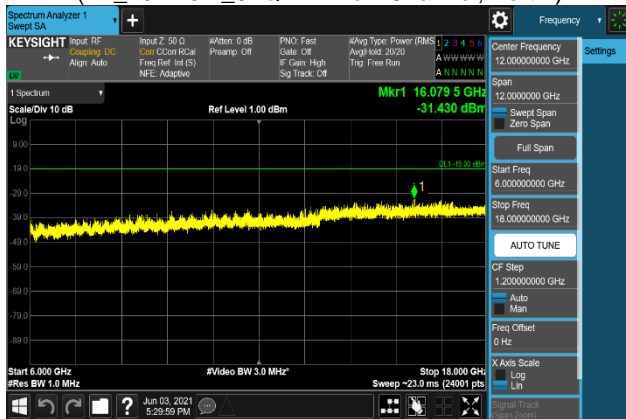
Plot 7-1873. Conducted Spurious Emission Plot 6 GHz to 18 GHz (B2_20M+5M_QPSK - Low Channel, Port 2)
