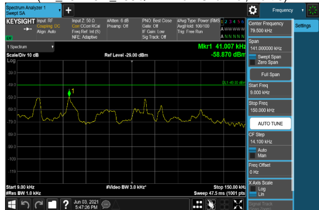
Plot 7-1826. Conducted Spurious Emission Plot 9 kHz to 150 kHz (B2_20M+5M_16QAM - Low Channel, Port 1)
