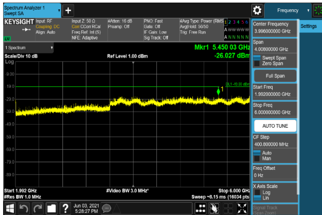
Plot 7-1869. Conducted Spurious Emission Plot 1.992 GHz to 6 GHz (B2_20M+5M_QPSK - Low Channel, Port 2)
