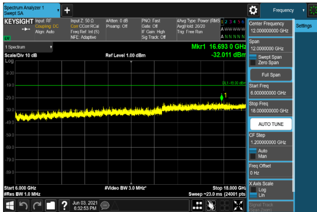
Plot 7-1875. Conducted Spurious Emission Plot 6 GHz to 18 GHz (B2_20M+5M_64QAM - Low Channel, Port 2)
