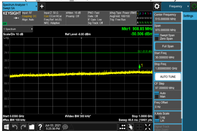
Plot 7-1861. Conducted Spurious Emission Plot 30 MHz to 1 GHz (B2_20M+5M_QPSK - Low Channel, Port 2)
