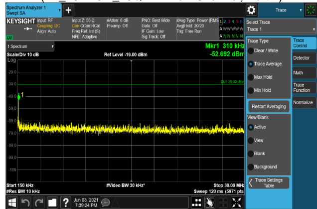
Plot 7-1832. Conducted Spurious Emission Plot 150 kHz to 30 MHz (B2_20M+5M_256QAM - Low Channel, Port 1)
