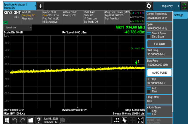
Plot 7-1834. Conducted Spurious Emission Plot 30 MHz to 1 GHz (B2_20M+5M_16QAM - Low Channel, Port 1)
