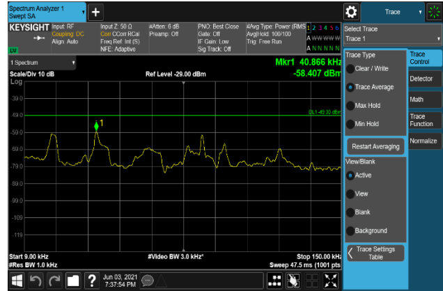
Plot 7-1828. Conducted Spurious Emission Plot 9 kHz to 150 kHz (B2_20M+5M_256QAM - Low Channel, Port 1)
