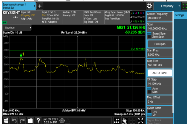
Plot 7-1825. Conducted Spurious Emission Plot 9 kHz to 150 kHz (B2_20M+5M_QPSK - Low Channel, Port 1)
