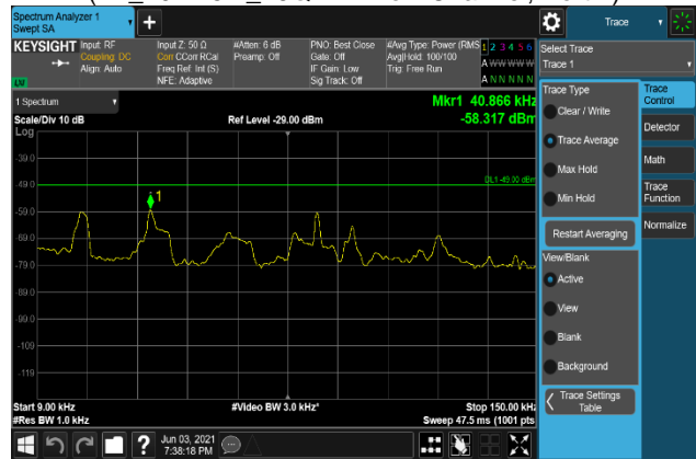
Plot 7-1856. Conducted Spurious Emission Plot 9 kHz to 150 kHz (B2_20M+5M_256QAM - Low Channel, Port 2)
