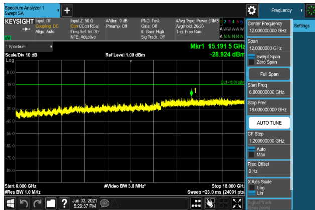
Plot 7-1845. Conducted Spurious Emission Plot 6 GHz to 18 GHz (B2_20M+5M_QPSK - Low Channel, Port 1)
