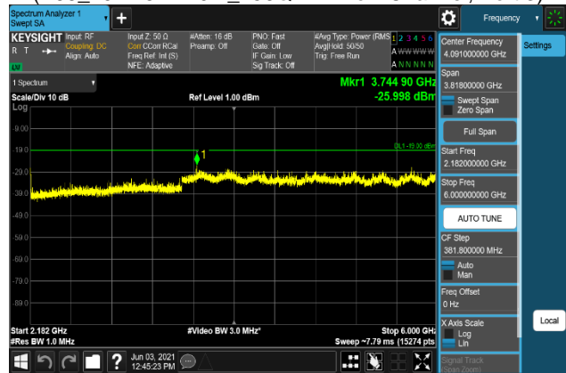
Plot 7-1786. Conducted Spurious Emission Plot 2.182 GHz to 6 GHz (B66_20M+5M+10M_16QAM - Low Channel, Port 3)
