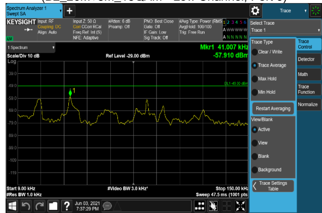
Plot 7-1800. Conducted Spurious Emission Plot 9 kHz to 150 kHz (B2_20M+5M_256QAM - Low Channel, Port 0)
