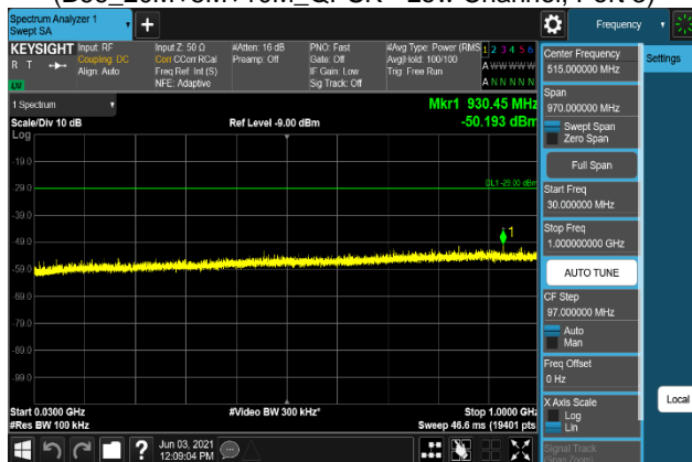
Plot 7-1779. Conducted Spurious Emission Plot 30 MHz to 1 GHz (B66_20M+5M+10M_64QAM - Low Channel, Port 3)
