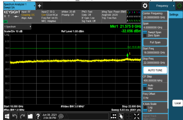
Plot 7-1768. Conducted Spurious Emission Plot 18 GHz to 22 GHz (B66_20M+5M+10M_256QAM - Low Channel, Port 2)
