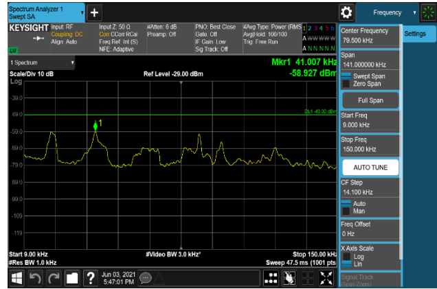
Plot 7-1798. Conducted Spurious Emission Plot 9 kHz to 150 kHz (B2_20M+5M_16QAM - Low Channel, Port 0)
