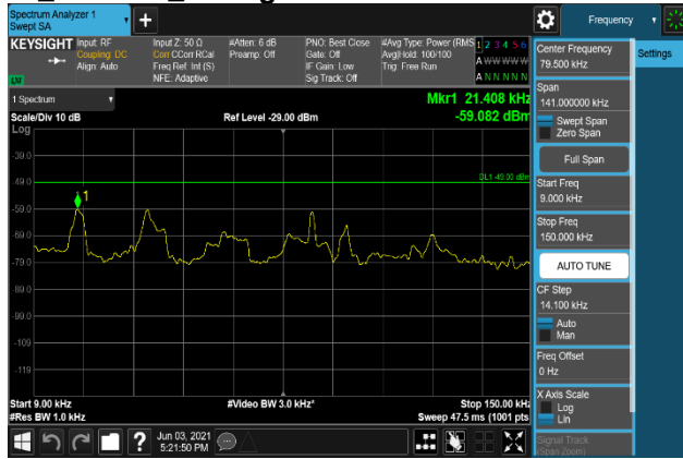
Plot 7-1797. Conducted Spurious Emission Plot 9 kHz to 150 kHz (B2_20M+5M_QPSK - Low Channel, Port 0)
