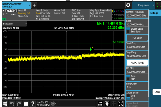
Plot 7-1761. Conducted Spurious Emission Plot 6 GHz to 18 GHz (B66_20M+5M+10M_QPSK - Low Channel, Port 2)
