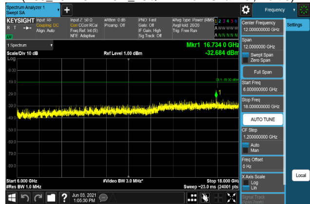
Plot 7-1792. Conducted Spurious Emission Plot 6 GHz to 18 GHz (B66_20M+5M+10M_256QAM - Low Channel, Port 3)
