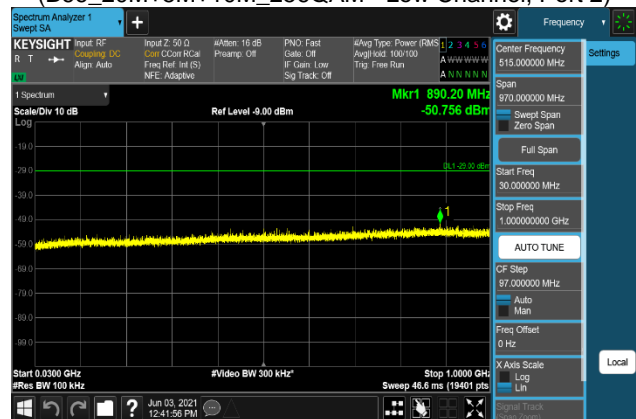
Plot 7-1750. Conducted Spurious Emission Plot 30 MHz to 1 GHz (B66_20M+5M+10M_16QAM - Low Channel, Port 2)
