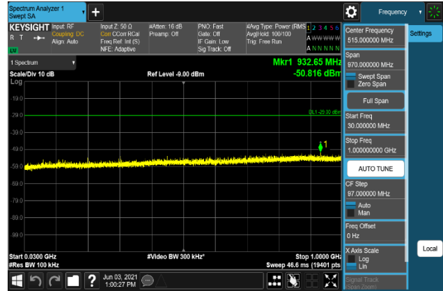
Plot 7-1752. Conducted Spurious Emission Plot 30 MHz to 1 GHz (B66_20M+5M+10M_256QAM - Low Channel, Port 2)
