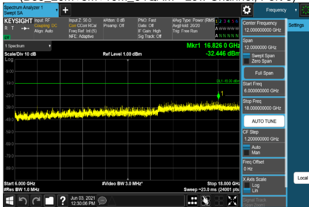
Plot 7-1789. Conducted Spurious Emission Plot 6 GHz to 18 GHz (B66_20M+5M+10M_QPSK - Low Channel, Port 3)
