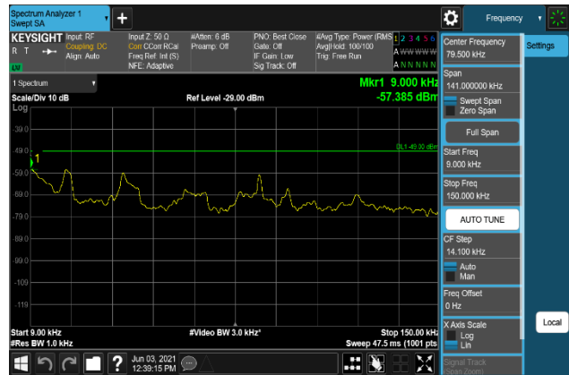
Plot 7-1770. Conducted Spurious Emission Plot 9 kHz to 150 kHz (B66_20M+5M+10M_16QAM - Low Channel, Port 3)
