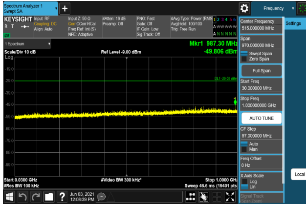
Plot 7-1751. Conducted Spurious Emission Plot 30 MHz to 1 GHz (B66_20M+5M+10M_64QAM - Low Channel, Port 2)
