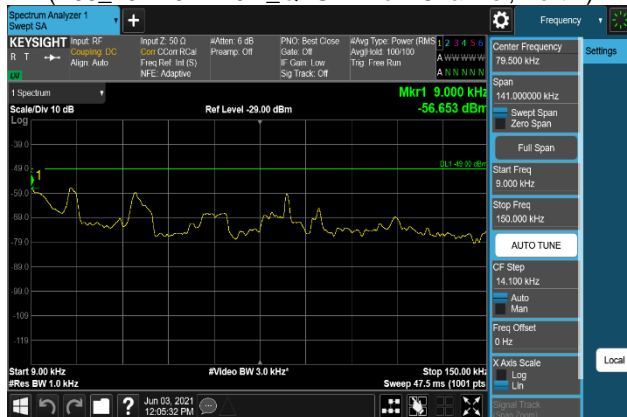
Plot 7-1743. Conducted Spurious Emission Plot 9 kHz to 150 kHz (B66_20M+5M+10M_64QAM - Low Channel, Port 2)
