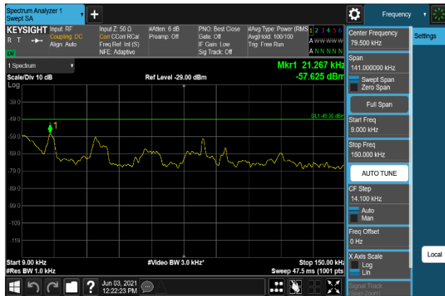
Plot 7-1769. Conducted Spurious Emission Plot 9 kHz to 150 kHz (B66_20M+5M+10M_QPSK - Low Channel, Port 3)
