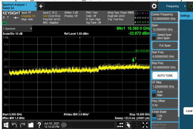
Plot 7-1791. Conducted Spurious Emission Plot 6 GHz to 18 GHz (B66_20M+5M+10M_64QAM - Low Channel, Port 3)
