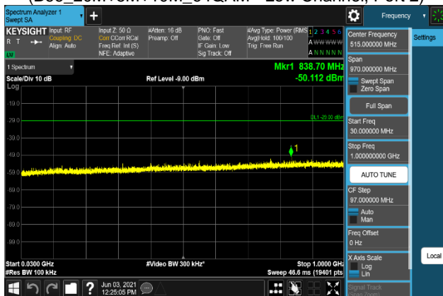
Plot 7-1749. Conducted Spurious Emission Plot 30 MHz to 1 GHz (B66_20M+5M+10M_QPSK - Low Channel, Port 2)
