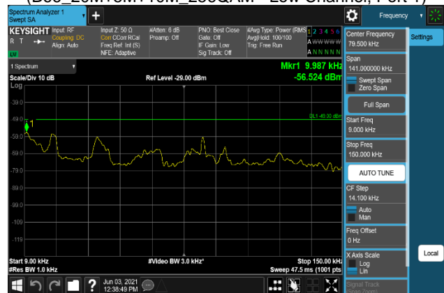
Plot 7-1742. Conducted Spurious Emission Plot 9 kHz to 150 kHz (B66_20M+5M+10M_16QAM - Low Channel, Port 2)
