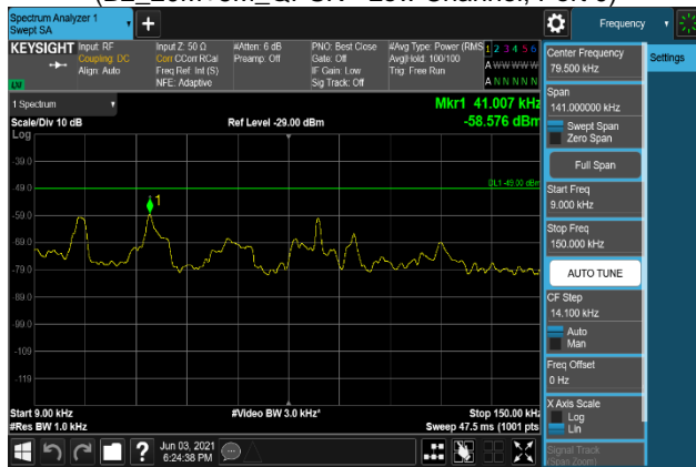
Plot 7-1799. Conducted Spurious Emission Plot 9 kHz to 150 kHz (B2_20M+5M_64QAM - Low Channel, Port 0)
