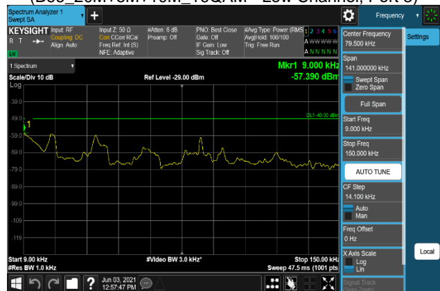
Plot 7-1772. Conducted Spurious Emission Plot 9 kHz to 150 kHz (B66_20M+5M+10M_256QAM - Low Channel, Port 3)
