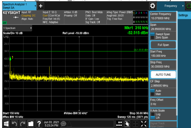
Plot 7-1801. Conducted Spurious Emission Plot 150 kHz to 30 MHz (B2_20M+5M_QPSK - Low Channel, Port 0)
