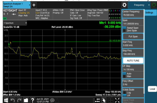
Plot 7-1744. Conducted Spurious Emission Plot 9 kHz to 150 kHz (B66_20M+5M+10M_256QAM - Low Channel, Port 2)
