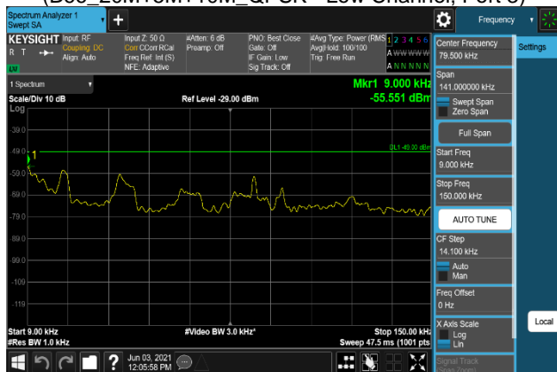
Plot 7-1771. Conducted Spurious Emission Plot 9 kHz to 150 kHz (B66_20M+5M+10M_64QAM - Low Channel, Port 3)
