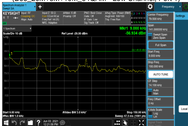
Plot 7-1741. Conducted Spurious Emission Plot 9 kHz to 150 kHz (B66_20M+5M+10M_QPSK - Low Channel, Port 2)
