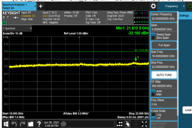
Plot 7-1765. Conducted Spurious Emission Plot 18 GHz to 22 GHz (B66_20M+5M+10M_QPSK - Low Channel, Port 2)
