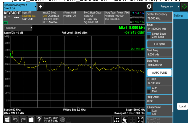
Plot 7-1714. Conducted Spurious Emission Plot 9 kHz to 150 kHz (B66_20M+5M+10M_16QAM - Low Channel, Port 1)
