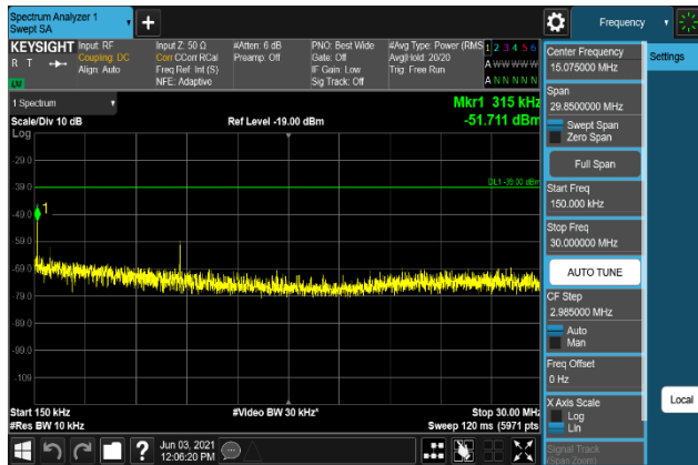
Plot 7-1691. Conducted Spurious Emission Plot 150 kHz to 30 MHz (B66_20M+5M+10M_64QAM - Low Channel, Port 0)
