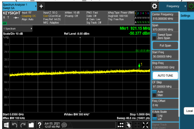
Plot 7-1695. Conducted Spurious Emission Plot 30 MHz to 1 GHz (B66_20M+5M+10M_64QAM - Low Channel, Port 0)
