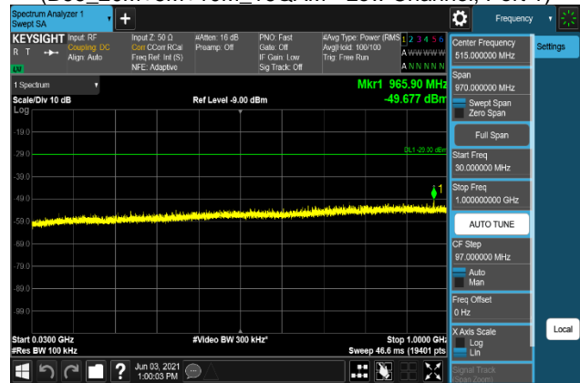
Plot 7-1724. Conducted Spurious Emission Plot 30 MHz to 1 GHz (B66_20M+5M+10M_256QAM - Low Channel, Port 1)
