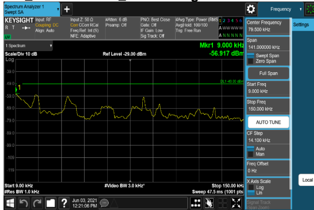
Plot 7-1685. Conducted Spurious Emission Plot 9 kHz to 150 kHz (B66_20M+5M+10M_QPSK - Low Channel, Port 0)
