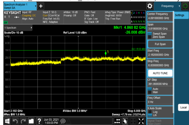
Plot 7-1732. Conducted Spurious Emission Plot 2.182 GHz to 6 GHz (B66_20M+5M+10M_256QAM - Low Channel, Port 1)
