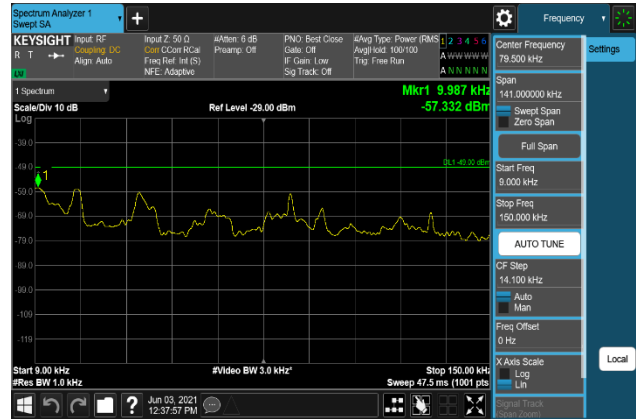
Plot 7-1686. Conducted Spurious Emission Plot 9 kHz to 150 kHz (B66_20M+5M+10M_16QAM - Low Channel, Port 0)
