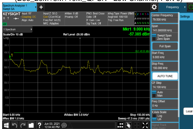
Plot 7-1687. Conducted Spurious Emission Plot 9 kHz to 150 kHz (B66_20M+5M+10M_64QAM - Low Channel, Port 0)
