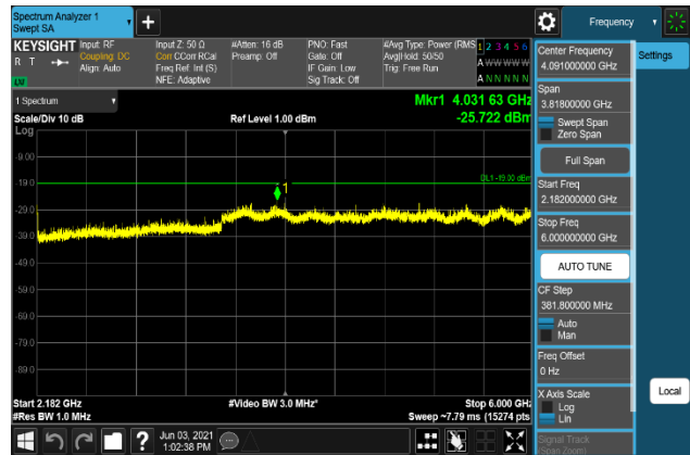
Plot 7-1704. Conducted Spurious Emission Plot 2.182 GHz to 6 GHz (B66_20M+5M+10M_256QAM - Low Channel, Port 0)
