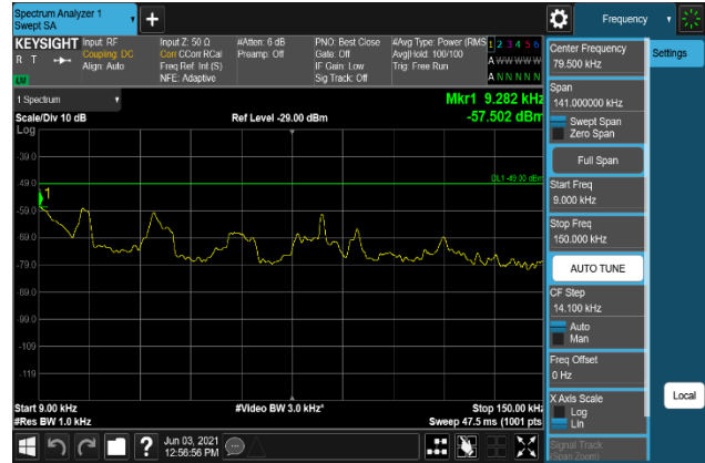
Plot 7-1716. Conducted Spurious Emission Plot 9 kHz to 150 kHz (B66_20M+5M+10M_256QAM - Low Channel, Port 1)
