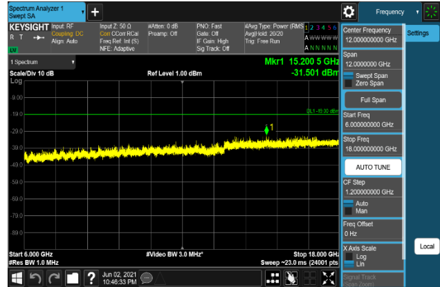
Plot 7-1680. Conducted Spurious Emission Plot 6 GHz to 18 GHz (B66_20M+5M+10M_256QAM - High Channel, Port 3)
