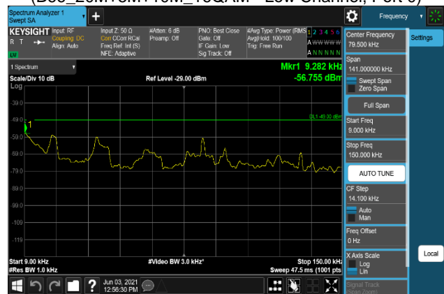
Plot 7-1688. Conducted Spurious Emission Plot 9 kHz to 150 kHz (B66_20M+5M+10M_256QAM - Low Channel, Port 0)
