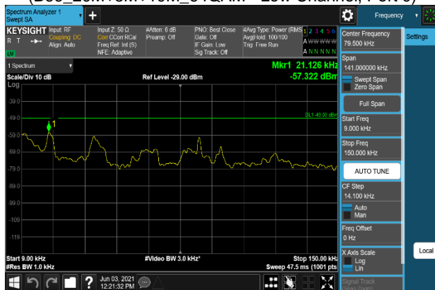
Plot 7-1713. Conducted Spurious Emission Plot 9 kHz to 150 kHz (B66_20M+5M+10M_QPSK - Low Channel, Port 1)
