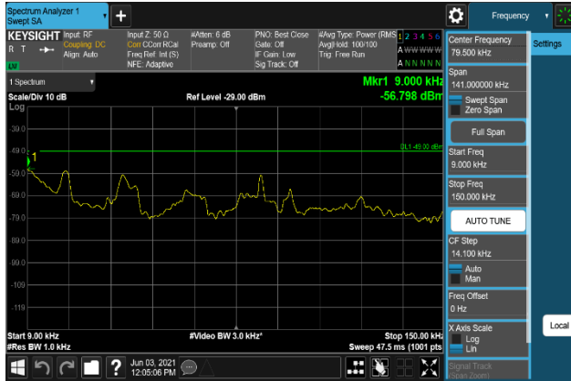
Plot 7-1715. Conducted Spurious Emission Plot 9 kHz to 150 kHz (B66_20M+5M+10M_64QAM - Low Channel, Port 1)
