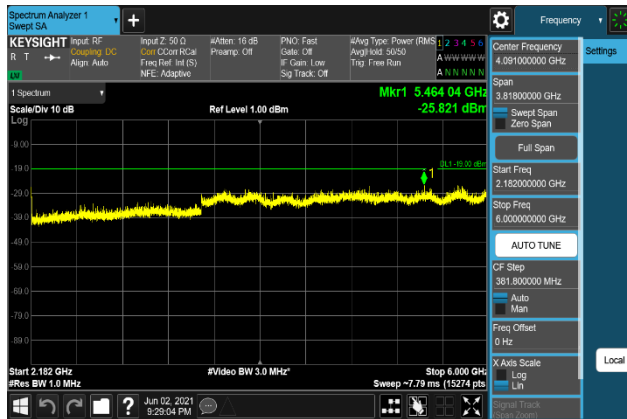
Plot 7-1673. Conducted Spurious Emission Plot 2.182 GHz to 6 GHz (B66_20M+5M+10M_QPSK - High Channel, Port 3)
