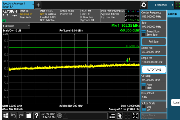
Plot 7-1721. Conducted Spurious Emission Plot 30 MHz to 1 GHz (B66_20M+5M+10M_QPSK - Low Channel, Port 1)
