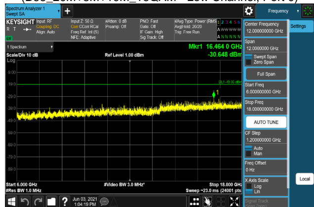
Plot 7-1708. Conducted Spurious Emission Plot 6 GHz to 18 GHz (B66_20M+5M_256QAM - Low Channel, Port 0)
