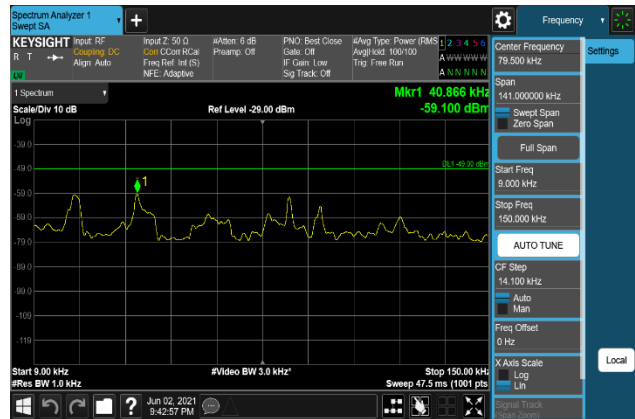
Plot 7-1602. Conducted Spurious Emission Plot 9 kHz to 150 kHz (B66_20M+5M+10M_16QAM - High Channel, Port 1)
