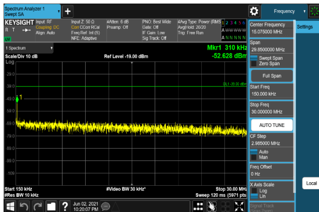
Plot 7-1607. Conducted Spurious Emission Plot 150 kHz to 30 MHz (B66_20M+5M+10M_64QAM - High Channel, Port 1)
