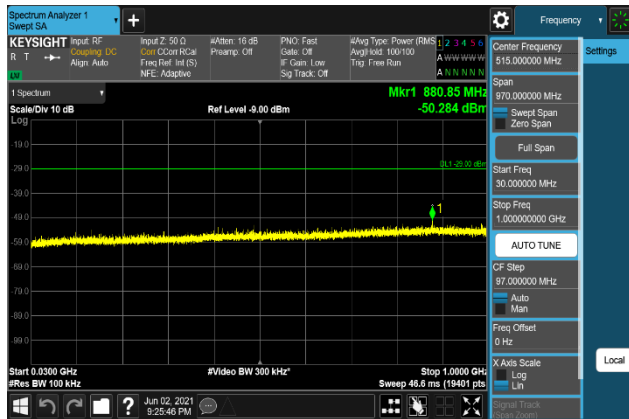
Plot 7-1637. Conducted Spurious Emission Plot 30 MHz to 1 GHz (B66_20M+5M+10M_QPSK - High Channel, Port 2)
