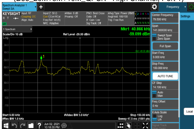
Plot 7-1603. Conducted Spurious Emission Plot 9 kHz to 150 kHz (B66_20M+5M+10M_64QAM - High Channel, Port 1)
