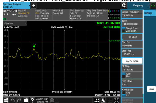
Plot 7-1658. Conducted Spurious Emission Plot 9 kHz to 150 kHz (B66_20M+5M+10M_256QAM - High Channel, Port 3)
