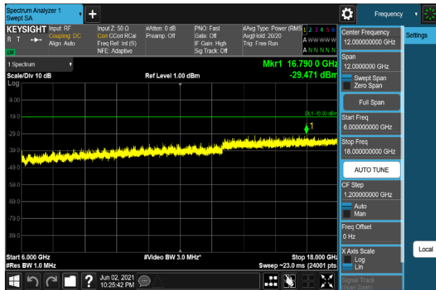
Plot 7-1595. Conducted Spurious Emission Plot 6 GHz to 18 GHz (B66_20M+5M+10M_64QAM - High Channel, Port 0)
