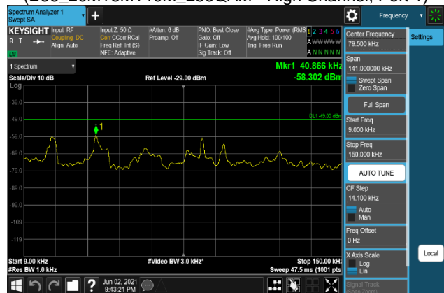
Plot 7-1630. Conducted Spurious Emission Plot 9 kHz to 150 kHz (B66_20M+5M+10M_16QAM - High Channel, Port 2)
