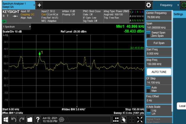
Plot 7-1631. Conducted Spurious Emission Plot 9 kHz to 150 kHz (B66_20M+5M+10M_64QAM - High Channel, Port 2)
