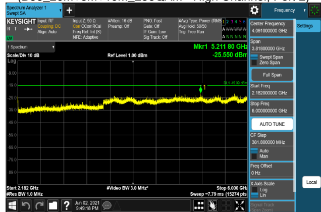
Plot 7-1646. Conducted Spurious Emission Plot 2.182 GHz to 6 GHz (B66_20M+5M+10M_16QAM - High Channel, Port 2)
