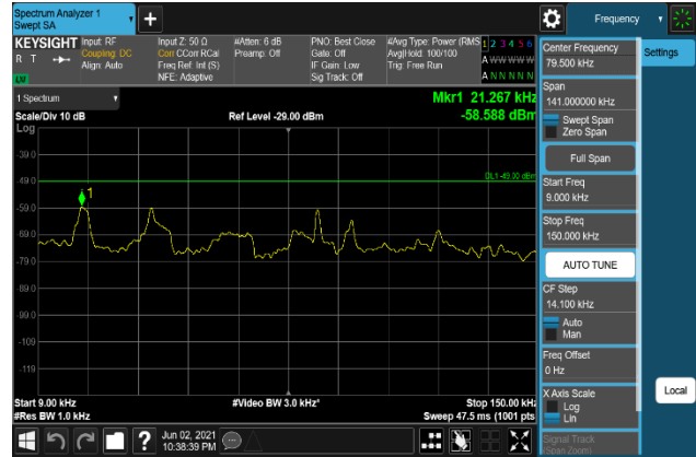
Plot 7-1632. Conducted Spurious Emission Plot 9 kHz to 150 kHz (B66_20M+5M+10M_256QAM - High Channel, Port 2)
