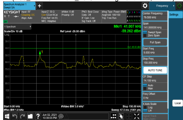
Plot 7-1660. Conducted Spurious Emission Plot 9 kHz to 150 kHz (B66_20M+5M+10M_256QAM - High Channel, Port 3)
