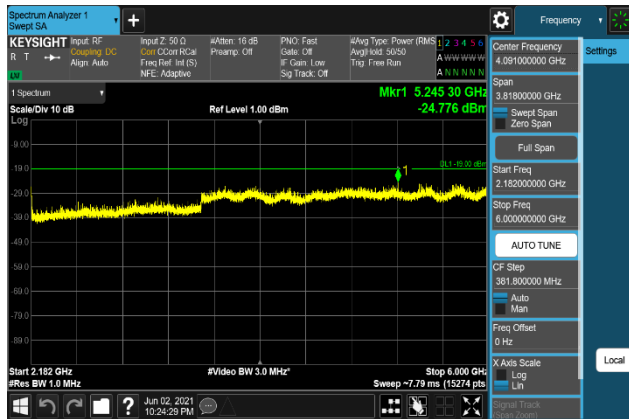
Plot 7-1619. Conducted Spurious Emission Plot 2.182 GHz to 6 GHz (B66_20M+5M+10M_64QAM - High Channel, Port 1)
