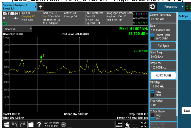
Plot 7-1657. Conducted Spurious Emission Plot 9 kHz to 150 kHz (B66_20M+5M+10M_QPSK - High Channel, Port 3)
