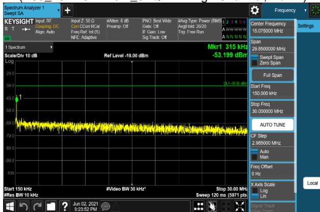
Plot 7-1605. Conducted Spurious Emission Plot 150 kHz to 30 MHz (B66_20M+5M+10M_QPSK - High Channel, Port 1)
