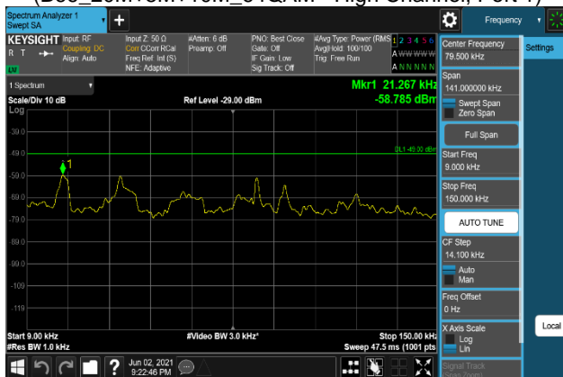
Plot 7-1629. Conducted Spurious Emission Plot 9 kHz to 150 kHz (B66_20M+5M+10M_QPSK - High Channel, Port 2)
