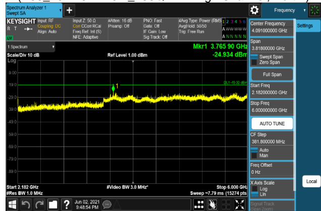
Plot 7-1618. Conducted Spurious Emission Plot 2.182 GHz to 6 GHz (B66_20M+5M+10M_16QAM - High Channel, Port 1)
