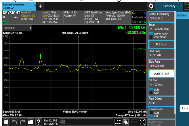
Plot 7-1659. Conducted Spurious Emission Plot 9 kHz to 150 kHz (B66_20M+5M+10M_64QAM - High Channel, Port 3)
