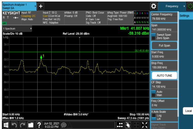
Plot 7-1601. Conducted Spurious Emission Plot 9 kHz to 150 kHz (B66_20M+5M+10M_QPSK - High Channel, Port 1)
