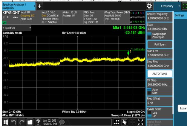
Plot 7-1645. Conducted Spurious Emission Plot 2.182 GHz to 6 GHz (B66_20M+5M+10M_QPSK - High Channel, Port 2)
