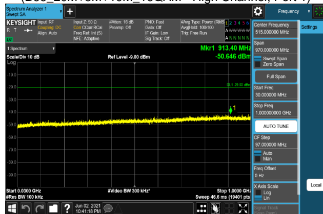
Plot 7-1612. Conducted Spurious Emission Plot 30 MHz to 1 GHz (B66_20M+5M+10M_256QAM - High Channel, Port 1)
