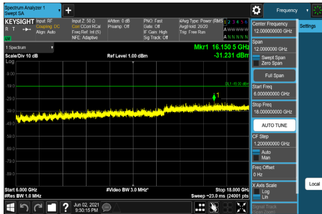
Plot 7-1649. Conducted Spurious Emission Plot 6 GHz to 18 GHz (B66_20M+5M+10M_QPSK - High Channel, Port 2)
