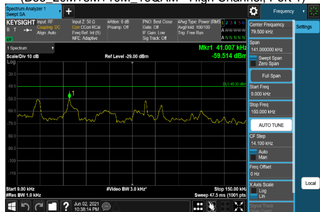
Plot 7-1604. Conducted Spurious Emission Plot 9 kHz to 150 kHz (B66_20M+5M+10M_256QAM - High Channel, Port 1)
