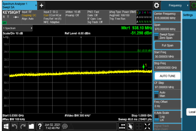
Plot 7-1553. Conducted Spurious Emission Plot 30 MHz to 1 GHz (B66_20M+5M+10M_QPSK - Middle Channel, Port 3)
