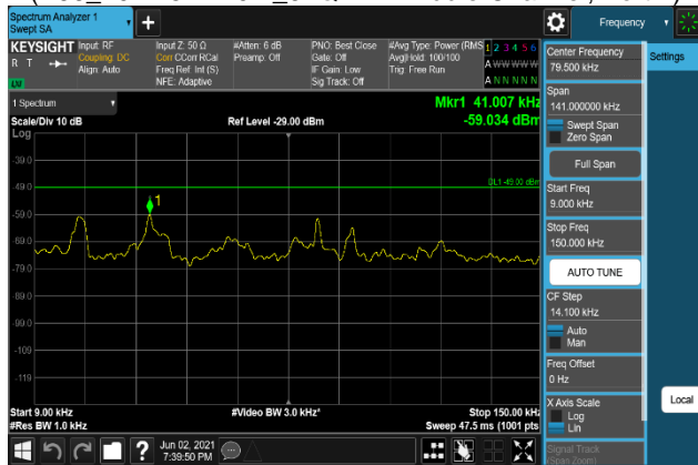
Plot 7-1545. Conducted Spurious Emission Plot 9 kHz to 150 kHz (B66_20M+5M+10M_QPSK - Middle Channel, Port 3)
