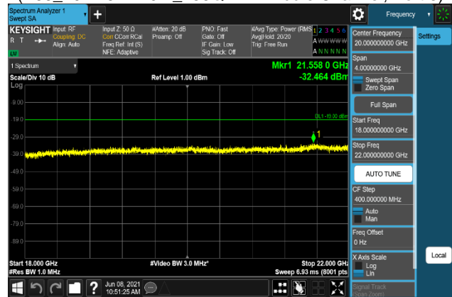
Plot 7-1570. Conducted Spurious Emission Plot 18 GHz to 22 GHz (B66_20M+5M+10M_16QAM - Middle Channel, Port 3)
