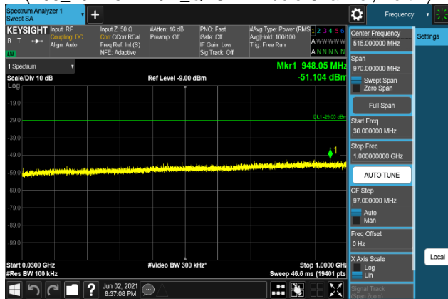
Plot 7-1527. Conducted Spurious Emission Plot 30 MHz to 1 GHz (B66_20M+5M+10M_64QAM - Middle Channel, Port 2)
