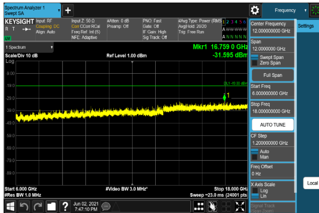
Plot 7-1565. Conducted Spurious Emission Plot 6 GHz to 18 GHz (B66_20M+5M+10M_QPSK - Middle Channel, Port 3)
