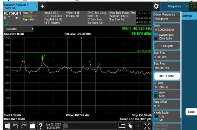
Plot 7-1546. Conducted Spurious Emission Plot 9 kHz to 150 kHz (B66_20M+5M+10M_16QAM - Middle Channel, Port 3)
