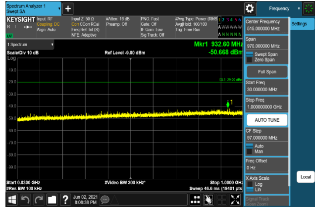
Plot 7-1554. Conducted Spurious Emission Plot 30 MHz to 1 GHz (B66_20M+5M+10M_16QAM - Middle Channel, Port 3)
