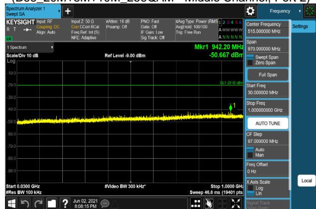
Plot 7-1526. Conducted Spurious Emission Plot 30 MHz to 1 GHz (B66_20M+5M+10M_256QAM - Middle Channel, Port 2)
