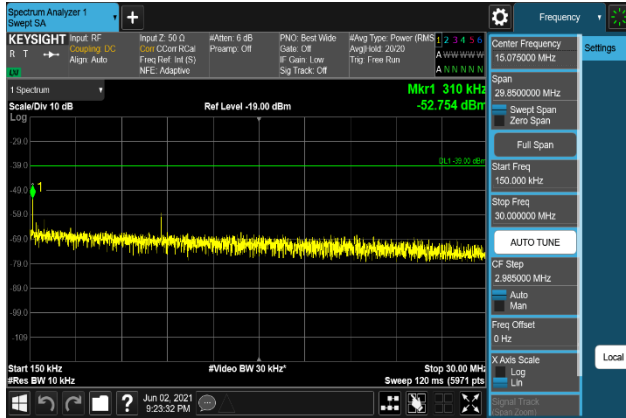
Plot 7-1577. Conducted Spurious Emission Plot 150 kHz to 30 MHz (B66_20M+5M+10M_QPSK - High Channel, Port 0)
