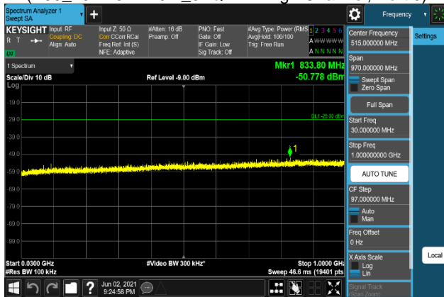
Plot 7-1581. Conducted Spurious Emission Plot 30 MHz to 1 GHz (B66_20M+5M+10M_QPSK - High Channel, Port 0)
