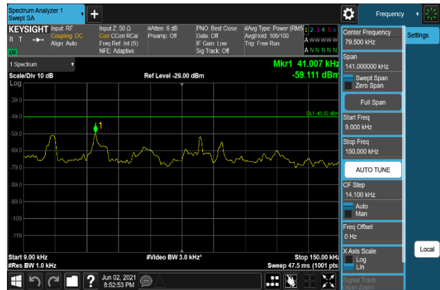
Plot 7-1548. Conducted Spurious Emission Plot 9 kHz to 150 kHz (B66_20M+5M+10M_256QAM - Middle Channel, Port 3)
