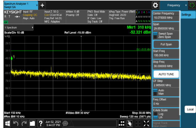
Plot 7-1578. Conducted Spurious Emission Plot 150 kHz to 30 MHz (B66_20M+5M+10M_16QAM - High Channel, Port 0)
