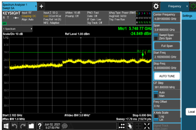
Plot 7-1589. Conducted Spurious Emission Plot 2.182 GHz to 6 GHz (B66_20M+5M+10M_QPSK - High Channel, Port 0)
