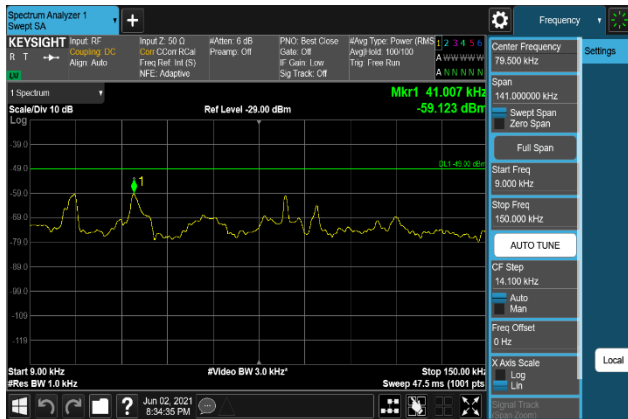
Plot 7-1547. Conducted Spurious Emission Plot 9 kHz to 150 kHz (B66_20M+5M+10M_64QAM - Middle Channel, Port 3)
