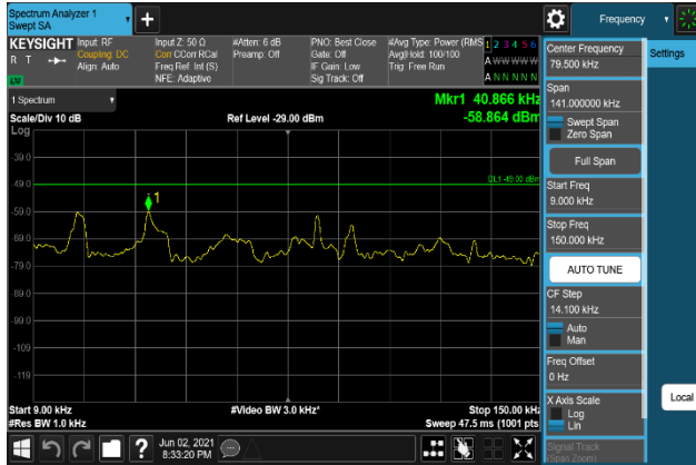
Plot 7-1463. Conducted Spurious Emission Plot 9 kHz to 150 kHz (B66_20M+5M+10M_64QAM - Middle Channel, Port 0)
