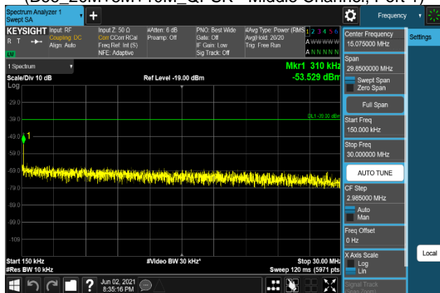
Plot 7-1495. Conducted Spurious Emission Plot 150 kHz to 30 MHz (B66_20M+5M+10M_64QAM - Middle Channel, Port 1)
