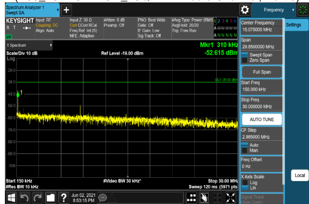
Plot 7-1468. Conducted Spurious Emission Plot 150 kHz to 30 MHz (B66_20M+5M+10M_256QAM - Middle Channel, Port 0)
