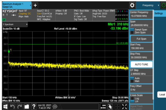
Plot 7-1493. Conducted Spurious Emission Plot 150 kHz to 30 MHz (B66_20M+5M+10M_QPSK - Middle Channel, Port 1)
