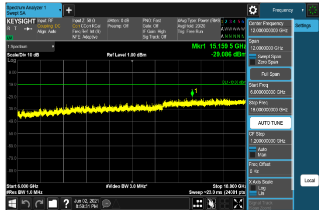
Plot 7-1512. Conducted Spurious Emission Plot 6 GHz to 18 GHz (B66_20M+5M+10M_256QAM - Middle Channel, Port 1)
