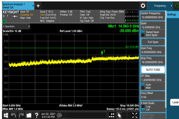
Plot 7-1511. Conducted Spurious Emission Plot 6 GHz to 18 GHz (B66_20M+5M+10M_64QAM - Middle Channel, Port 1)
