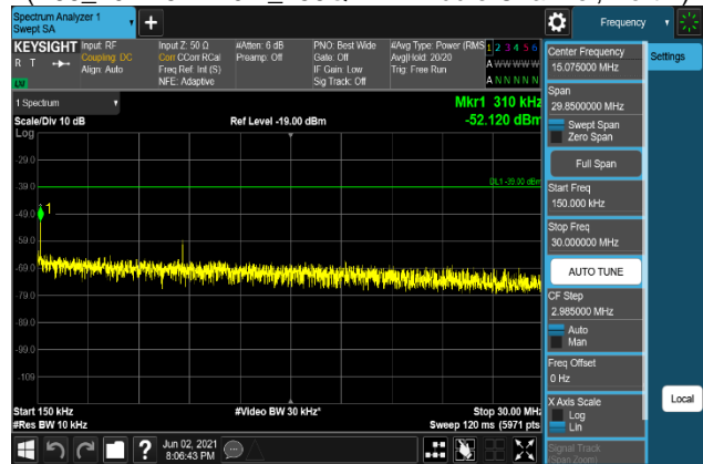
Plot 7-1522. Conducted Spurious Emission Plot 150 kHz to 30 MHz (B66_20M+5M+10M_16QAM - Middle Channel, Port 2)
