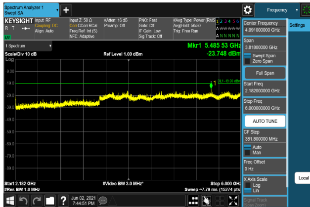
Plot 7-1505. Conducted Spurious Emission Plot 2.182 GHz to 6 GHz (B66_20M+5M+10M_QPSK - Middle Channel, Port 1)
