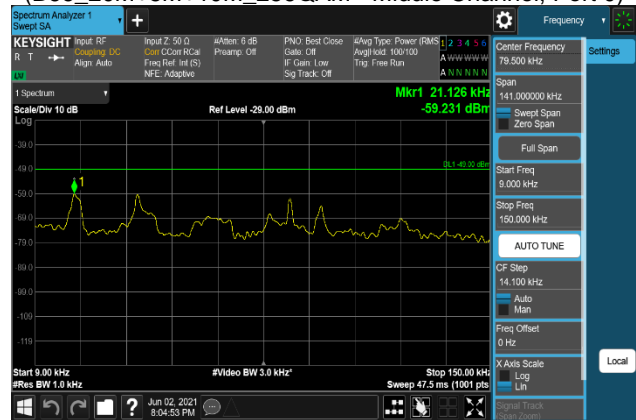
Plot 7-1490. Conducted Spurious Emission Plot 9 kHz to 150 kHz (B66_20M+5M+10M_16QAM - Middle Channel, Port 1)
