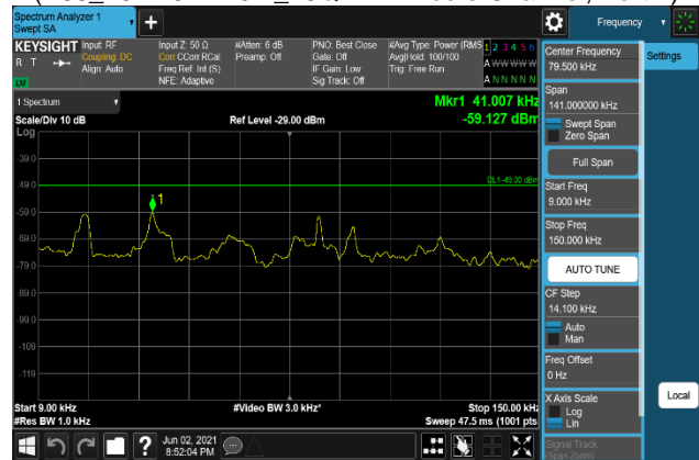
Plot 7-1492. Conducted Spurious Emission Plot 9 kHz to 150 kHz (B66_20M+5M+10M_256QAM - Middle Channel, Port 1)
