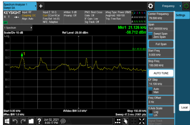
Plot 7-1518. Conducted Spurious Emission Plot 9 kHz to 150 kHz (B66_20M+5M+10M_16QAM - Middle Channel, Port 2)
