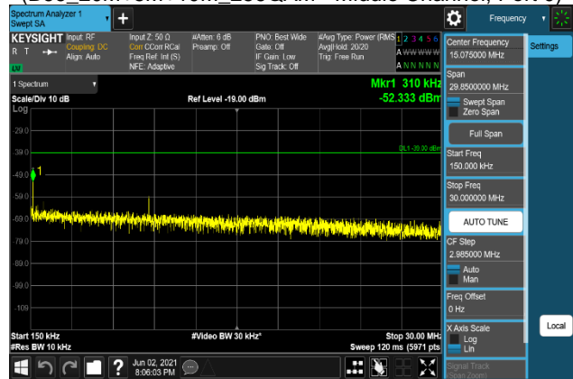
Plot 7-1466. Conducted Spurious Emission Plot 150 kHz to 30 MHz (B66_20M+5M+10M_16QAM - Middle Channel, Port 0)
