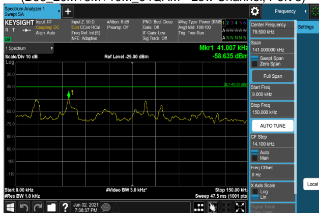
Plot 7-1461. Conducted Spurious Emission Plot 9 kHz to 150 kHz (B66_20M+5M+10M_QPSK - Middle Channel, Port 0)
