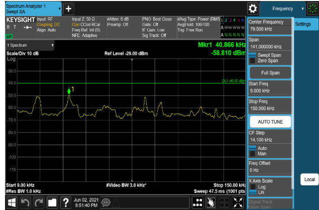
Plot 7-1464. Conducted Spurious Emission Plot 9 kHz to 150 kHz (B66_20M+5M+10M_256QAM - Middle Channel, Port 0)
