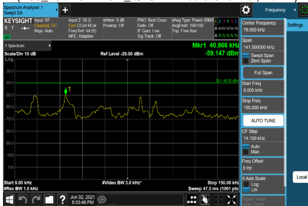
Plot 7-1491. Conducted Spurious Emission Plot 9 kHz to 150 kHz (B66_20M+5M+10M_64QAM - Middle Channel, Port 1)
