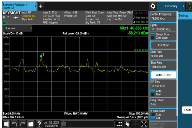
Plot 7-1517. Conducted Spurious Emission Plot 9 kHz to 150 kHz (B66_20M+5M+10M_QPSK - Middle Channel, Port 2)
