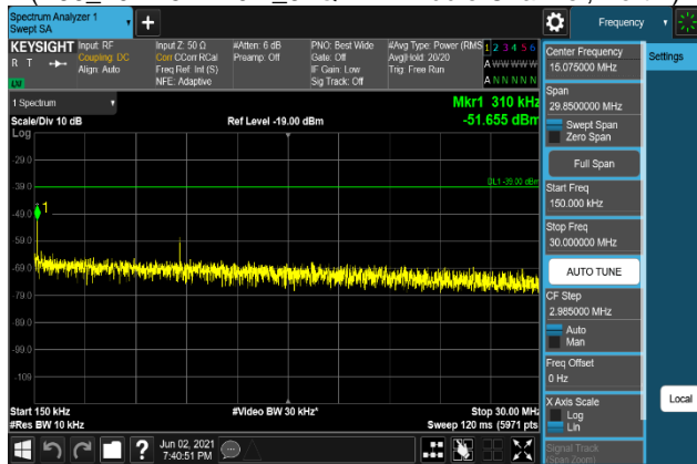
Plot 7-1521. Conducted Spurious Emission Plot 150 kHz to 30 MHz (B66_20M+5M+10M_QPSK - Middle Channel, Port 2)
