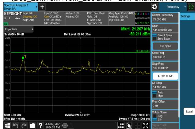
Plot 7-1462. Conducted Spurious Emission Plot 9 kHz to 150 kHz (B66_20M+5M+10M_16QAM - Middle Channel, Port 0)
