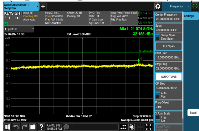
Plot 7-1516. Conducted Spurious Emission Plot 18 GHz to 22 GHz (B66_20M+5M+10M_256QAM - Middle Channel, Port 1)
