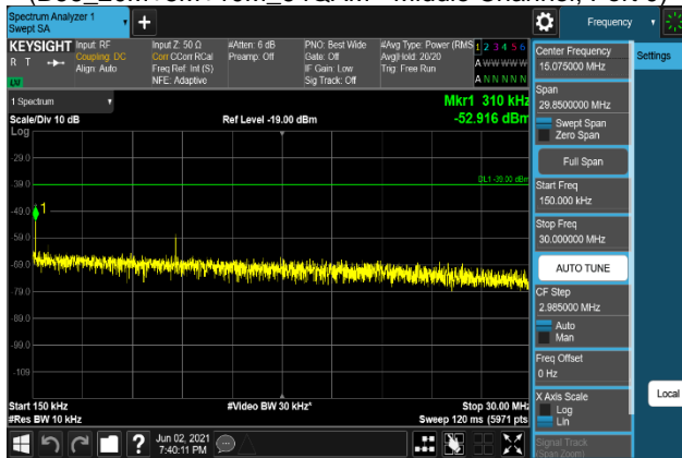
Plot 7-1465. Conducted Spurious Emission Plot 150 kHz to 30 MHz (B66_20M+5M+10M_QPSK - Middle Channel, Port 0)
