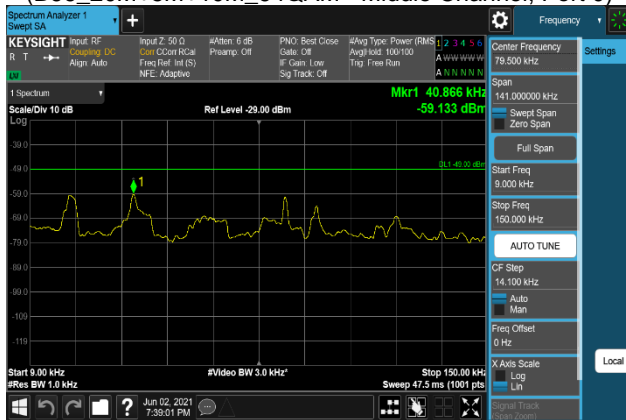
Plot 7-1489. Conducted Spurious Emission Plot 9 kHz to 150 kHz (B66_20M+5M+10M_QPSK - Middle Channel, Port 1)
