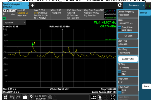
Plot 7-1520. Conducted Spurious Emission Plot 9 kHz to 150 kHz (B66_20M+5M+10M_256QAM - Middle Channel, Port 2)
