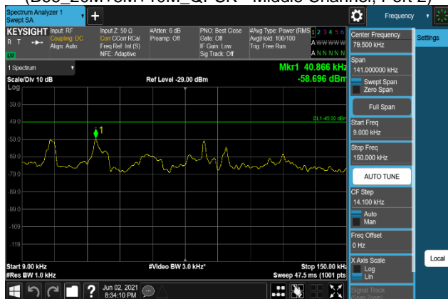
Plot 7-1519. Conducted Spurious Emission Plot 9 kHz to 150 kHz (B66_20M+5M+10M_64QAM - Middle Channel, Port 2)
