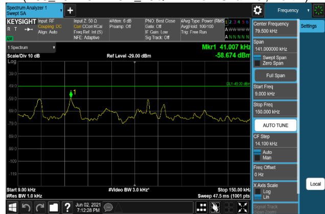
Plot 7-1408. Conducted Spurious Emission Plot 9 kHz to 150 kHz (B66_20M+5M+10M_256QAM - Low Channel, Port 2)
