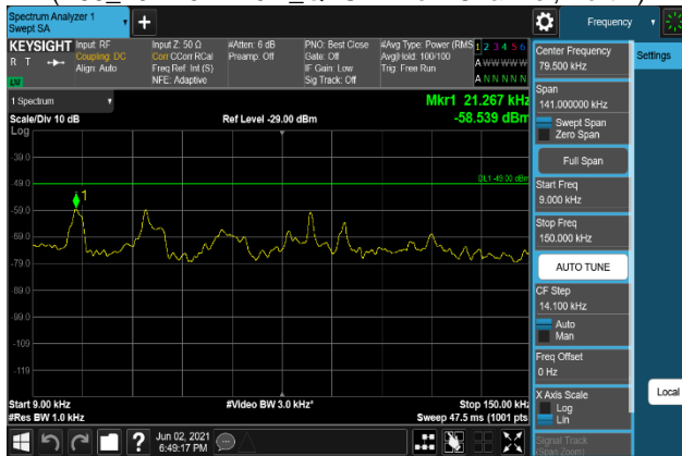
Plot 7-1407. Conducted Spurious Emission Plot 9 kHz to 150 kHz (B66_20M+5M+10M_64QAM - Low Channel, Port 2)
