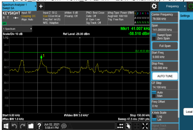
Plot 7-1405. Conducted Spurious Emission Plot 9 kHz to 150 kHz (B66_20M+5M+10M_QPSK - Low Channel, Port 2)
