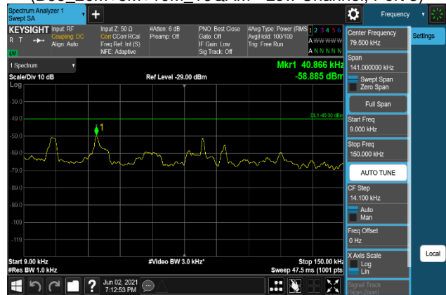
Plot 7-1436. Conducted Spurious Emission Plot 9 kHz to 150 kHz (B66_20M+5M+10M_256QAM - Low Channel, Port 3)
