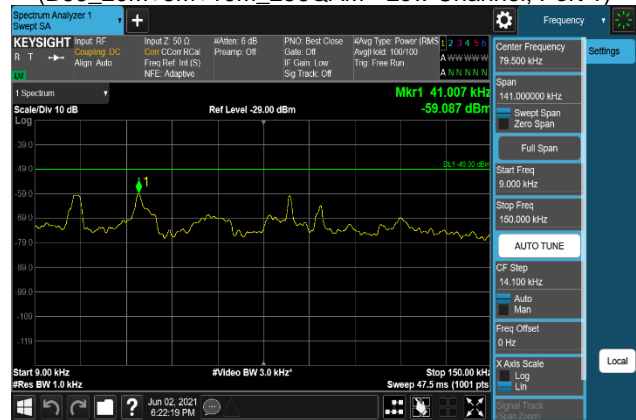
Plot 7-1406. Conducted Spurious Emission Plot 9 kHz to 150 kHz (B66_20M+5M+10M_16QAM - Low Channel, Port 2)
