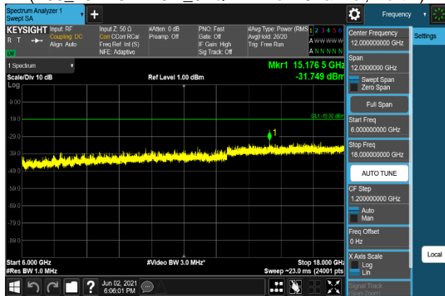
Plot 7-1425. Conducted Spurious Emission Plot 6 GHz to 18 GHz (B66_20M+5M+10M_QPSK - Low Channel, Port 2)
