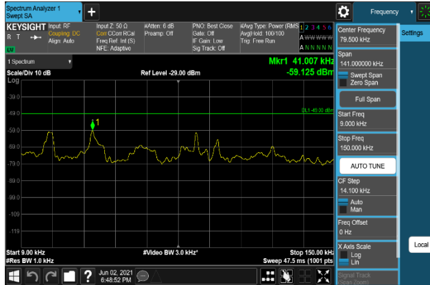
Plot 7-1379. Conducted Spurious Emission Plot 9 kHz to 150 kHz (B66_20M+5M+10M_64QAM - Low Channel, Port 1)
