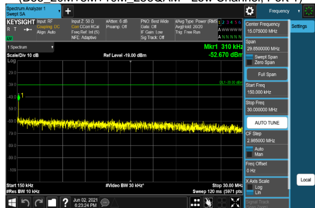
Plot 7-1382. Conducted Spurious Emission Plot 150 kHz to 30 MHz (B66_20M+5M+10M_16QAM - Low Channel, Port 1)
