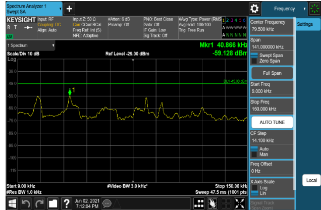
Plot 7-1380. Conducted Spurious Emission Plot 9 kHz to 150 kHz (B66_20M+5M+10M_256QAM - Low Channel, Port 1)
