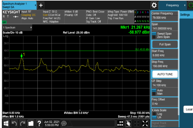
Plot 7-1433. Conducted Spurious Emission Plot 9 kHz to 150 kHz (B66_20M+5M+10M_QPSK - Low Channel, Port 3)
