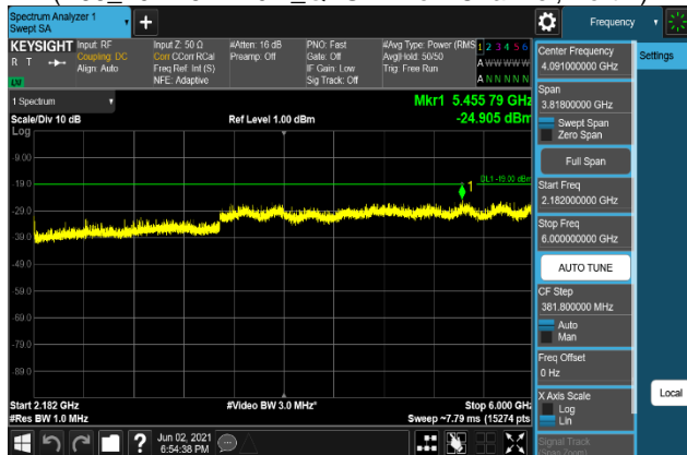
Plot 7-1395. Conducted Spurious Emission Plot 2.182 GHz to 6 GHz (B66_20M+5M+10M_64QAM - Low Channel, Port 1)
