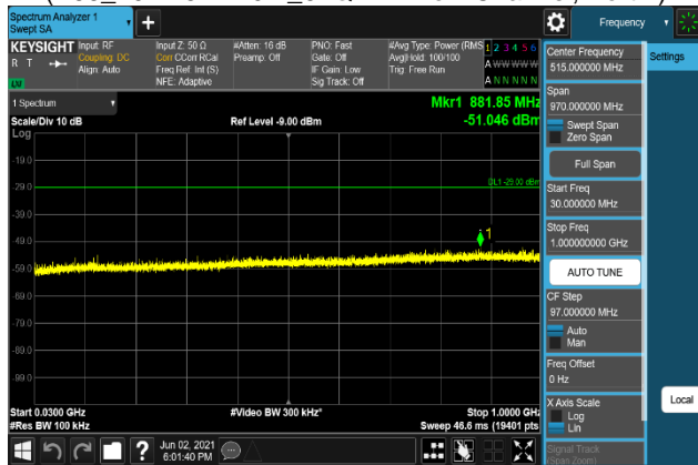
Plot 7-1413. Conducted Spurious Emission Plot 30 MHz to 1 GHz (B66_20M+5M+10M_QPSK - Low Channel, Port 2)
