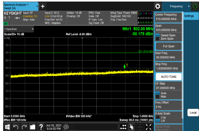
Plot 7-1386. Conducted Spurious Emission Plot 30 MHz to 1 GHz (B66_20M+5M+_16QAM - Low Channel, Port 1)
