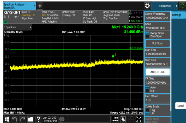
Plot 7-1428. Conducted Spurious Emission Plot 6 GHz to 18 GHz (B66_20M+5M+10M_256QAM - Low Channel, Port 2)
