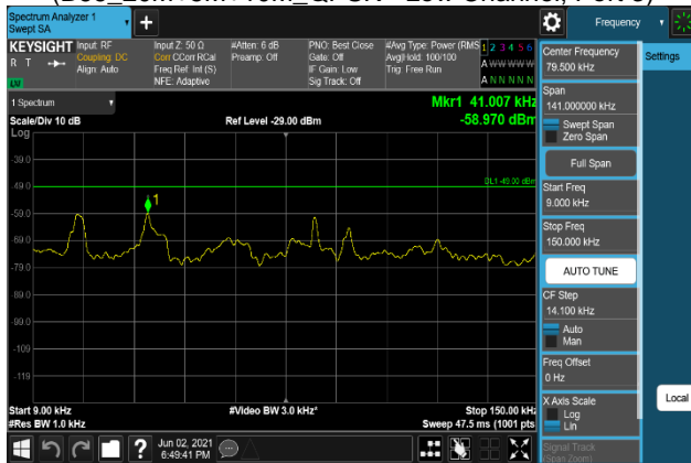
Plot 7-1435. Conducted Spurious Emission Plot 9 kHz to 150 kHz (B66_20M+5M+10M_64QAM - Low Channel, Port 3)
