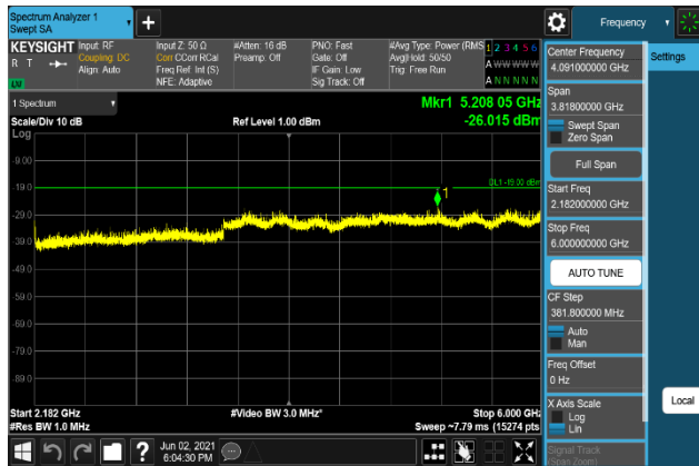
Plot 7-1421. Conducted Spurious Emission Plot 2.182 GHz to 6 GHz (B66_20M+5M+10M_QPSK - Low Channel, Port 2)
