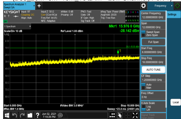
Plot 7-1400. Conducted Spurious Emission Plot 6 GHz to 18 GHz (B66_20M+5M+10M_256QAM - Low Channel, Port 1)
