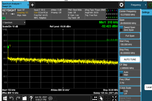
Plot 7-1383. Conducted Spurious Emission Plot 150 kHz to 30 MHz (B66_20M+5M+10M_64QAM - Low Channel, Port 1)
