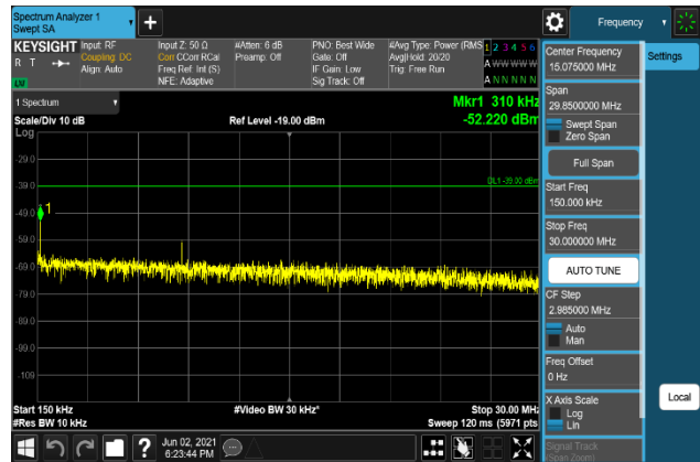
Plot 7-1410. Conducted Spurious Emission Plot 150 kHz to 30 MHz (B66_20M+5M+10M_16QAM - Low Channel, Port 2)
