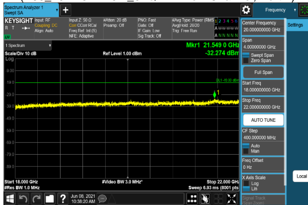
Plot 7-1401. Conducted Spurious Emission Plot 18 GHz to 22 GHz (B66_20M+5M+10M_QPSK - Low Channel, Port 1)
