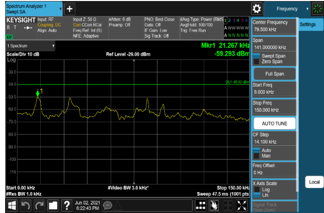
Plot 7-1434. Conducted Spurious Emission Plot 9 kHz to 150 kHz (B66_20M+5M+10M_16QAM - Low Channel, Port 3)
