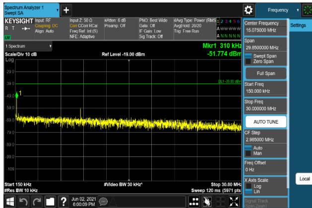
Plot 7-1409. Conducted Spurious Emission Plot 150 kHz to 30 MHz (B66_20M+5M+10M_QPSK - Low Channel, Port 2)
