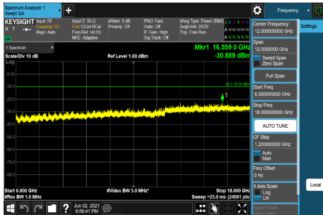
Plot 7-1427. Conducted Spurious Emission Plot 6 GHz to 18 GHz (B66_20M+5M+10M_64QAM - Low Channel, Port 2)
