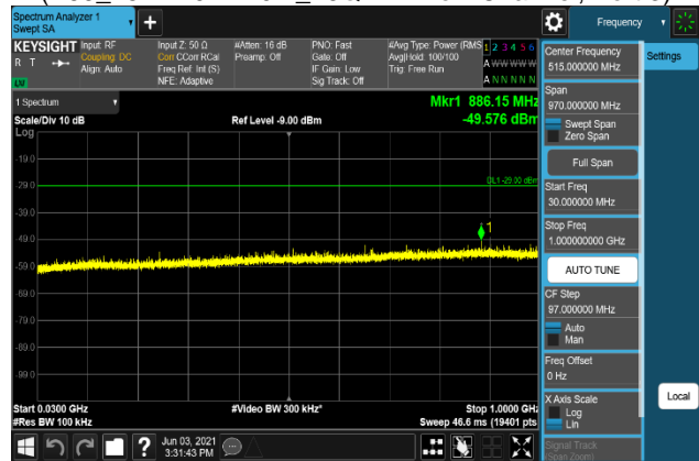
Plot 7-1332. Conducted Spurious Emission Plot 30 MHz to 1 GHz (B66_15M+10M+10M_256QAM - Low Channel, Port 3)
