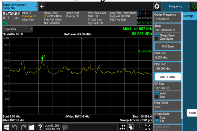
Plot 7-1349. Conducted Spurious Emission Plot 9 kHz to 150 kHz (B66_20M+5M+10M_QPSK - Low Channel, Port 0)
