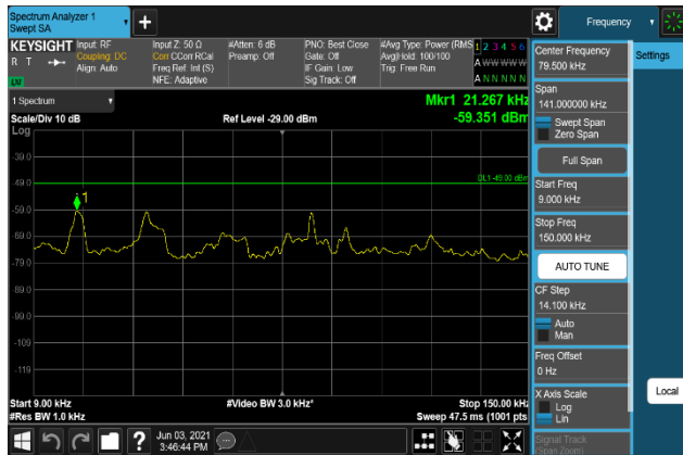
Plot 7-1321. Conducted Spurious Emission Plot 9 kHz to 150 kHz (B66_15M+10M+10M_QPSK - Low Channel, Port 3)
