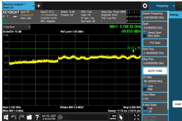
Plot 7-1309. Conducted Spurious Emission Plot 2.182 GHz to 6 GHz (B66_15M+10M+10M_QPSK - Low Channel, Port 2)
