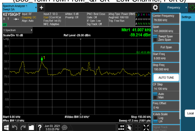
Plot 7-1323. Conducted Spurious Emission Plot 9 kHz to 150 kHz (B66_15M+10M+10M_64QAM - Low Channel, Port 3)
