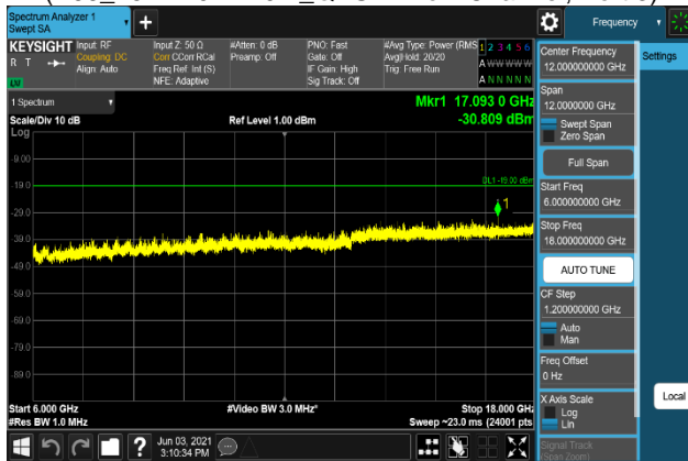
Plot 7-1343. Conducted Spurious Emission Plot 6 GHz to 18 GHz (B66_15M+10M+10M_64QAM - Low Channel, Port 3)
