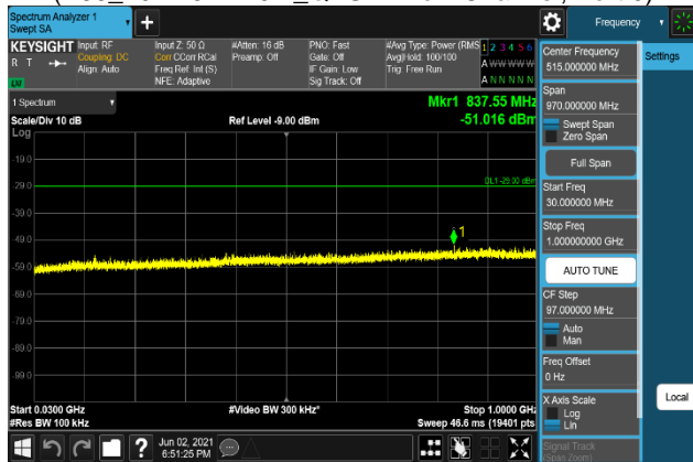
Plot 7-1359. Conducted Spurious Emission Plot 30 MHz to 1 GHz (B66_20M+5M+10M_64QAM - Low Channel, Port 0)
