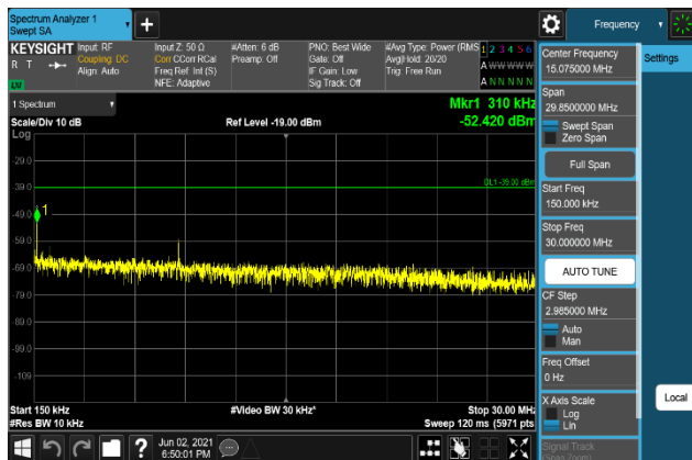
Plot 7-1355. Conducted Spurious Emission Plot 150 kHz to 30 MHz (B66_20M+5M+10M_64QAM - Low Channel, Port 0)
