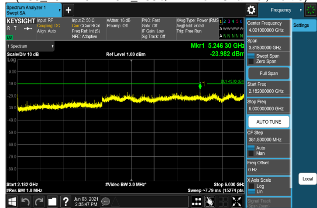
Plot 7-1338. Conducted Spurious Emission Plot 2.182 GHz to 6 GHz (B66_15M+10M+10M_16QAM - Low Channel, Port 3)
