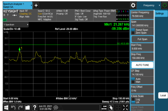
Plot 7-1322. Conducted Spurious Emission Plot 9 kHz to 150 kHz (B66_15M+10M+10M_16QAM - Low Channel, Port 3)
