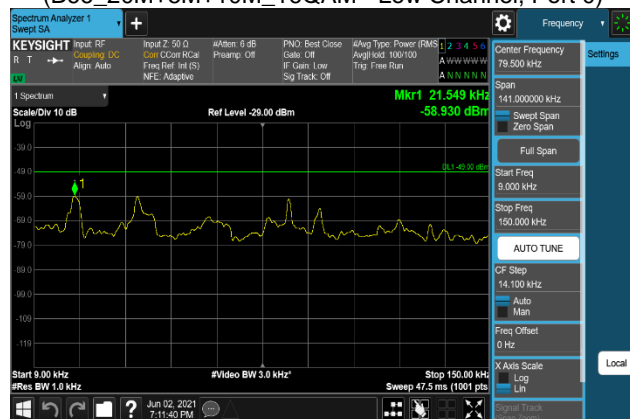
Plot 7-1352. Conducted Spurious Emission Plot 9 kHz to 150 kHz (B66_20M+5M+10M_256QAM - Low Channel, Port 0)
