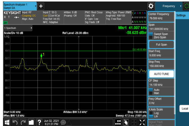
Plot 7-1350. Conducted Spurious Emission Plot 9 kHz to 150 kHz (B66_20M+5M+10M_16QAM - Low Channel, Port 0)
