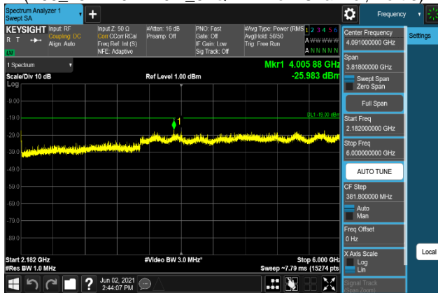
Plot 7-1337. Conducted Spurious Emission Plot 2.182 GHz to 6 GHz (B66_15M+10M+10M_QPSK - Low Channel, Port 3)
