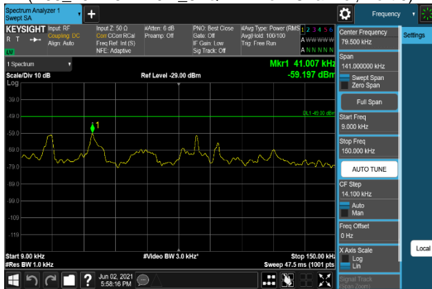
Plot 7-1377. Conducted Spurious Emission Plot 9 kHz to 150 kHz (B66_20M+5M+10M_QPSK - Low Channel, Port 1)
