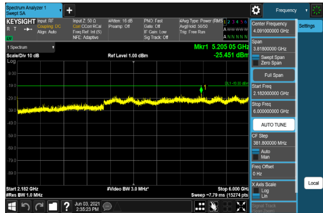
Plot 7-1310. Conducted Spurious Emission Plot 2.182 GHz to 6 GHz (B66_15M+10M+10M_16QAM - Low Channel, Port 2)
