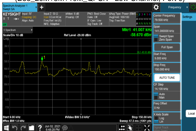
Plot 7-1351. Conducted Spurious Emission Plot 9 kHz to 150 kHz (B66_20M+5M+10M_64QAM - Low Channel, Port 0)
