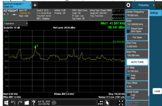
Plot 7-1378. Conducted Spurious Emission Plot 9 kHz to 150 kHz (B66_20M+5M+10M_16QAM - Low Channel, Port 1)
