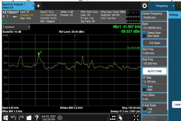
Plot 7-1295. Conducted Spurious Emission Plot 9 kHz to 150 kHz (B66_15M+10M+10M_64QAM - Low Channel, Port 2)
