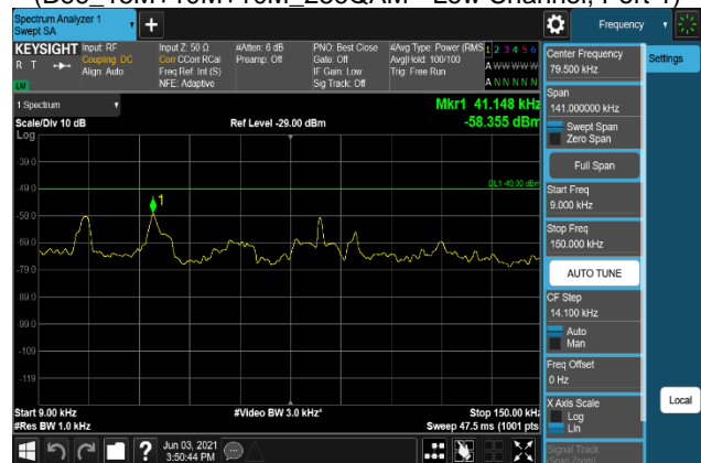
Plot 7-1294. Conducted Spurious Emission Plot 9 kHz to 150 kHz (B66_15M+10M+10M_256QAM - Low Channel, Port 2)
