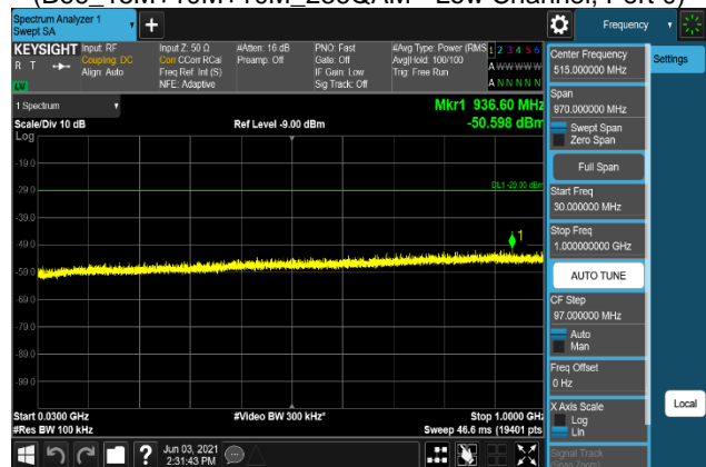
Plot 7-1246. Conducted Spurious Emission Plot 30 MHz to 1 GHz (B66_15M+10M+10M_16QAM - Low Channel, Port 0)
