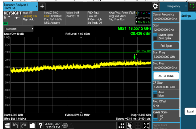
Plot 7-1288. Conducted Spurious Emission Plot 6 GHz to 18 GHz (B66_15M+10M+10M_256QAM - Low Channel, Port 1)
