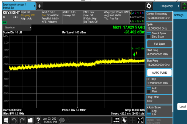
Plot 7-1259. Conducted Spurious Emission Plot 6 GHz to 18 GHz (B66_15M+10M+10M_64QAM - Low Channel, Port 0)
