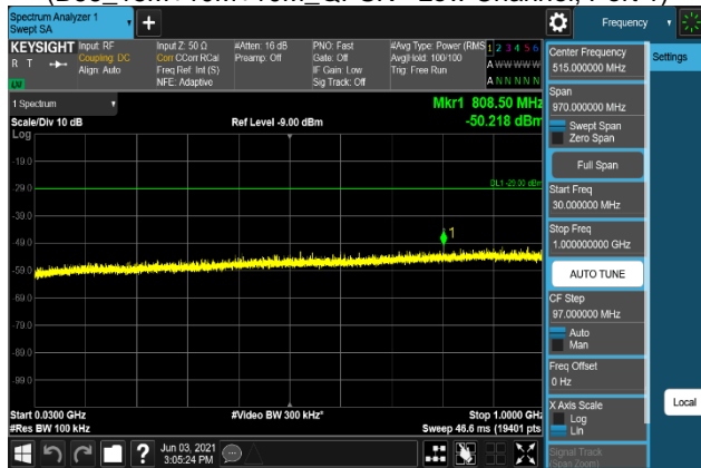
Plot 7-1275. Conducted Spurious Emission Plot 30 MHz to 1 GHz (B66_15M+10M+10M_64Q AM - Low Channel, Port 1)
