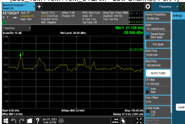
Plot 7-1293. Conducted Spurious Emission Plot 9 kHz to 150 kHz (B66_15M+10M+10M_QPSK - Low Channel, Port 2)
