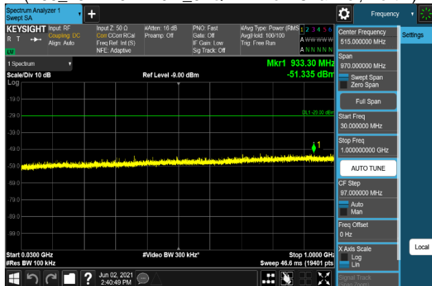
Plot 7-1301. Conducted Spurious Emission Plot 30 MHz to 1 GHz (B66_15M+10M+10M_QPSK - Low Channel, Port 2)
