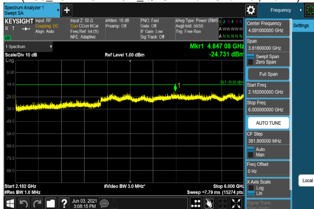
Plot 7-1283. Conducted Spurious Emission Plot 2.182 GHz to 6 GHz (B66_15M+10M+10M_64QAM - Low Channel, Port 1)
