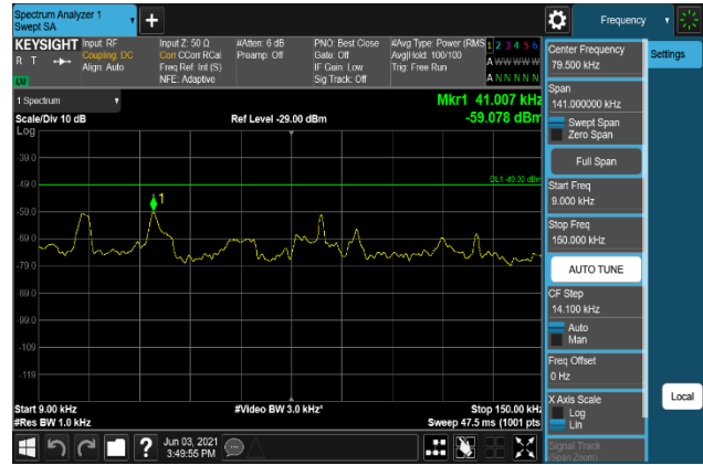
Plot 7-1238. Conducted Spurious Emission Plot 9 kHz to 150 kHz (B66_15M+10M+10M_16QAM - Low Channel, Port 0)
