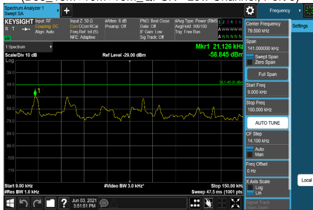
Plot 7-1239. Conducted Spurious Emission Plot 9 kHz to 150 kHz (B66_15M+10M+10M_64QAM - Low Channel, Port 0)
