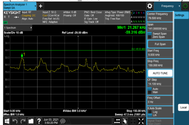
Plot 7-1266. Conducted Spurious Emission Plot 9 kHz to 150 kHz (B66_15M+10M+10M_16QAM - Low Channel, Port 1)
