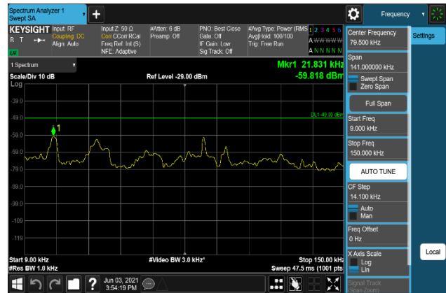
Plot 7-1268. Conducted Spurious Emission Plot 9 kHz to 150 kHz (B66_15M+10M+10M_256QAM - Low Channel, Port 1)
