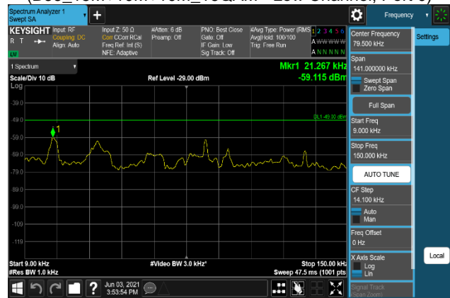
Plot 7-1240. Conducted Spurious Emission Plot 9 kHz to 150 kHz (B66_15M+10M+10M_256QAM - Low Channel, Port 0)
