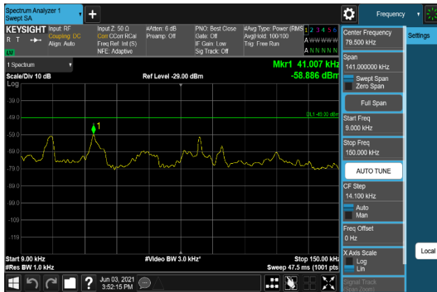
Plot 7-1267. Conducted Spurious Emission Plot 9 kHz to 150 kHz (B66_15M+10M+10M_64QAM - Low Channel, Port 1)
