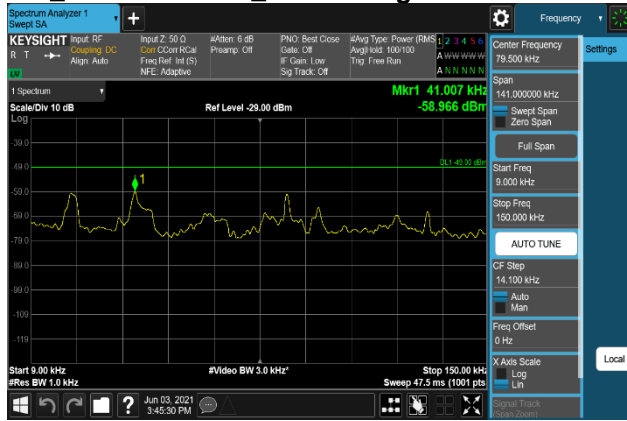
Plot 7-1237. Conducted Spurious Emission Plot 9 kHz to 150 kHz (B66_15M+10M+10M_QPSK - Low Channel, Port 0)
