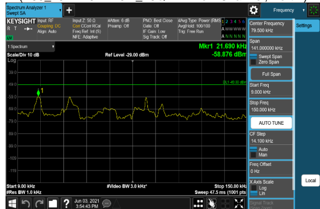
Plot 7-1296. Conducted Spurious Emission Plot 9 kHz to 150 kHz (B66_15M+10M+10M_256QAM - Low Channel, Port 2)
