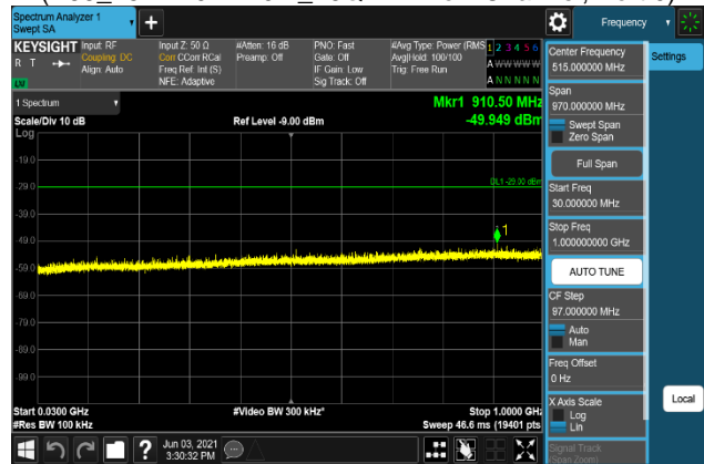
Plot 7-1248. Conducted Spurious Emission Plot 30 MHz to 1 GHz (B66_15M+10M+10M_256QAM - Low Channel, Port 0)
