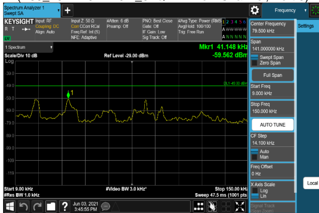
Plot 7-1265. Conducted Spurious Emission Plot 9 kHz to 150 kHz (B66_15M+10M+10M_QPSK - Low Channel, Port 1)
