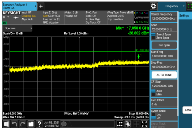
Plot 7-1285. Conducted Spurious Emission Plot 6 GHz to 18 GHz (B66_15M+10M+10M_QPSK - Low Channel, Port 1)
