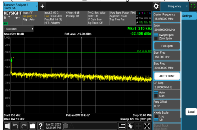
Plot 7-1188. Conducted Spurious Emission Plot 150 kHz to 30 MHz (B66_15M+10M+10M_256QAM - High Channel, Port 2)
