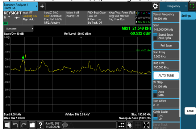
Plot 7-1210. Conducted Spurious Emission Plot 9 kHz to 150 kHz (B66_15M+10M+10M_256QAM - High Channel, Port 3)
