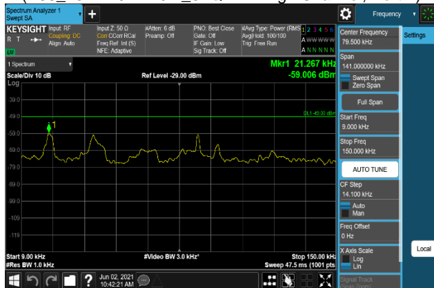
Plot 7-1181. Conducted Spurious Emission Plot 9 kHz to 150 kHz (B66_15M+10M+10M_QPSK - High Channel, Port 2)
