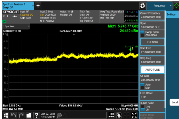
Plot 7-1171. Conducted Spurious Emission Plot 2.182 GHz to 6 GHz (B66_15M+10M+10M_64QAM - High Channel, Port 1)
