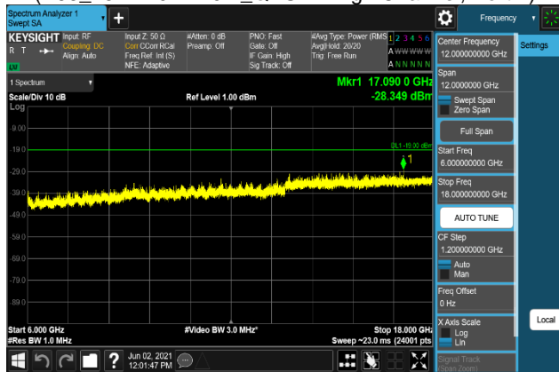
Plot 7-1175. Conducted Spurious Emission Plot 6 GHz to 18 GHz (B66_15M+10M+10M_64QAM - High Channel, Port 1)
