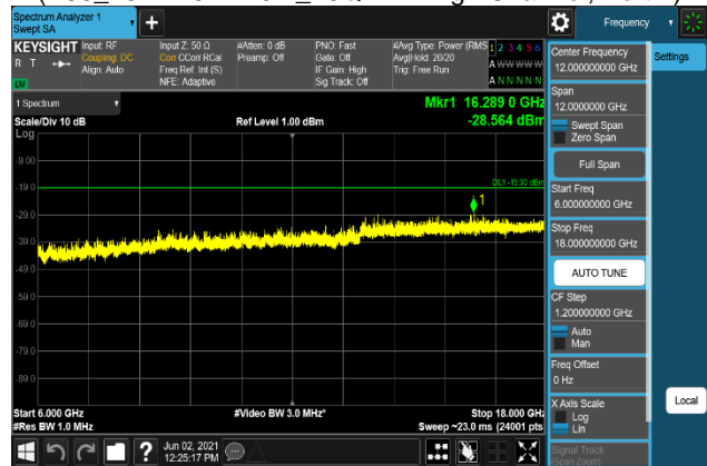
Plot 7-1176. Conducted Spurious Emission Plot 6 GHz to 18 GHz (B66_15M+10M+10M_256QAM - High Channel, Port 1)
