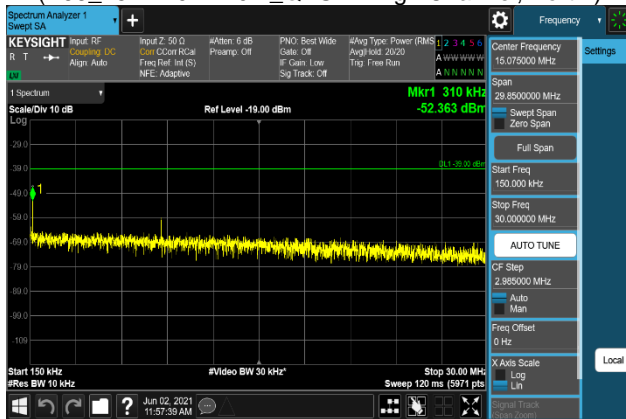
Plot 7-1187. Conducted Spurious Emission Plot 150 kHz to 30 MHz (B66_15M+10M+10M_64QAM - High Channel, Port 2)
