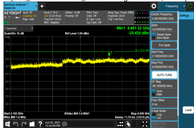
Plot 7-1200. Conducted Spurious Emission Plot 2.182 GHz to 6 GHz (B66_15M+10M+10M_256QAM - High Channel, Port 2)
