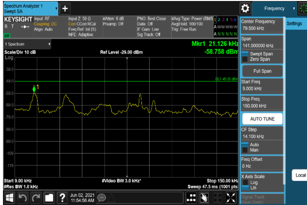
Plot 7-1183. Conducted Spurious Emission Plot 9 kHz to 150 kHz (B66_15M+10M+10M_64QAM - High Channel, Port 2)
