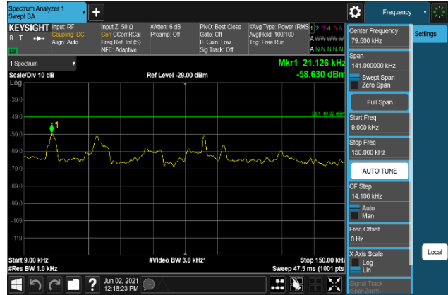
Plot 7-1184. Conducted Spurious Emission Plot 9 kHz to 150 kHz (B66_15M+10M+10M_256QAM - High Channel, Port 2)
