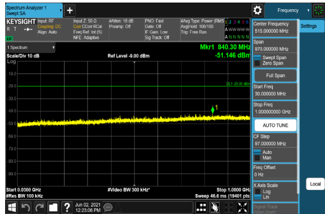
Plot 7-1220. Conducted Spurious Emission Plot 30 MHz to 1 GHz (B66_15M+10M+10M_256QAM - High Channel, Port 3)
