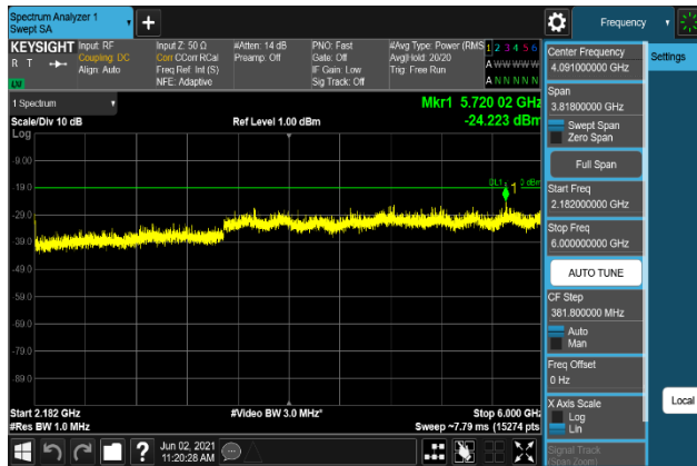
Plot 7-1225. Conducted Spurious Emission Plot 2.182 GHz to 6 GHz (B66_15M+10M+10M_QPSK - High Channel, Port 3)
