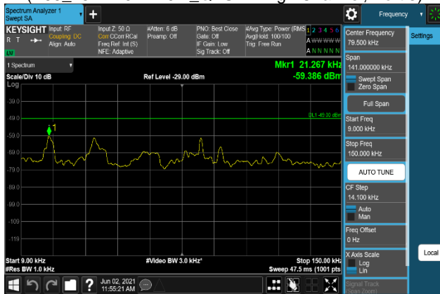
Plot 7-1211. Conducted Spurious Emission Plot 9 kHz to 150 kHz (B66_15M+10M+10M_64QAM - High Channel, Port 3)
