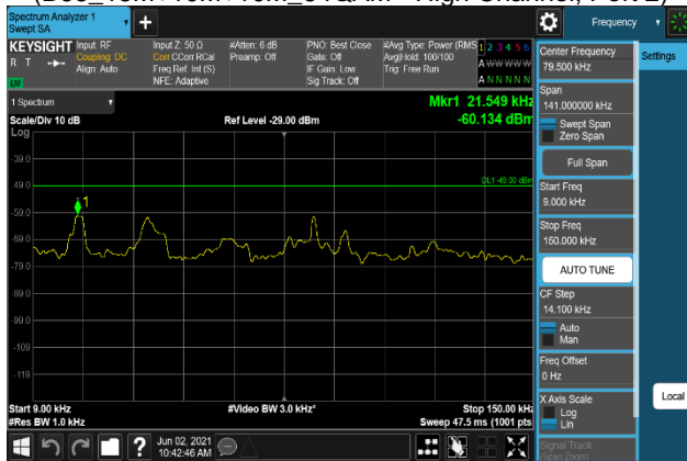
Plot 7-1209. Conducted Spurious Emission Plot 9 kHz to 150 kHz (B66_15M+10M+10M_QPSK - High Channel, Port 3)
