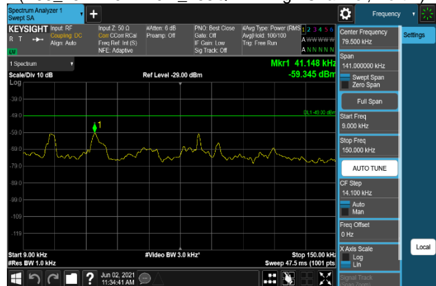
Plot 7-1182. Conducted Spurious Emission Plot 9 kHz to 150 kHz (B66_15M+10M+10M_16QAM - High Channel, Port 2)
