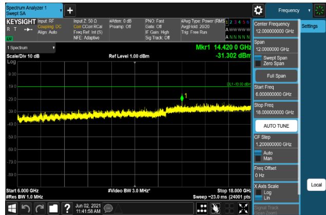
Plot 7-1202. Conducted Spurious Emission Plot 6 GHz to 18 GHz (B66_15M+10M+10M_16QAM - High Channel, Port 2)
