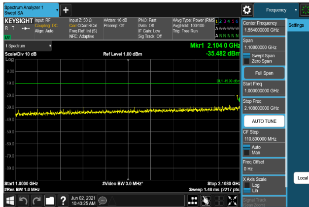
Plot 7-1165. Conducted Spurious Emission Plot 1 GHz to 2.108 GHz (B66_15M+10M+10M_QPSK - High Channel, Port 1)
