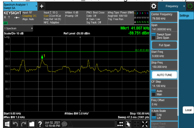
Plot 7-1212. Conducted Spurious Emission Plot 9 kHz to 150 kHz (B66_15M+10M+10M_256QAM - High Channel, Port 3)
