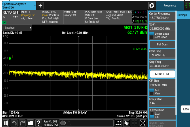
Plot 7-1103. Conducted Spurious Emission Plot 150 kHz to 30 MHz (B66_15M+10M+10M_64QAM - Middle Channel, Port 3)
