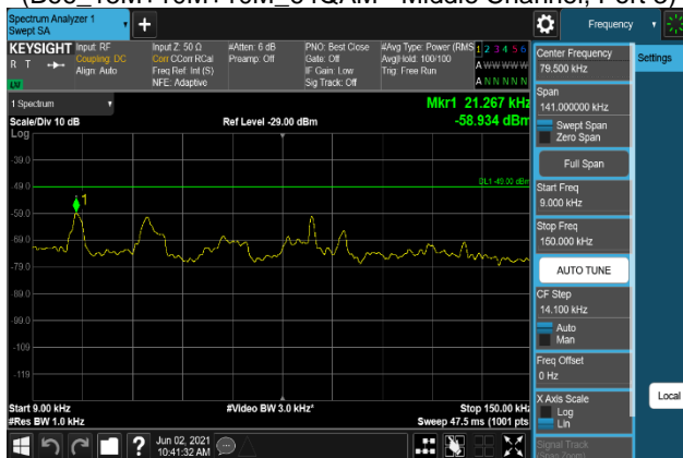
Plot 7-1125. Conducted Spurious Emission Plot 9 kHz to 150 kHz (B66_15M+10M+10M_QPSK - High Channel, Port 0)
