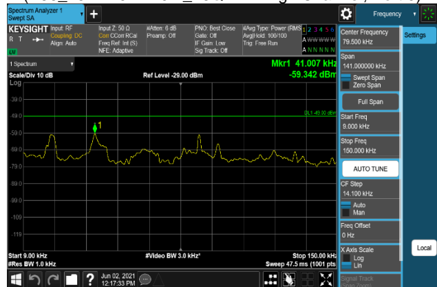
Plot 7-1128. Conducted Spurious Emission Plot 9 kHz to 150 kHz (B66_15M+10M+10M_256QAM - High Channel, Port 0)
