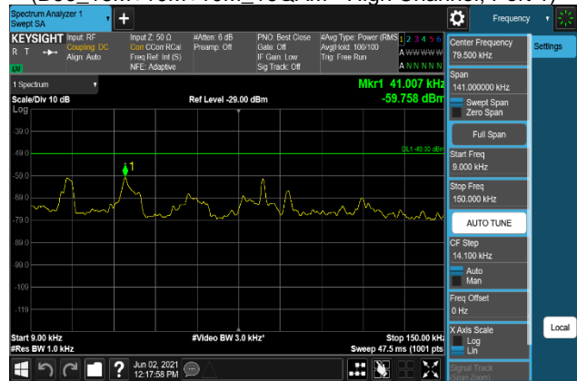
Plot 7-1156. Conducted Spurious Emission Plot 9 kHz to 150 kHz (B66_15M+10M+10M_256QAM - High Channel, Port 1)
