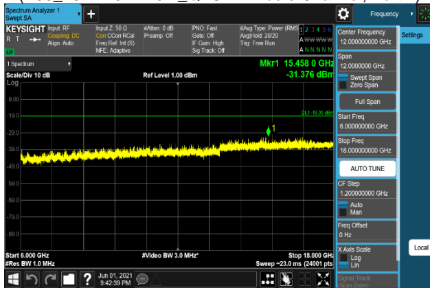
Plot 7-1091. Conducted Spurious Emission Plot 6 GHz to 18 GHz (B66_15M+10M+10M_64QAM - Middle Channel, Port 2)
