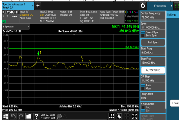
Plot 7-1155. Conducted Spurious Emission Plot 9 kHz to 150 kHz (B66_15M+10M+10M_64QAM - High Channel, Port 1)
