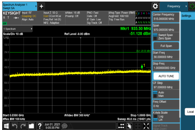
Plot 7-1105. Conducted Spurious Emission Plot 30 MHz to 1 GHz (B66_15M+10M+10M_QPSK - Middle Channel, Port 3)
