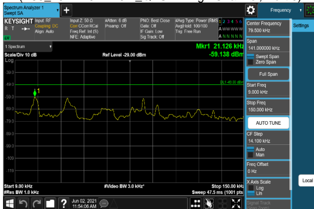
Plot 7-1127. Conducted Spurious Emission Plot 9 kHz to 150 kHz (B66_15M+10M+10M_64QAM - High Channel, Port 0)
