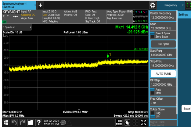
Plot 7-1147. Conducted Spurious Emission Plot 6 GHz to 18 GHz (B66_15M+10M+10M_64QAM - High Channel, Port 0)
