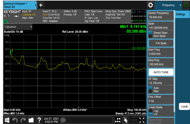
Plot 7-1100. Conducted Spurious Emission Plot 9 kHz to 150 kHz (B66_15M+10M+10M_256QAM - Middle Channel, Port 3)
