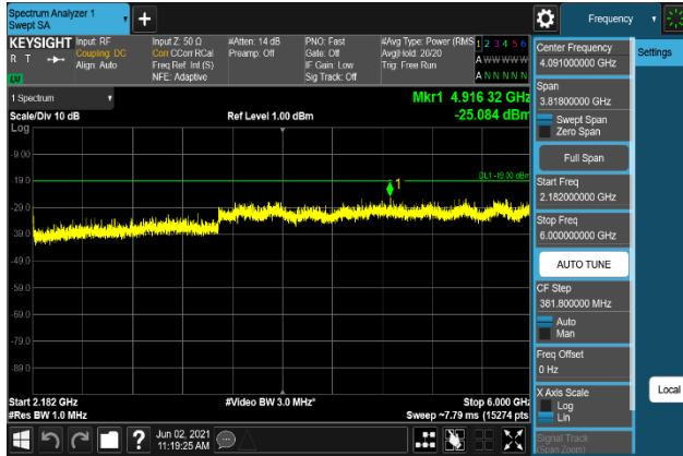
Plot 7-1141. Conducted Spurious Emission Plot 2.182 GHz to 6 GHz (B66_15M+10M+10M_QPSK - High Channel, Port 0)
