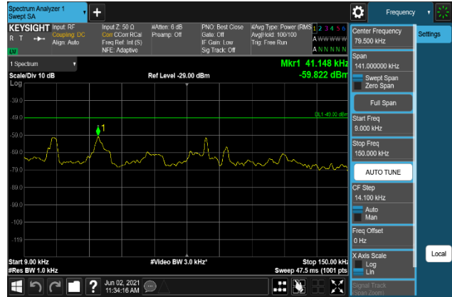
Plot 7-1154. Conducted Spurious Emission Plot 9 kHz to 150 kHz (B66_15M+10M+10M_16QAM - High Channel, Port 1)
