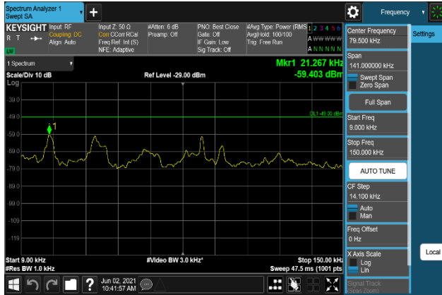
Plot 7-1153. Conducted Spurious Emission Plot 9 kHz to 150 kHz (B66_15M+10M+10M_QPSK - High Channel, Port 1)
