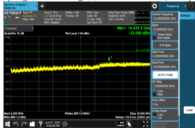
Plot 7-1092. Conducted Spurious Emission Plot 6 GHz to 18 GHz (B66_15M+10M+10M_256QAM - Middle Channel, Port 2)
