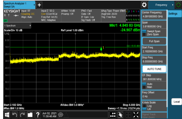
Plot 7-1142. Conducted Spurious Emission Plot 2.182 GHz to 6 GHz (B66_15M+10M+10M_16QAM - High Channel, Port 0)
