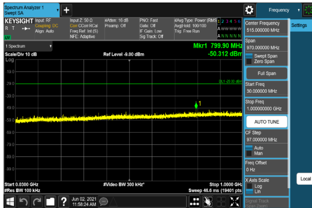
Plot 7-1135. Conducted Spurious Emission Plot 30 MHz to 1 GHz (B66_15M+10M+10M_64QAM - High Channel, Port 0)
