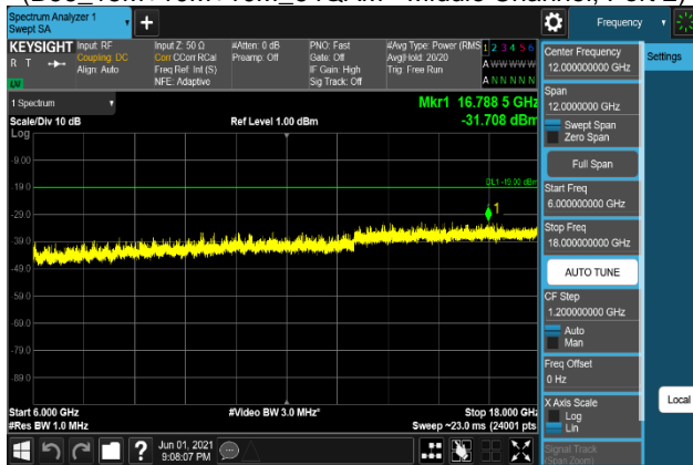
Plot 7-1089. Conducted Spurious Emission Plot 6 GHz to 18 GHz (B66_15M+10M+10M_QPSK - Middle Channel, Port 2)
