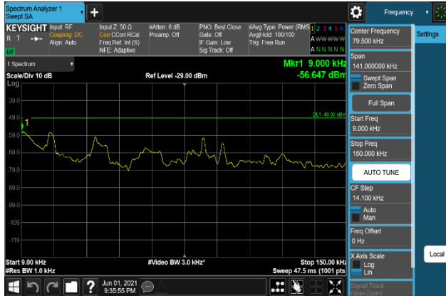
Plot 7-1099. Conducted Spurious Emission Plot 9 kHz to 150 kHz (B66_15M+10M+10M_64QAM - Middle Channel, Port 3)
