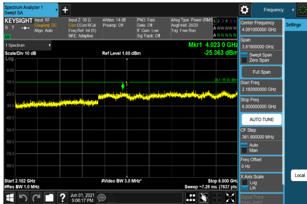
Plot 7-1057. Conducted Spurious Emission Plot 2.182 GHz to 6 GHz (B66_15M+10M+10M_QPSK - Middle Channel, Port 1)
