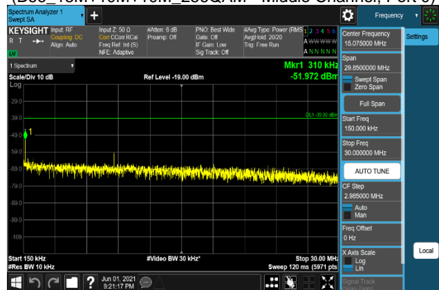
Plot 7-1018. Conducted Spurious Emission Plot 150 kHz to 30 MHz (B66_15M+10M+10M_16QAM - Middle Channel, Port 0)
