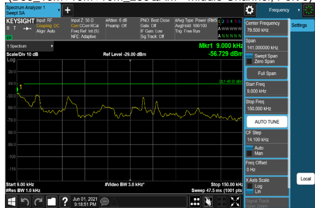
Plot 7-1042. Conducted Spurious Emission Plot 9 kHz to 150 kHz (B66_15M+10M+10M_16QAM - Middle Channel, Port 1)
