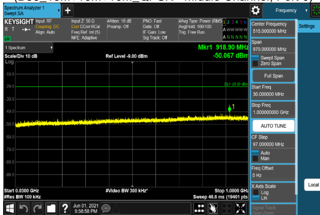
Plot 7-1023. Conducted Spurious Emission Plot 30 MHz to 1 GHz (B66_15M+10M+10M_64QAM - Middle Channel, Port 0)
