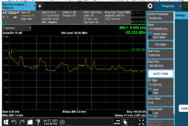
Plot 7-1071. Conducted Spurious Emission Plot 9 kHz to 150 kHz (B66_15M+10M+10M_64QAM - Middle Channel, Port 2)
