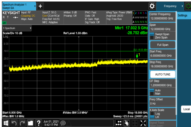
Plot 7-1063. Conducted Spurious Emission Plot 6 GHz to 18 GHz (B66_15M+10M+10M_64QAM - Middle Channel, Port 1)
