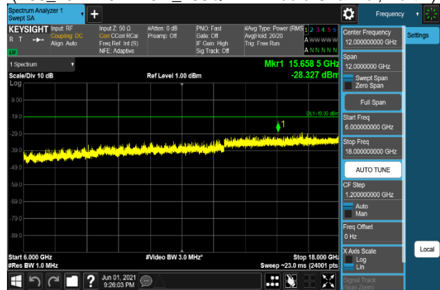
Plot 7-1062. Conducted Spurious Emission Plot 6 GHz to 18 GHz (B66_15M+10M+10M_16QAM - Middle Channel, Port 1)
