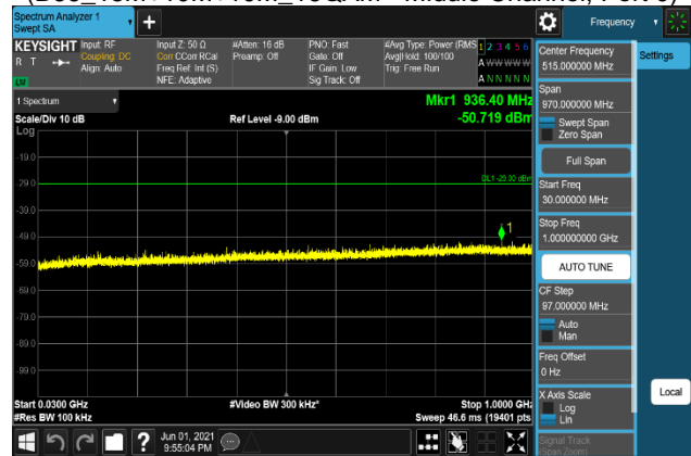
Plot 7-1024. Conducted Spurious Emission Plot 30 MHz to 1 GHz (B66_15M+10M+10M_256QAM - Middle Channel, Port 0)
