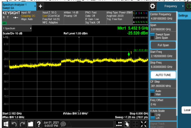
Plot 7-1029. Conducted Spurious Emission Plot 2.182 GHz to 6 GHz (B66_15M+10M+10M_QPSK - Middle Channel, Port 0)
