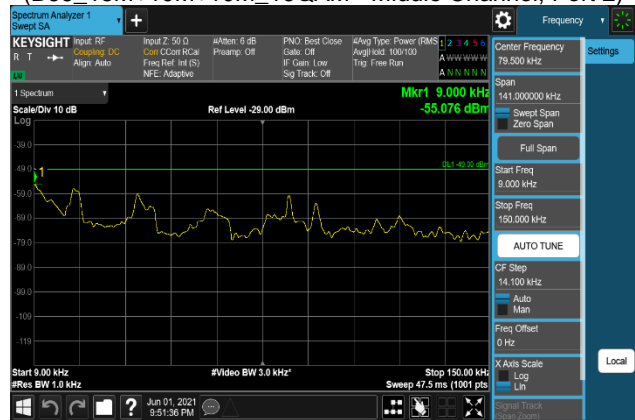
Plot 7-1072. Conducted Spurious Emission Plot 9 kHz to 150 kHz (B66_15M+10M+10M_256QAM - Middle Channel, Port 2)
