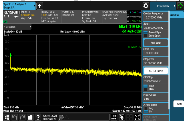
Plot 7-1020. Conducted Spurious Emission Plot 150 kHz to 30 MHz (B66_15M+10M+10M_256QAM - Middle Channel, Port 0)
