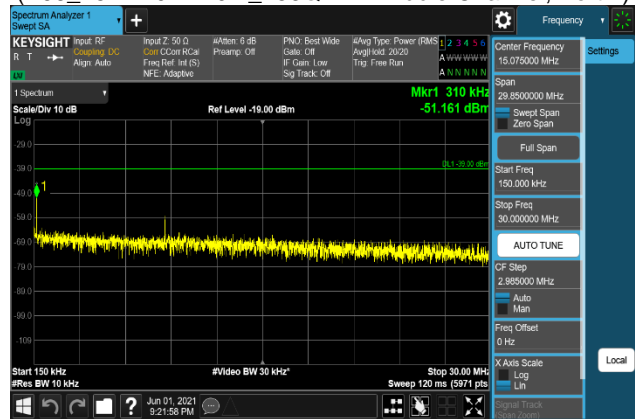
Plot 7-1074. Conducted Spurious Emission Plot 150 kHz to 30 MHz (B66_15M+10M+10M_16QAM - Middle Channel, Port 2)
