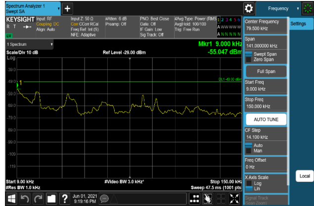
Plot 7-1070. Conducted Spurious Emission Plot 9 kHz to 150 kHz (B66_15M+10M+10M_16QAM - Middle Channel, Port 2)
