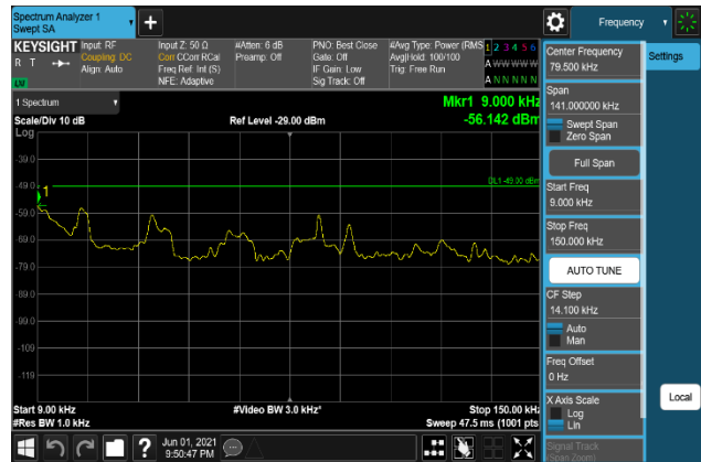
Plot 7-1016. Conducted Spurious Emission Plot 9 kHz to 150 kHz (B66_15M+10M+10M_256QAM - Middle Channel, Port 0)
