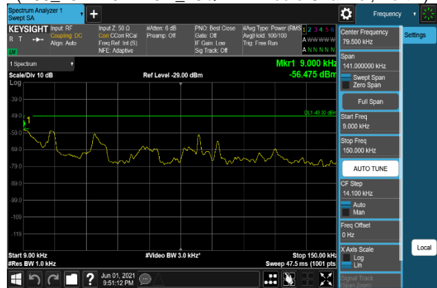
Plot 7-1044. Conducted Spurious Emission Plot 9 kHz to 150 kHz (B66_15M+10M+10M_256QAM - Middle Channel, Port 1)
