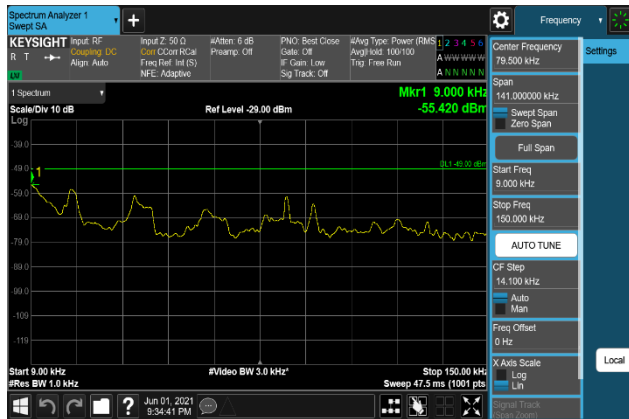
Plot 7-1015. Conducted Spurious Emission Plot 9 kHz to 150 kHz (B66_15M+10M+10M_64QAM - Middle Channel, Port 0)
