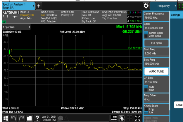
Plot 7-1043. Conducted Spurious Emission Plot 9 kHz to 150 kHz (B66_15M+10M+10M_64QAM - Middle Channel, Port 1)
