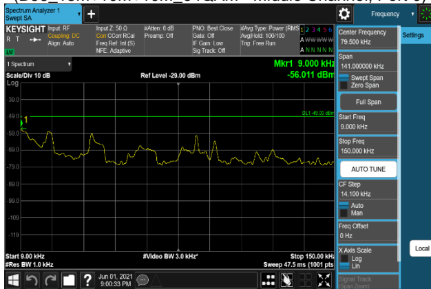
Plot 7-1041. Conducted Spurious Emission Plot 9 kHz to 150 kHz (B66_15M+10M+10M_QPSK - Middle Channel, Port 1)
