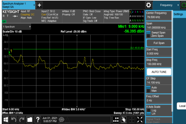
Plot 7-1069. Conducted Spurious Emission Plot 9 kHz to 150 kHz (B66_15M+10M+10M_QPSK - Middle Channel, Port 2)
