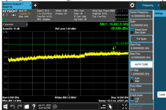
Plot 7-1061. Conducted Spurious Emission Plot 6 GHz to 18 GHz (B66_15M+10M+10M_QPSK - Middle Channel, Port 1)
