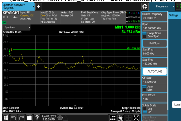
Plot 7-957. Conducted Spurious Emission Plot 9 kHz to 150 kHz (B66_15M+10M+10M_QPSK - Low Channel, Port 2)
