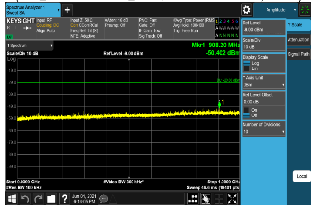
Plot 7-966. Conducted Spurious Emission Plot 30 MHz to 1 GHz (B66_15M+10M+10M_16QAM - Low Channel, Port 2)
