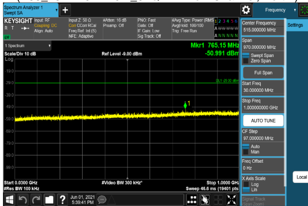
Plot 7-965. Conducted Spurious Emission Plot 30 MHz to 1 GHz (B66_15M+10M+10M_QPSK - Low Channel, Port 2)
