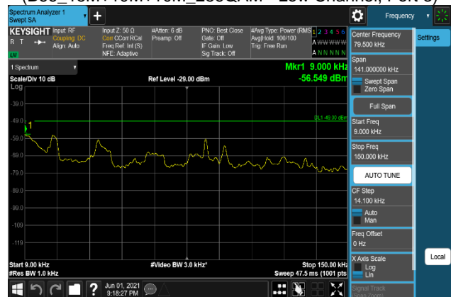
Plot 7-1014. Conducted Spurious Emission Plot 9 kHz to 150 kHz (B66_15M+10M+10M_16QAM - Middle Channel, Port 0)
