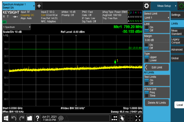
Plot 7-967. Conducted Spurious Emission Plot 30 MHz to 1 GHz (B66_15M+10M+10M_64QAM - Low Channel, Port 2)
