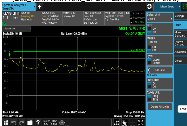
Plot 7-987. Conducted Spurious Emission Plot 9 kHz to 150 kHz (B66_15M+10M+10M_64QAM - Low Channel, Port 3)
