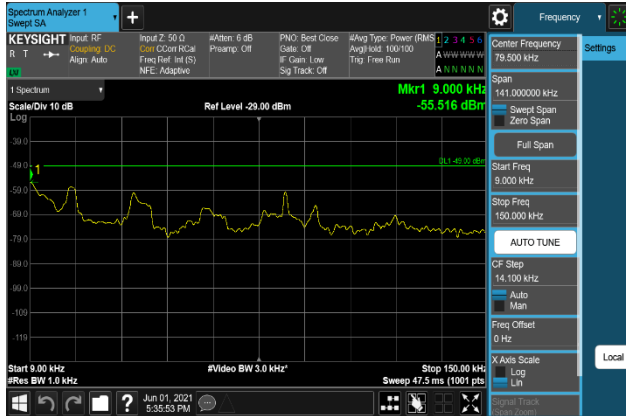
Plot 7-985. Conducted Spurious Emission Plot 9 kHz to 150 kHz (B66_15M+10M+10M_QPSK - Low Channel, Port 3)
