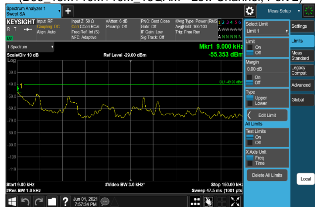
Plot 7-960. Conducted Spurious Emission Plot 9 kHz to 150 kHz (B66_15M+10M+10M_256QAM - Low Channel, Port 2)
