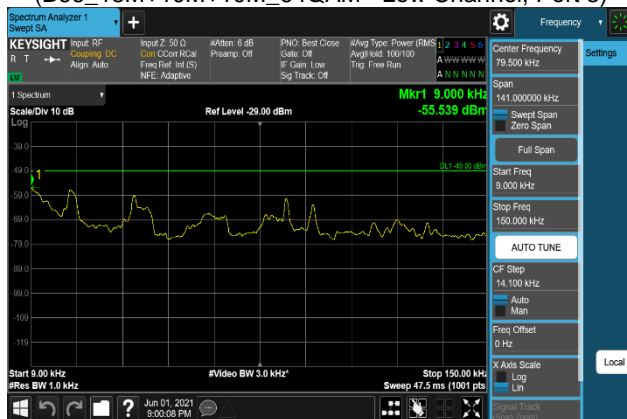
Plot 7-1013. Conducted Spurious Emission Plot 9 kHz to 150 kHz (B66_15M+10M+10M_QPSK - Middle Channel, Port 0)
