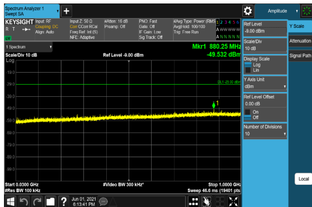
Plot 7-938. Conducted Spurious Emission Plot 30 MHz to 1 GHz (B66_15M+10M+10M_16QAM - Low Channel, Port 1)
