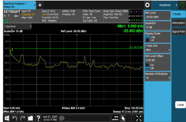
Plot 7-986. Conducted Spurious Emission Plot 9 kHz to 150 kHz (B66_15M+10M+10M_16QAM - Low Channel, Port 3)
