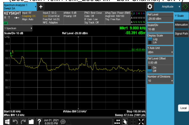
Plot 7-958. Conducted Spurious Emission Plot 9 kHz to 150 kHz (B66_15M+10M+10M_256QAM - Low Channel, Port 2)
