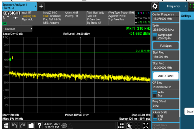
Plot 7-989. Conducted Spurious Emission Plot 150 kHz to 30 MHz (B66_15M+10M+10M_QPSK - Low Channel, Port 3)
