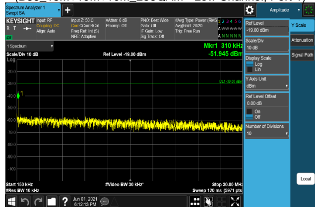
Plot 7-934. Conducted Spurious Emission Plot 150 kHz to 30 MHz (B66_15M+10M+10M_16QAM - Low Channel, Port 1)
