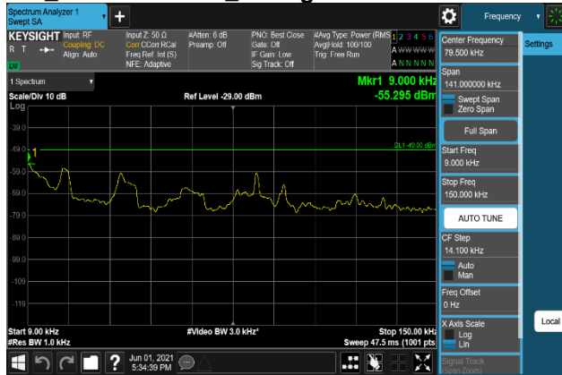
Plot 7-901. Conducted Spurious Emission Plot 9 kHz to 150 kHz (B66_15M+10M+10M_QPSK - Low Channel, Port 0)
