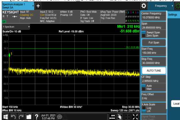
Plot 7-933. Conducted Spurious Emission Plot 150 kHz to 30 MHz (B66_15M+10M+10M_QPSK - Low Channel, Port 1)
