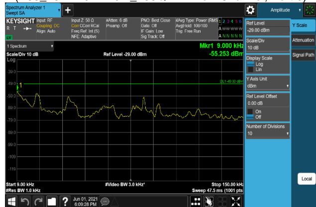
Plot 7-930. Conducted Spurious Emission Plot 9 kHz to 150 kHz (B66_15M+10M+10M_16QAM - Low Channel, Port 1)
