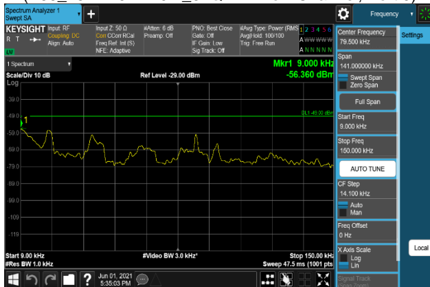
Plot 7-929. Conducted Spurious Emission Plot 9 kHz to 150 kHz (B66_15M+10M+10M_QPSK - Low Channel, Port 1)
