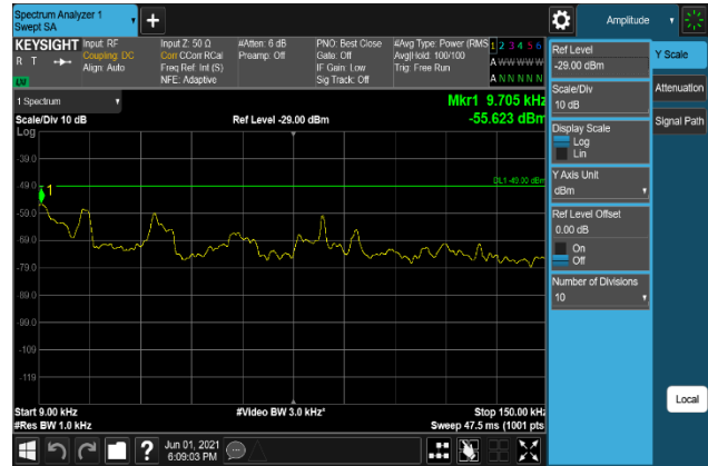
Plot 7-902. Conducted Spurious Emission Plot 9 kHz to 150 kHz (B66_15M+10M+10M_16QAM - Low Channel, Port 0)
