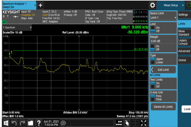
Plot 7-931. Conducted Spurious Emission Plot 9 kHz to 150 kHz (B66_15M+10M+10M_64QAM - Low Channel, Port 1)
