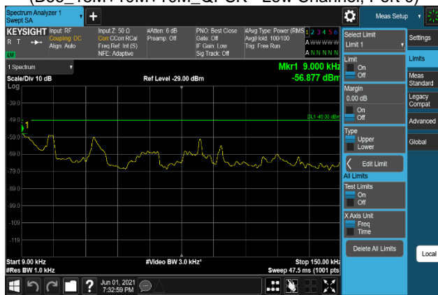
Plot 7-903. Conducted Spurious Emission Plot 9 kHz to 150 kHz (B66_15M+10M+10M_64QAM - Low Channel, Port 0)
