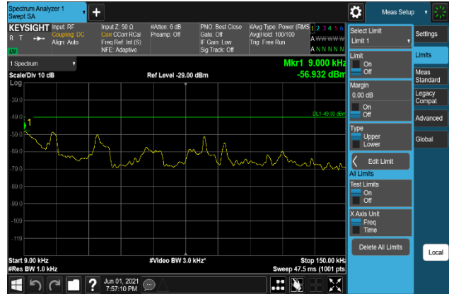
Plot 7-932. Conducted Spurious Emission Plot 9 kHz to 150 kHz (B66_15M+10M+10M_256QAM - Low Channel, Port 1)
