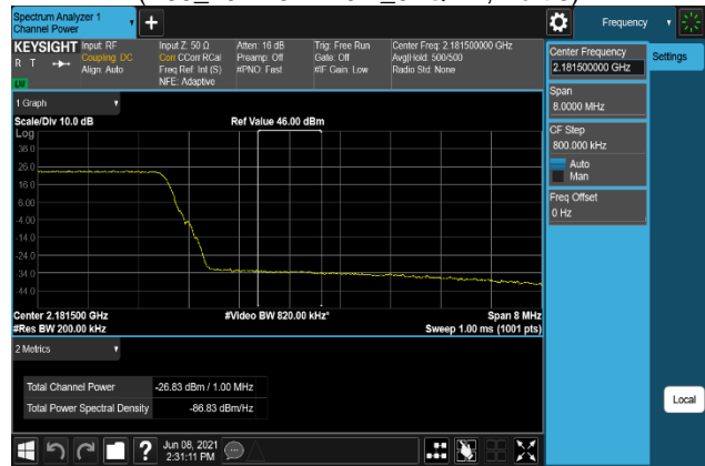
Plot 7-772. Band Edge Emission(Channel Power) Plot (B66_20M+5M+10M_256QAM, Port 3)
