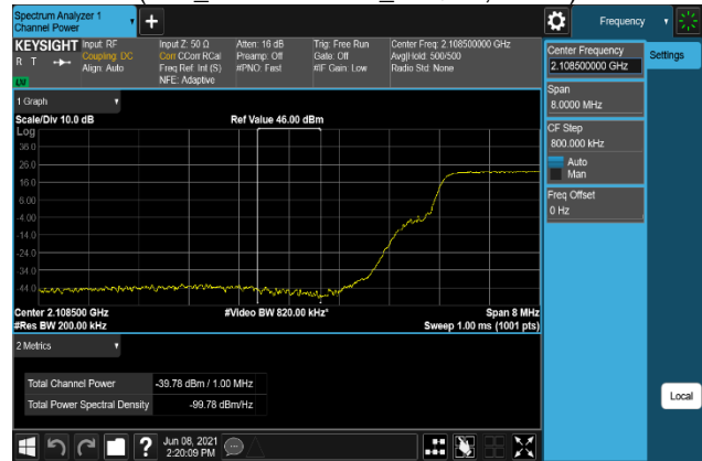
Plot 7-714. Band Edge Emission(Channel Power) Plot (B66_20M+5M+10M_64QAM, Port 0)
