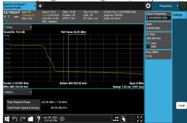
Plot 7-748. Band Edge Emission(Channel Power) Plot (B66_20M+5M+10M_256QAM, Port 0)
