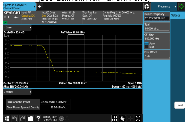
Plot 7-744. Band Edge Emission(Channel Power) Plot (B66_20M+5M+10M_16QAM, Port 0)
