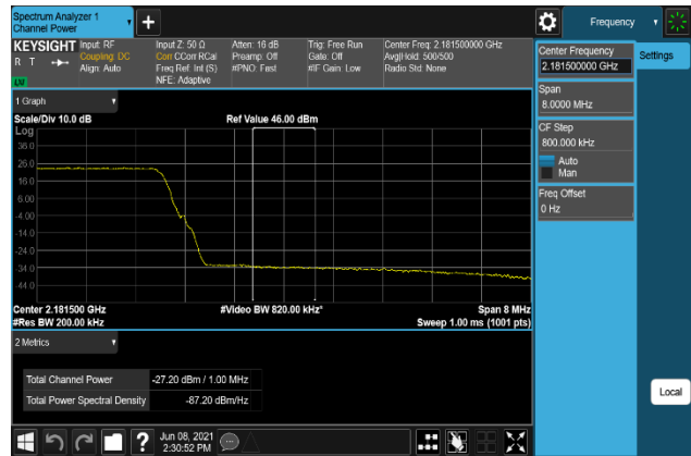
Plot 7-764. Band Edge Emission(Channel Power) Plot (B66_20M+5M+10M_256QAM, Port 2)
