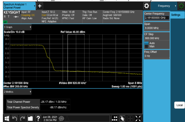
Plot 7-756. Band Edge Emission(Channel Power) Plot (B66_20M+5M+10M_256QAM, Port 1)
