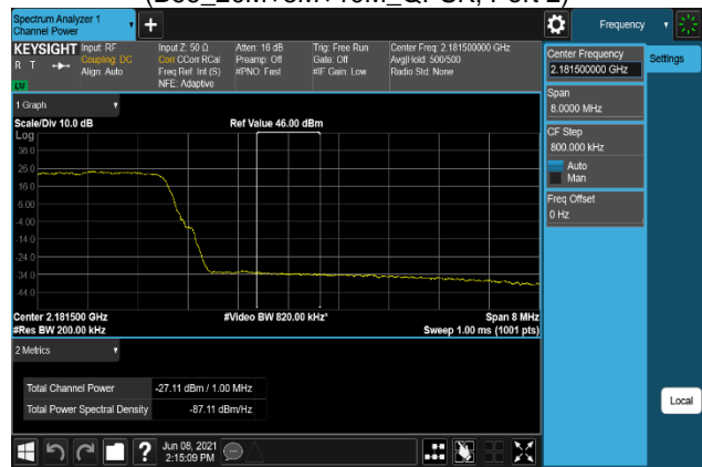
Plot 7-760. Band Edge Emission(Channel Power) Plot (B66_20M+5M+10M_16QAM, Port 2)
