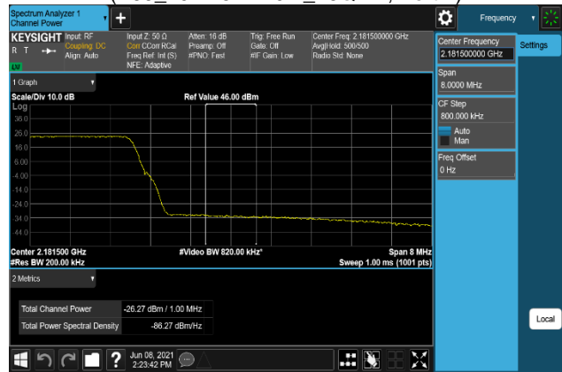
Plot 7-754. Band Edge Emission(Channel Power) Plot (B66_20M+5M+10M_64QAM, Port 1)
