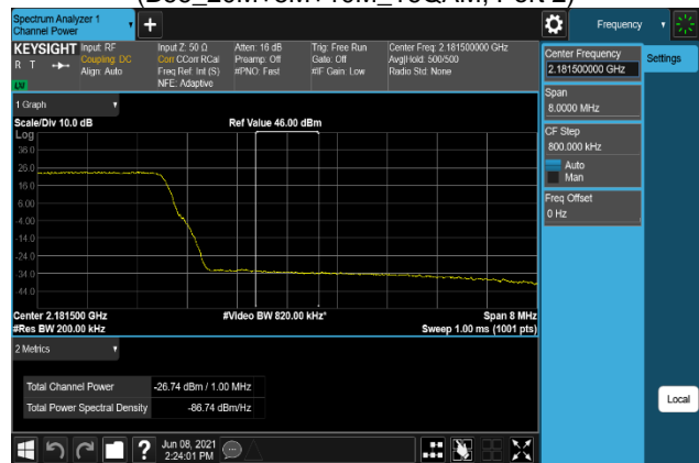
Plot 7-762. Band Edge Emission(Channel Power) Plot (B66_20M+5M+10M_64QAM, Port 2)
