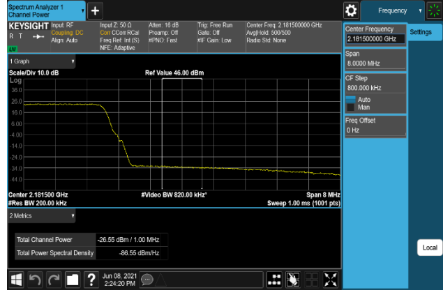
Plot 7-770. Band Edge Emission(Channel Power) Plot (B66_20M+5M+10M_64QAM, Port 3)
