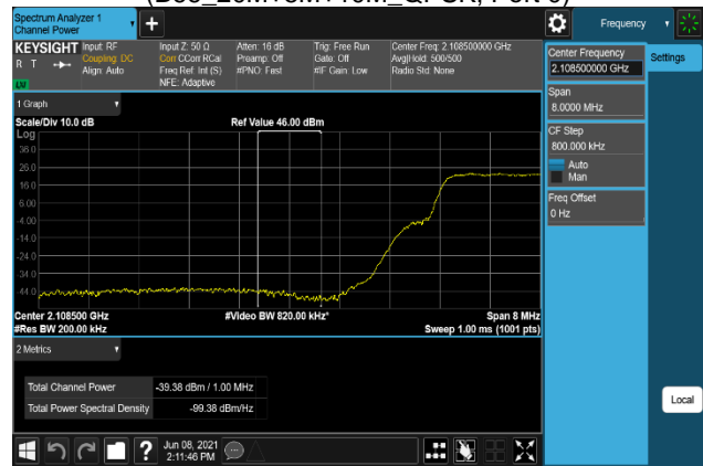
Plot 7-712. Band Edge Emission(Channel Power) Plot (B66_20M+5M+10M_16QAM, Port 0)
