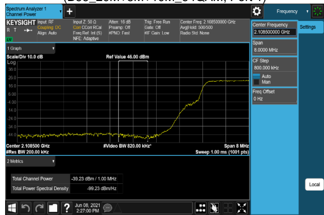
Plot 7-724. Band Edge Emission(Channel Power) Plot (B66_20M+5M+10M_256QAM, Port 1)
