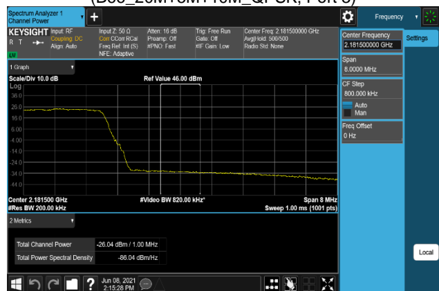
Plot 7-768. Band Edge Emission(Channel Power) Plot (B66_20M+5M+10M_16QAM, Port 3)
