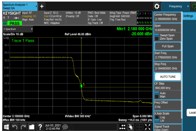
Plot 7-629. Band Edge Emission Plot (B66_15M+10M+10M_QPSK, Port 2)
