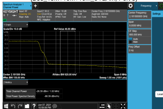
Plot 7-644. Band Edge Emission(Channel Power) Plot (B66_15M+10M+10M_256QAM, Port 3)
