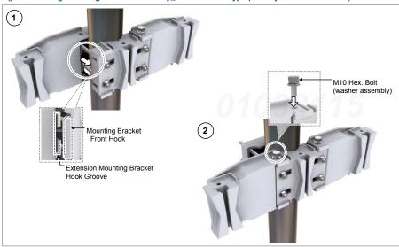
7 Check the level of mounting bracket assembly on a pole and adjust the level.
