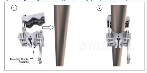
3 Locate the upper stud bolt in the upper side hole of the mounting bracket\_rear and fix the fastening materials temporarily on upper side.
