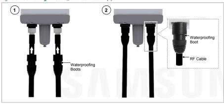
5 Insert the rubber for waterproofing boot to the system side RF ports. (ANT1, ANT2)
