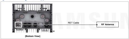
${f 3}$  Separate the cap from the system side connector (RET port).
