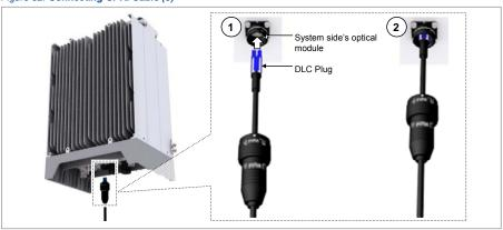
7 Insert the connector aligning the cable side connector's white dot and system side connector's white dot. When inserting the connector, push the shell to upper side.
