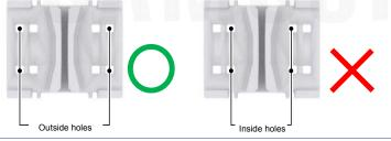
2 Insert stud bolts to the outside hole of mounting bracket\_front.
