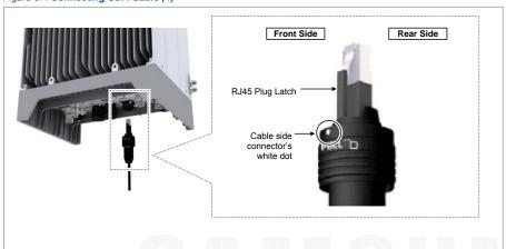
**6** Insert the RJ-45 plug to the system side connector.
