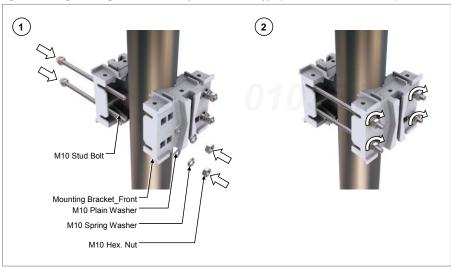
5 Check the level of mounting bracket assembly on a pole and adjust the level.
