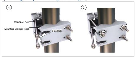
4 Locate the lower stud bolt in the lower side hole of the mounting bracket\_rear and fix the all fastening materials.
