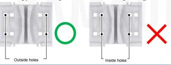
2 Insert stud bolts to the outside hole of mounting bracket\_front.
