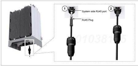
7 Insert the connector aligning the cable side connector's white dot and system side connector's white dot. When inserting the connector, push the shell to
