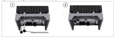
**6** Connect cables to the system side RF port. (ANT1, ANT2)
