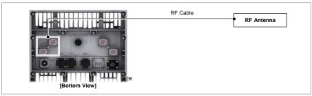
2 Insert the rubber for waterproofing boot to the RF antenna ports.
