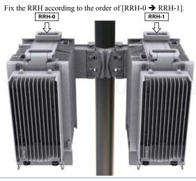
2 Hang the unit bracket hook of RRH-0 side on the mounting bracket\_front hook's groove and fix it using fasteners.
