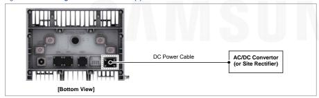
3 Insert the connector aligning the cable side connector's white dot and system side connector's white dot. When inserting the connector, push the shell to upper side.
