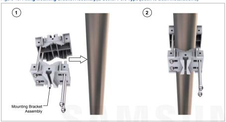
4 Pass a stud bolt through 2sector mounting bracket assembly\_front hole and fix mounting bracket assembly using fasteners.
