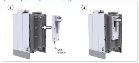
3 Fix a unit bracket using fasteners.
