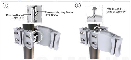
6 Fit the Extension mounting bracket's groove into the mounting bracket\_front's left hook, fix it using fasteners.
