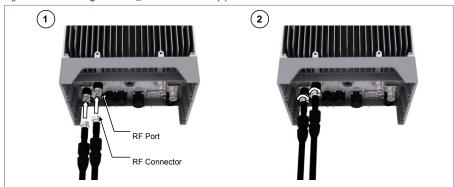
7 After connecting the connector, push waterproofing boots up to the connector
