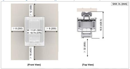
Figure 11. RRH Arrangement\_1 Sector Wall Type Installation (Side Installation)
