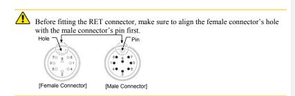
${\bf 2} \quad \text{Install an RET cable from the RF Antenna to the RRH RET port.}$
