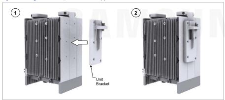
3 Fix a unit bracket using fasteners.
