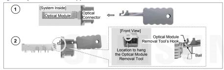
2 Completely remove the optical module from the optical module cage by pulling the Optical Module Removal Tool.
