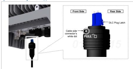
**6** Insert the DLC plug to the system side's optical module.
