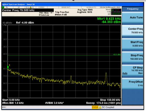
Antenna 1 / 150 kHz ~ 30 MHz / 5G NR n66 20 MHz 1 Carrier + 5G NR n66 10 MHz 1 Carrier [2 Carrier] / Contiguous / QPSK / High
