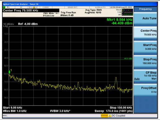
Antenna 0 / 150 kHz ~ 30 MHz / 5G NR n66 20 MHz 1 Carrier + 5G NR n66 10 MHz 1 Carrier [2 Carrier] / Non-Contiguous / QPSK
