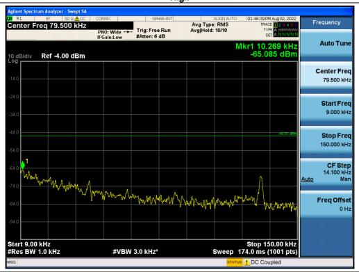
Antenna 1 / 150 kHz ~ 30 MHz / 5G NR n66 5 MHz 1 Carrier + LTE B66 5 MHz 1 Carrier [2 Carrier] / Contiguous / 256QAM / High
