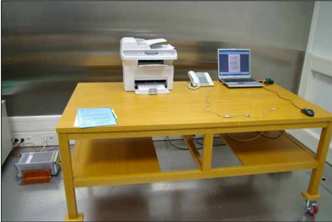
Picture 1. Conducted Emission (Front)
