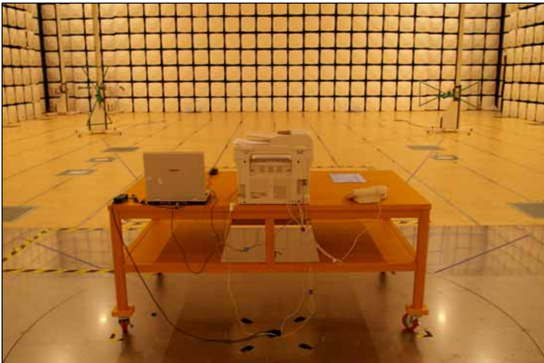
Picture 4. Radiated emission (Rear)
