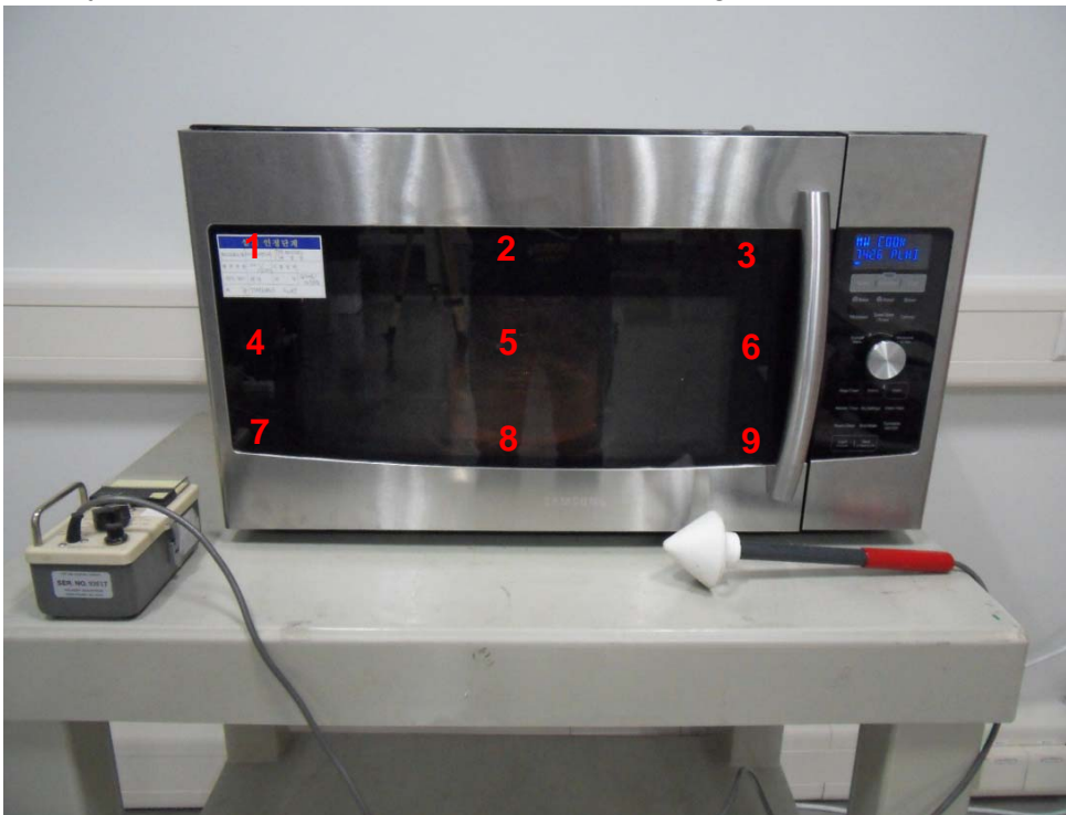
Fig. 1 Test Setup for Radiation Hazard Measurement
