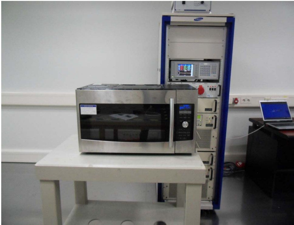
Fig. 2 Test Setup for Input power
