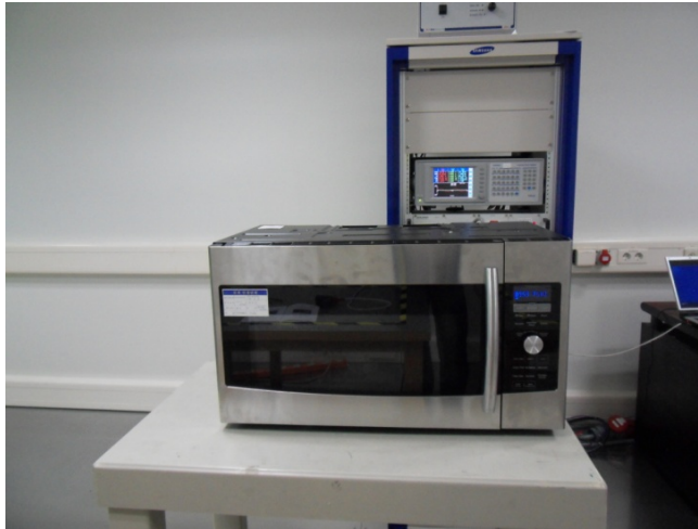
Fig.3 Test Setup for RF output power
