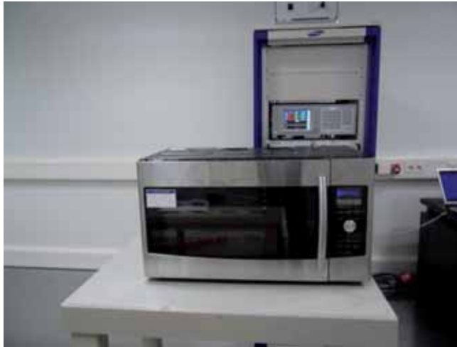
Fig.3 Test Setup for RF output power
