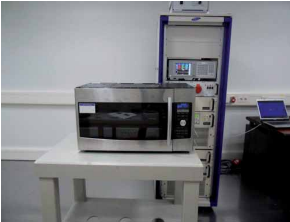
Fig. 2 Test Setup for Input power
