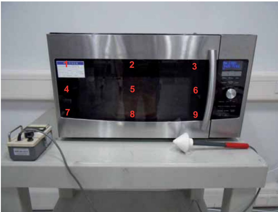
Fig. 1 Test Setup for Radiation Hazard Measurement
