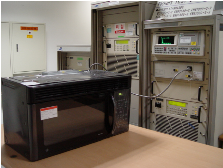
Fig. 2 Test Setup for Input power
