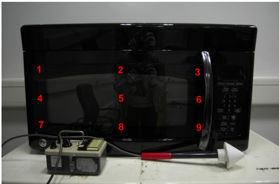
Fig. 1 Test Setup for Radiation Hazard Measurement
