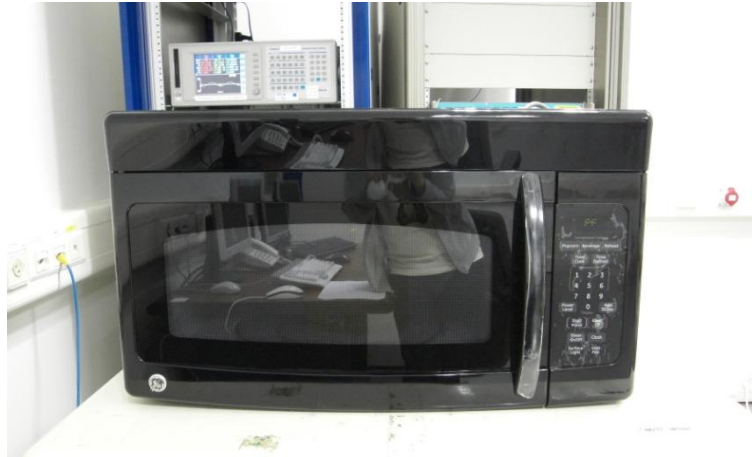
Fig.3 Test Setup for RF output power
