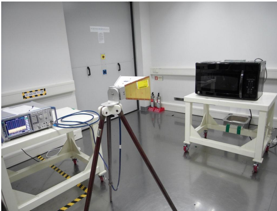
Fig. 4 Operating Frequency Measurements Configuration
