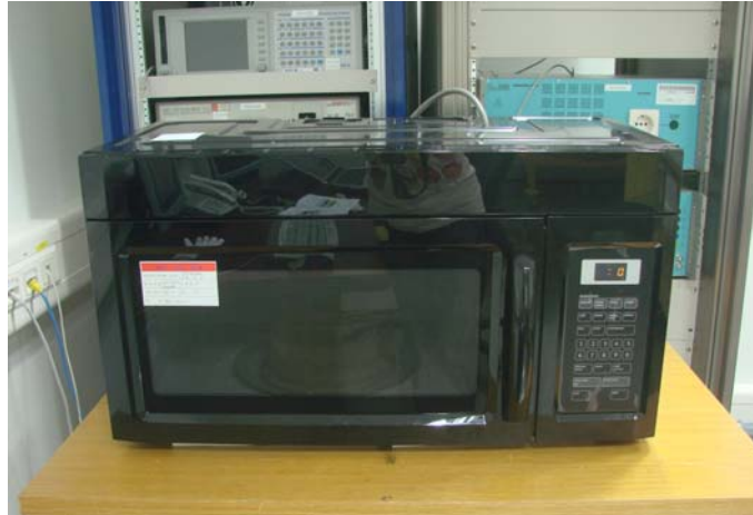
Fig.3 Test Setup for RF output power
