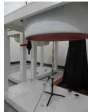
Photo of the dipole Antenna
