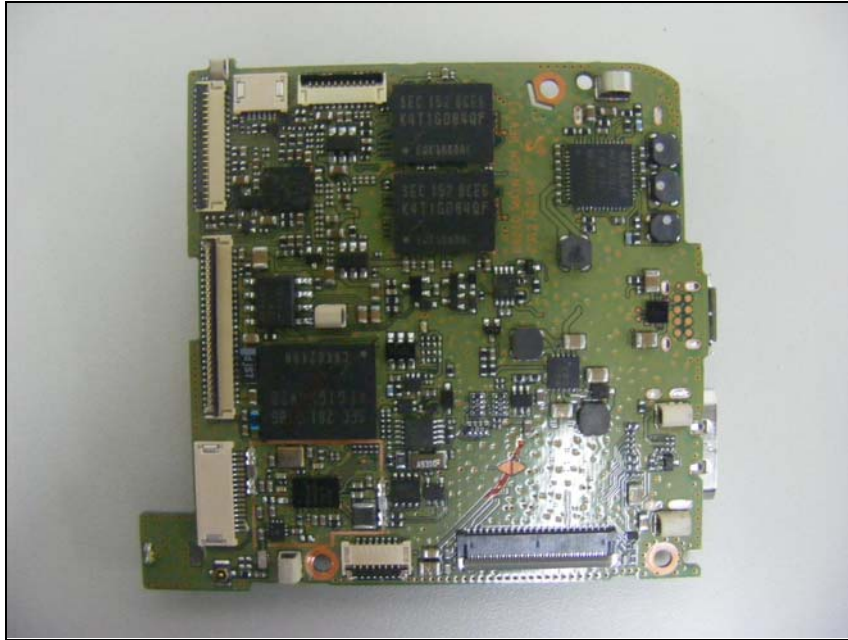
Top view of Main PCB
