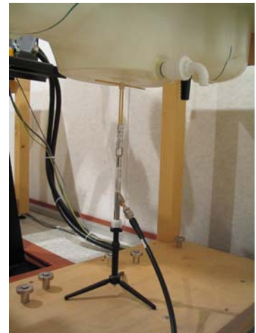
Photo of the dipole Antenna
